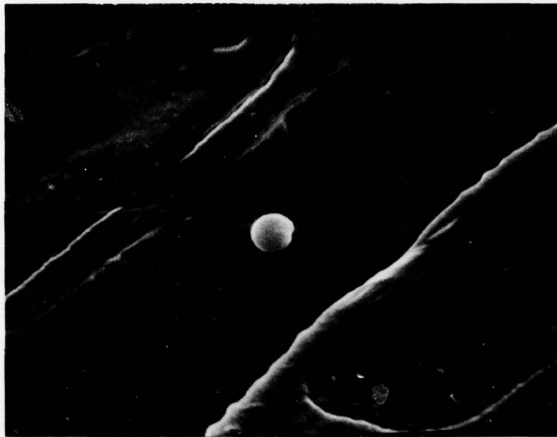
Figure 37. SEM picture of diode junction short on N5710T.
