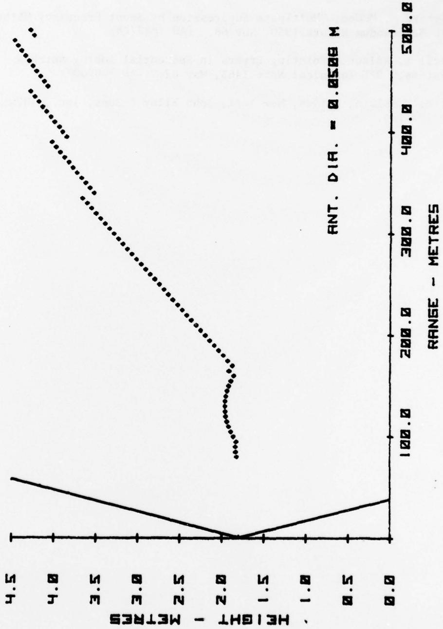
Figure 29. Theoretical Path of "Perfect" Beamrider, Antenna Diameter = 50.8 mm.
