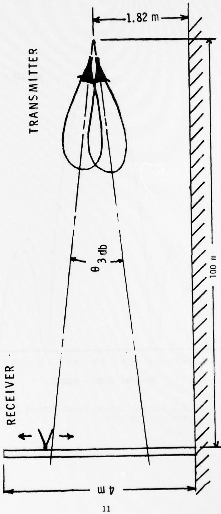
Figure 1. Experimental Setup
