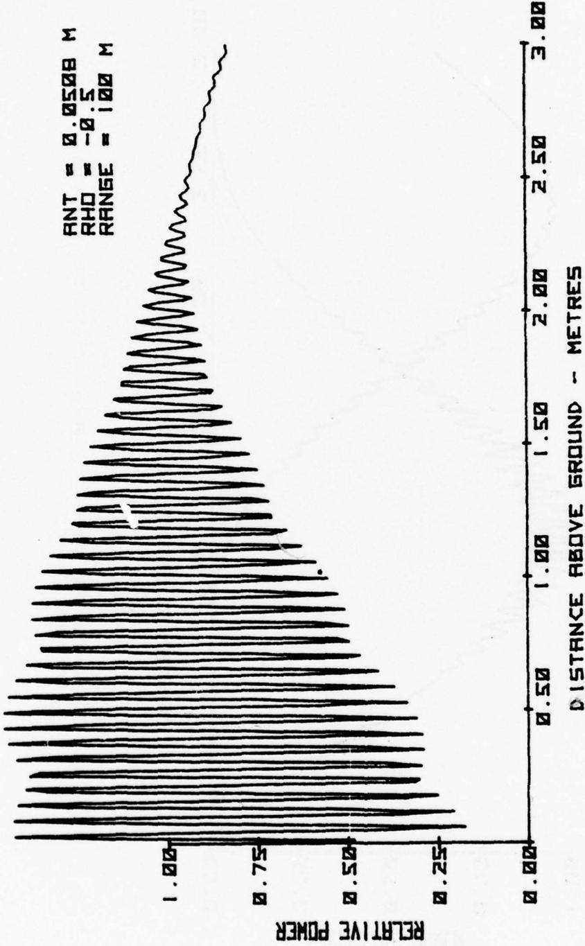
Figure 20. Theoretical Tracking Pattern, 50.8-mm Antenna,  $\rho = -0.5$
