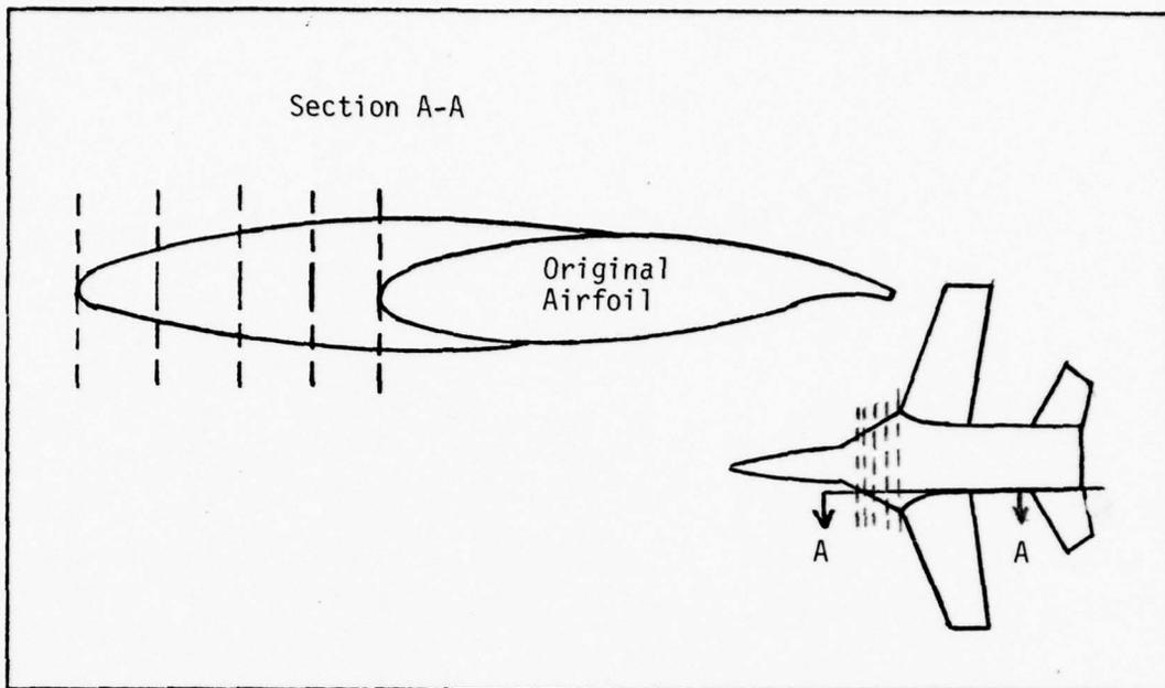
Figure 10. Root Chord Modification for F-111A Aircraft
