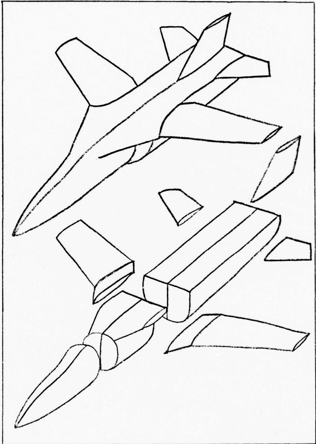
Figure 9. Component Identification for the F-111A Aircraft
