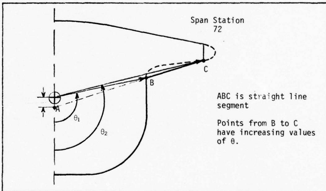
Figure 11. Glove Modification for Fuselage Cross Sections
