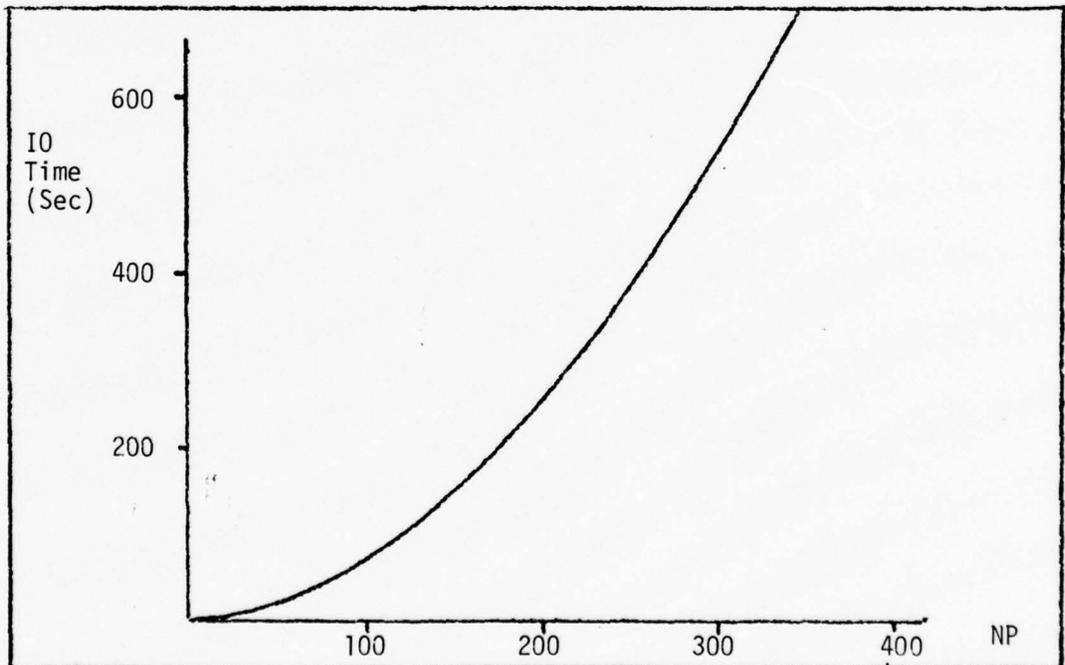
Figure 8. Input/Output Time Required vs. Number of Panels
