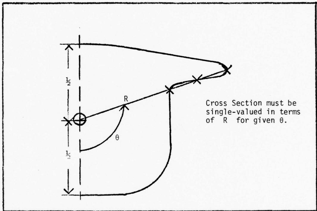
Figure 6. Example of Improper Data for USSAERO Program
