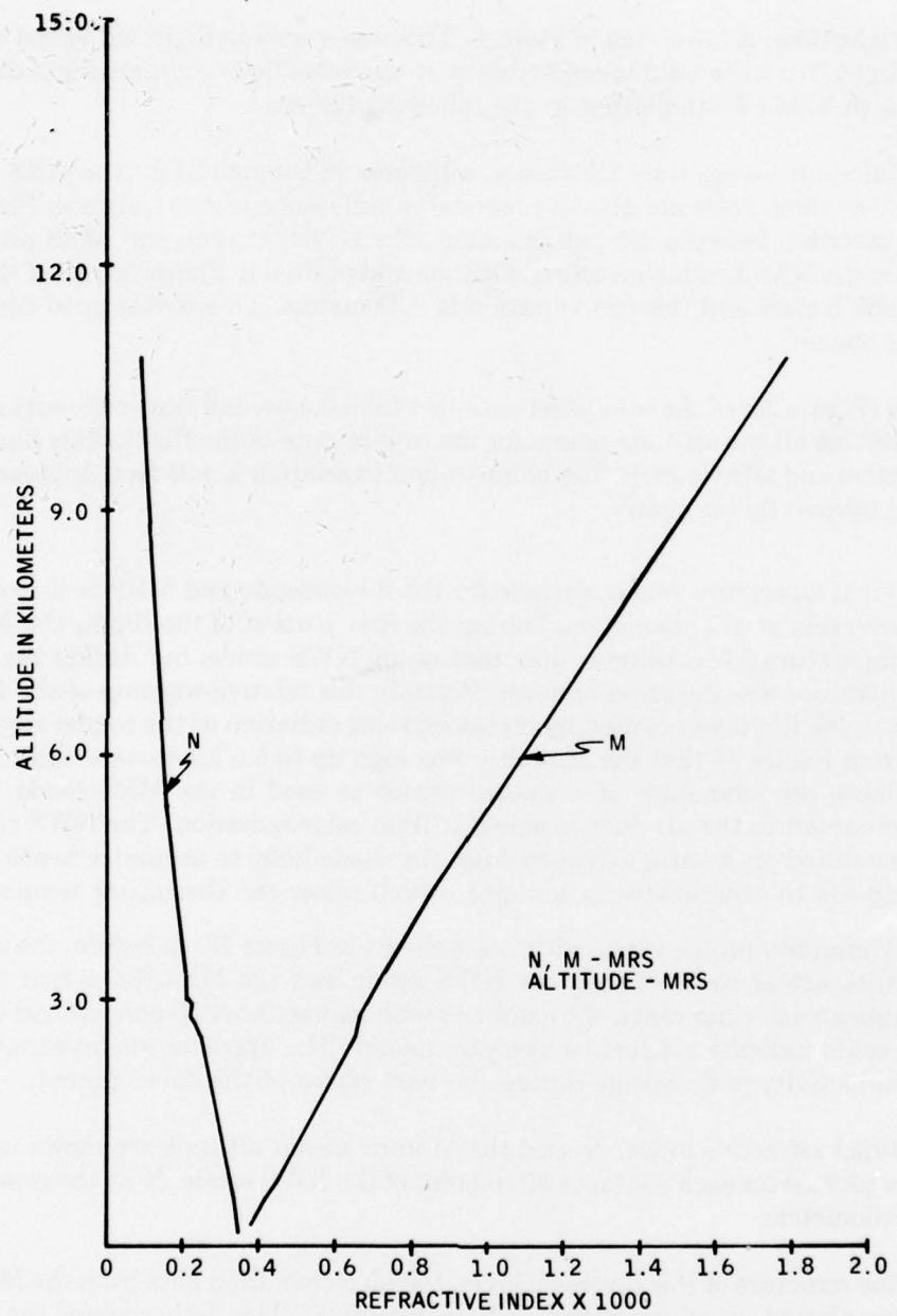
Figure 21. Plot of Modified Refractive Index, N, and M-Units versus Altitude Read by Mini-Refraction Sonde — Flight Number 2
