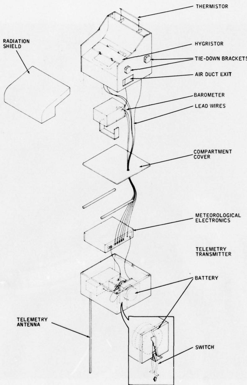
Figure 2. Exploded View of Minisonde Showing Subassemblies
