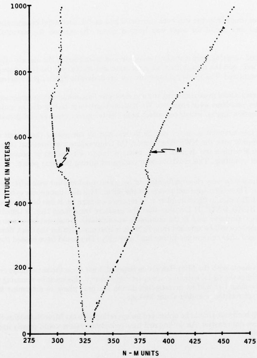
**Figure 32.** Plot of N and M versus Altitude for the First 1000 Meters of Flight Number 1 — Data Plotted for most of the Outputs of the Mini-Refraction Sonde at 2-1/2 Samples Per Second
