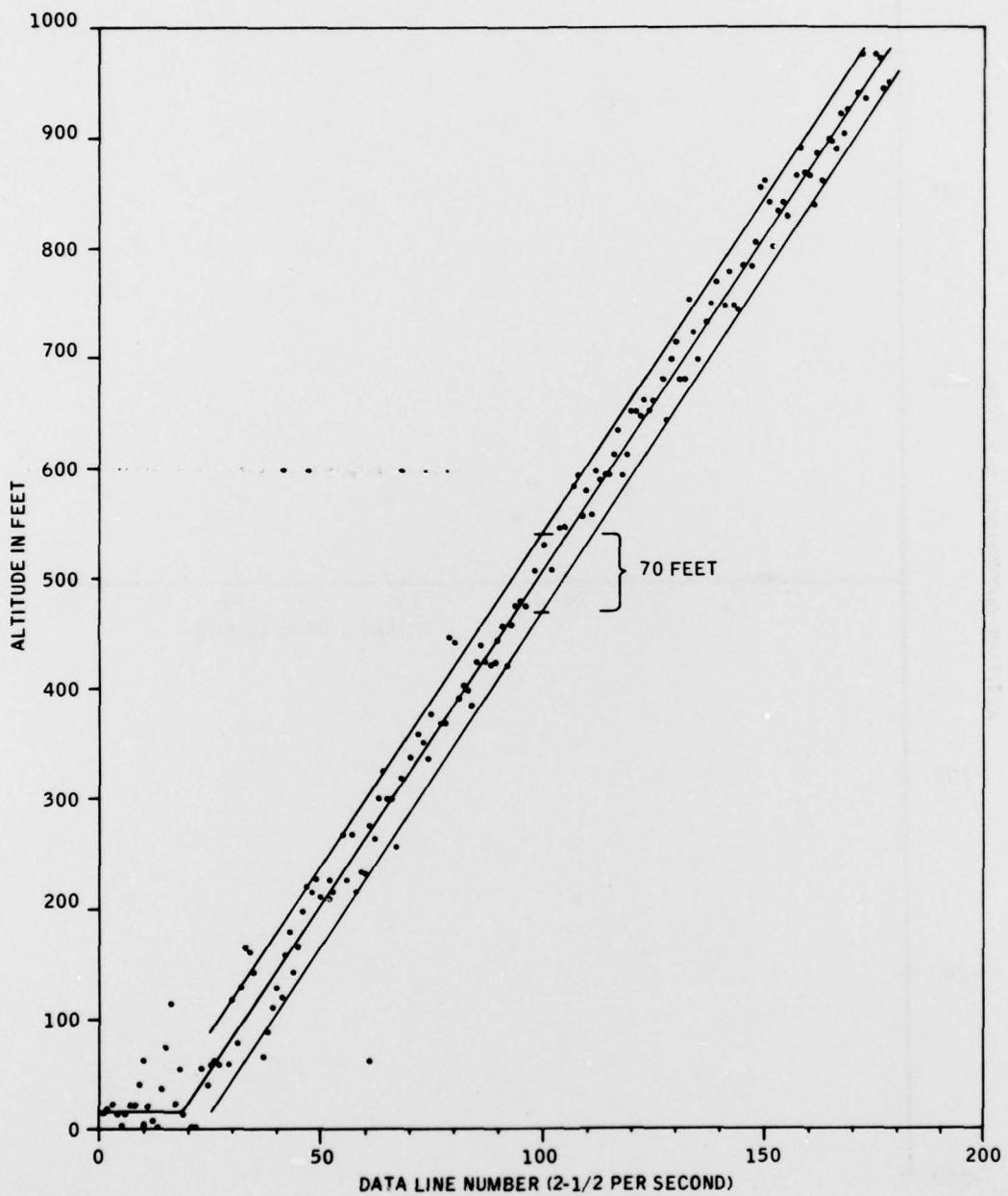
**Figure 26. Plot of Altitude versus Time for Flight Number 3 Measured with MRS.
