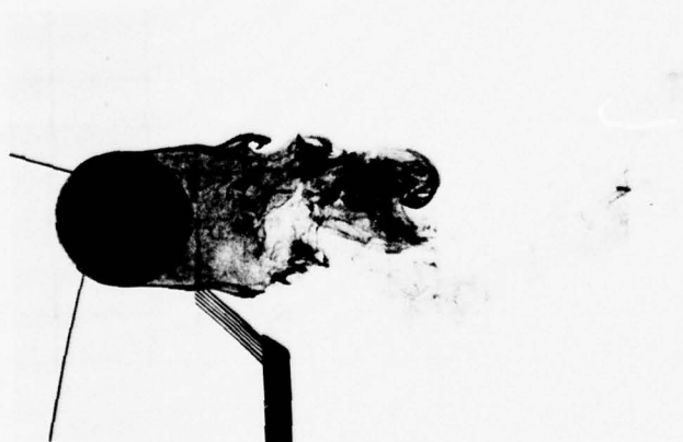
Figure 20. Dye Flow Visualization of Interaction of Six-Sensor Probe with Cylinder Wake
