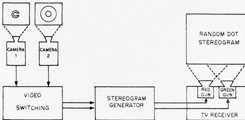
Fig. 1. Block diagram of stereogram generation system.
