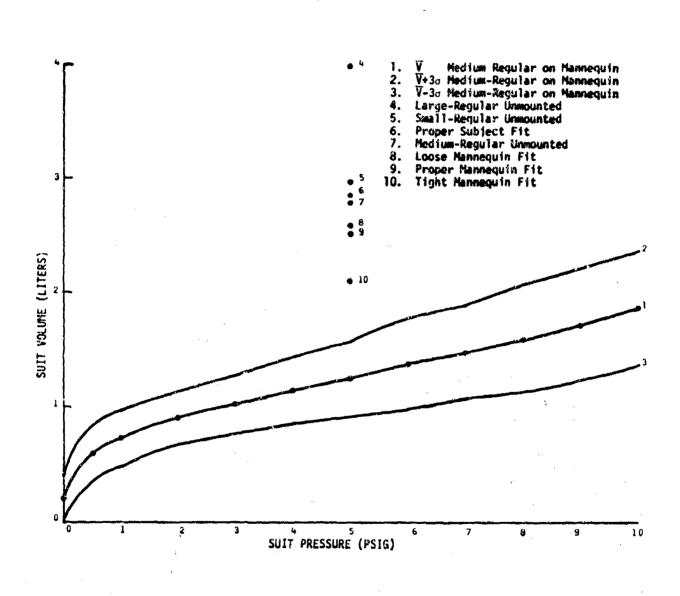
Figure 15. Abdominal bladder volume of the Pneumatic Lever Anti-G Suit.
