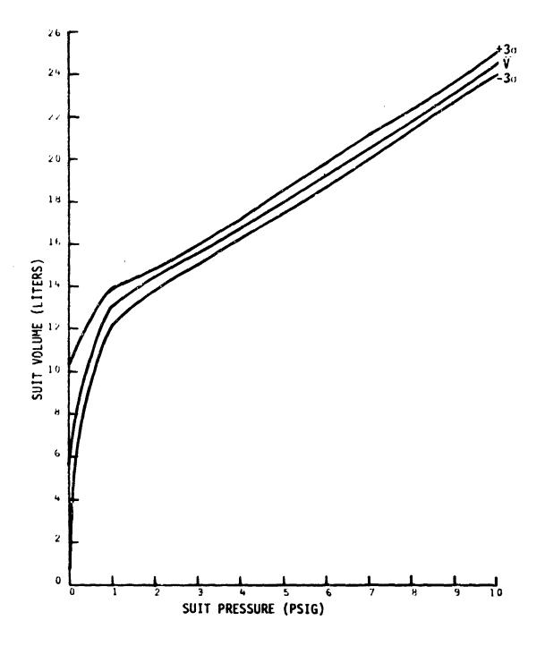
Figure 20. The effect of pressure on the volume (suit stretch) of the <u>CSU-12/P</u> anti-G suit (medium-regular size).
