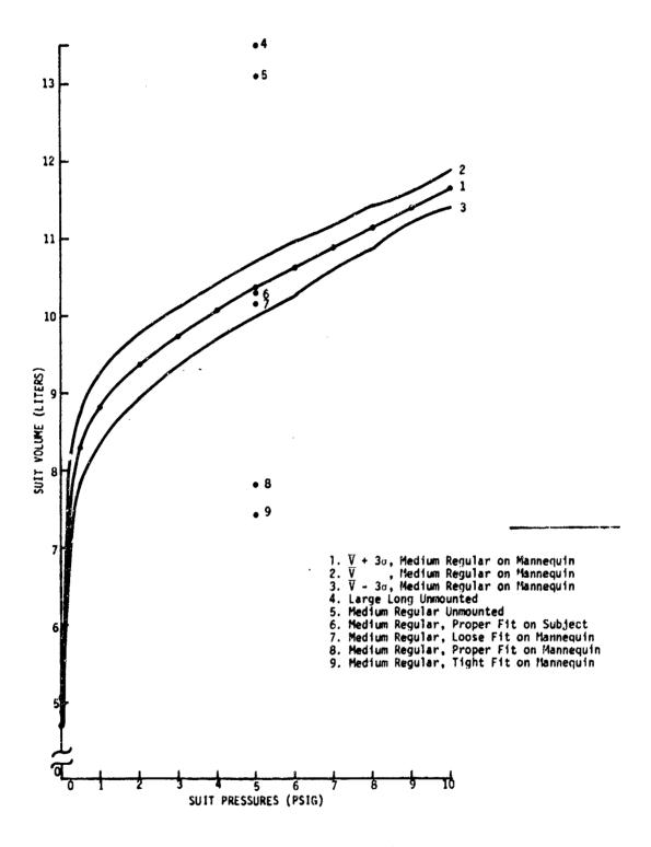
Figure 3. Volume of the <u>CSU-12/P</u> anti-G suit.
