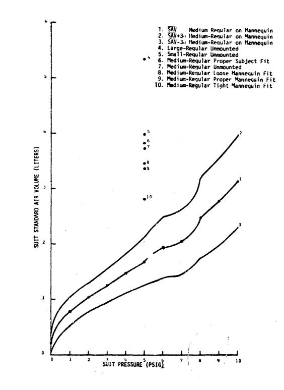
Figure 16. Standard air volume of the abdominal bladder in the Pogunatic Lever Anti-G Suit.
