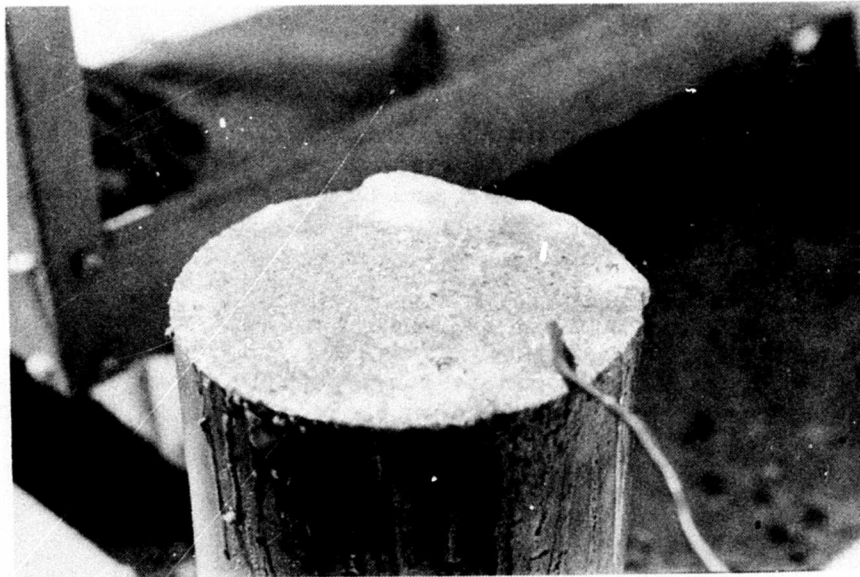
Figure 66. Close-up View of Blistered Speciment
