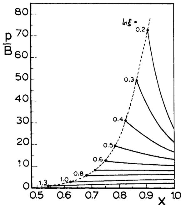
Fig. 6. Pressure profiles. The dashed line indicates the location of the interface.
