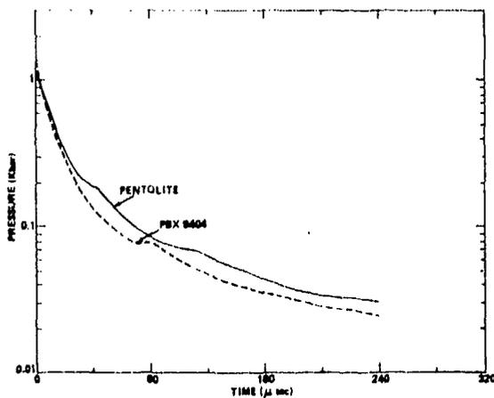
Fig. 7. Calculated pressure vs time at 10 charge radii, for centrally detonated PBX 9404 and pentolite, in water.
