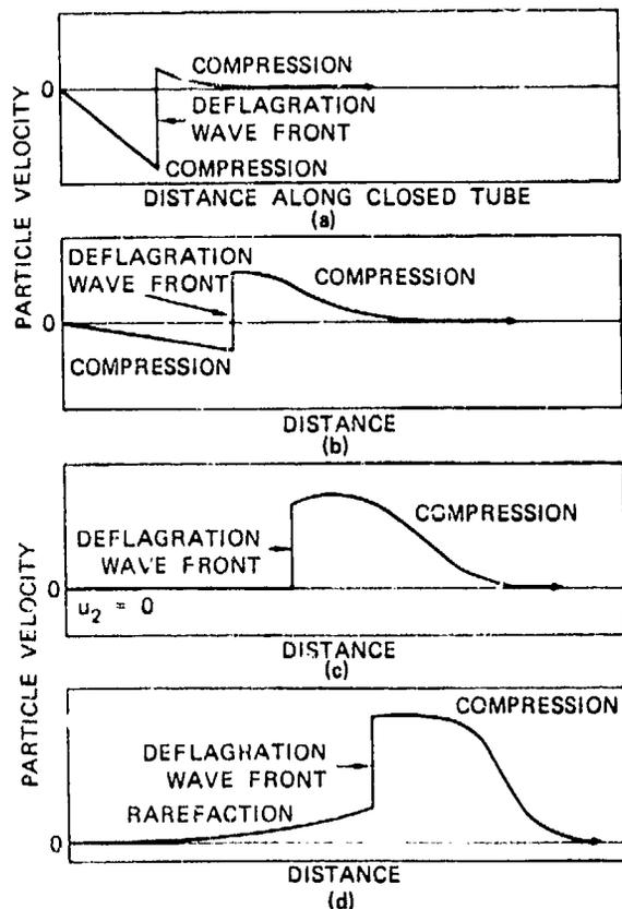
Fig. 6. Particle Velocity-Distance Diagrams for Accelerating Deflagration Waves
