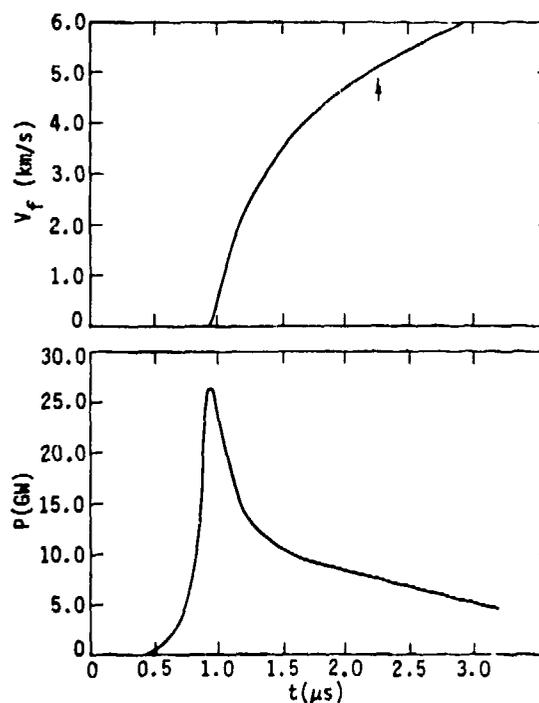
Fig. 2. (a) The upper curve is a laser-interferometer measurement of flyer velocity as a function of time for a 2.54-cm diameter, 0.025-cm thick flyer driven by a  $2.54 \times 2.54\text{-cm} \times 51\text{-}\mu\text{m}$  foil with 40 kV charging voltage on the capacitor bank. The arrow indicates the time at which the flyer reached the end of the barrel.
