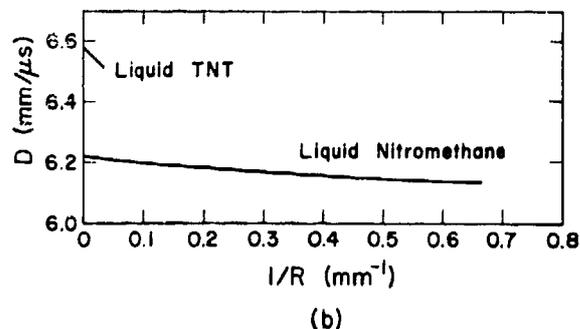
Fig. 5b. Diameter-effect curves for liquid TNT ( $\rho = 1.443 \text{ g/cm}^3$ ) and liquid nitromethane ( $\rho = 1.128 \text{ g/cm}^3$ ). The liquid TNT data points all lie within 0.4 m/s of the fit. The liquid nitromethane points all lie within 2 m/s of the fit.
