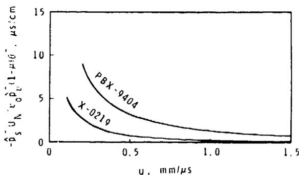
Fig. 2. Thermomechanical coefficient,  $-\hat{p}_s U_N / v_o \hat{p}_o (1-\mu)\theta^-$ , as a function of shock amplitude for unreactive PBX-9404 and X-0219. This coefficient couples the chemical energy release to the critical acceleration,  $\hat{\lambda}$ , per (4.2).
