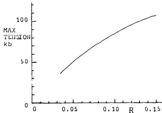
Fig. 6. Maximum tension vs. plate/charge thickness ratio R.
