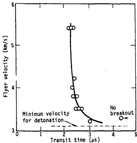
Fig. 6. Transit time of the detonation through 19-mm long pellets vs flyer velocity for 95% TATB (B-226)/5% KEL-F at a density of 1.80 Mg/m<sup>3</sup>.
