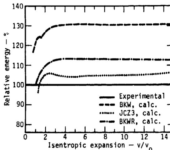
Fig. 6. TNT comparison of calculated and experimental isentrope energy.
