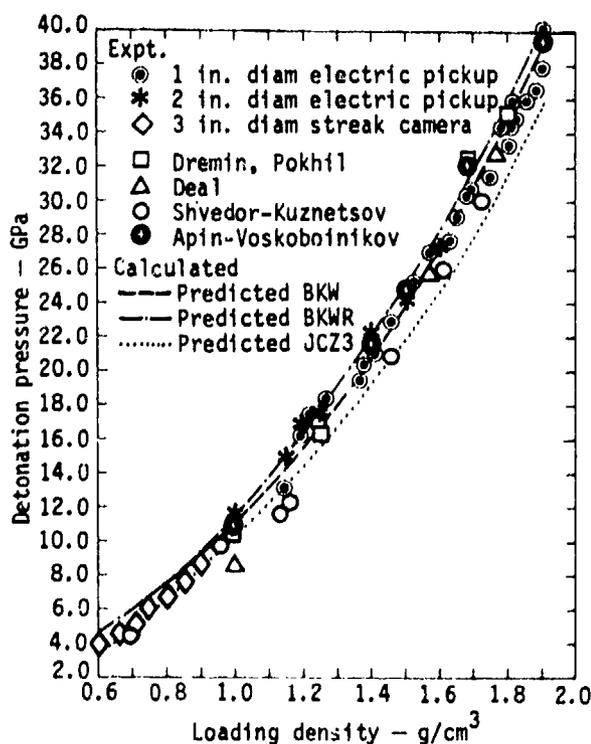
Fig. 1. HMX C-J pressure dependence on loading density.
