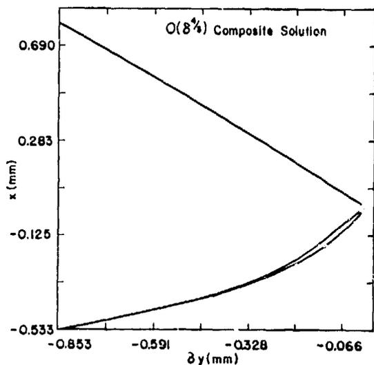
Fig. 3.10.  $O(\delta^{4/3})$  composite solution. The shock locus (upper curve), composite sonic locus (middle curve) and limiting characteristic (lower curve) in edge fixed coordinates. The parameter values are  $D = 8 \text{ mm}/\mu\text{s}$ ,  $\gamma = 3$ ,  $\kappa = 2 \mu\text{s}^{-1}$ , and  $\delta = 0.1$ .
