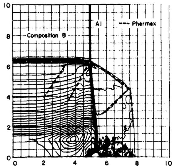
Fig. 6. The constant density profiles at 8 μsec for a 5-cm-half-thickness slab of Composition B detonating by the Forest Fire model up an aluminum plate 2.5-cm-thick. The prominent features of a radiograph of the flow are shown with dashed lines.
