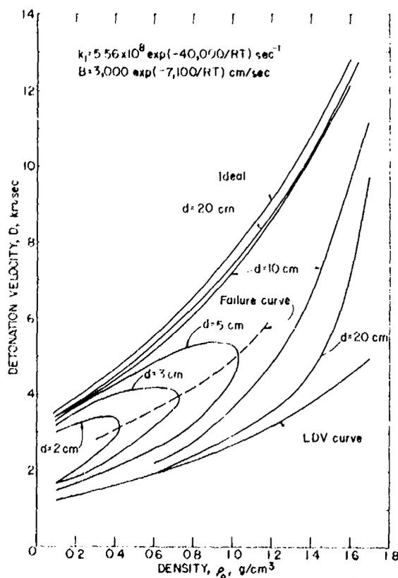
Fig. 3. Variation of Detonation Velocity With Loading Density "Modified Hypothetical" Explosive: Effect of Enhanced Grain Burning.
