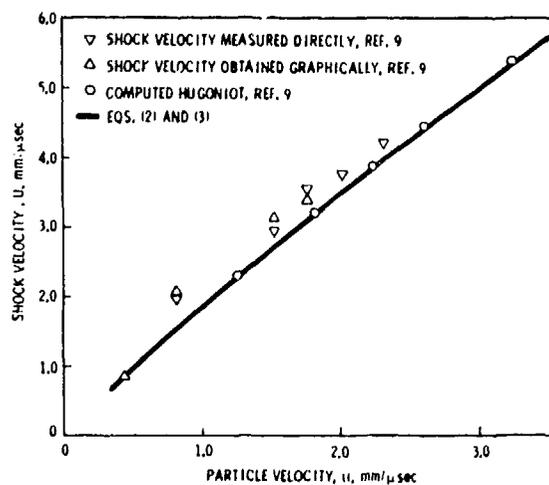
Fig. 10. Comparison of experimental and computed Hugoniot for AN at 0.86 g/cc.
