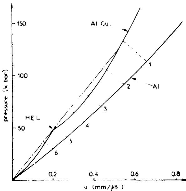
Hugoniot curve in  $(P, u)$  coordinates. The curvature is accentuated in order to make more apparent the limits of the instability region.
