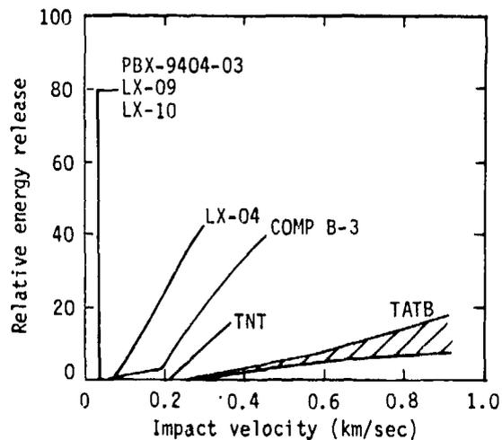
Fig. 2. Summary of Susan test data. All TATB formulations fell within the shaded region. These included neat TATB at densities of 1.70 and 1.84  $\text{Mg/m}^3$ ; and the following TATB/KEL-F formulations: 95/5 at  $\rho = 1.81 \text{ Mg/m}^3$ , 92.5/7.5 at  $\rho = 1.80$  and 1.90  $\text{Mg/m}^3$  and 90/10 at  $\rho = 1.92 \text{ Mg/m}^3$ . The LX-10 and LX-04 shown for reference are 94.5/5.5 and 85/15 HMX/Viton A respectively.
