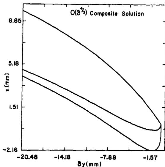
Fig. 3.9.  $O(\delta^{4/3})$  composite solution. The parameter values are  $D = 8 \text{ mm}/\mu\text{s}$ ,  $\gamma = 3$ ,  $\kappa = 2 \mu\text{s}^{-1}$ , and  $\delta = 0.33$ .
