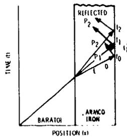
Fig. 5. X-t diagram of stress wave interactions. The elastic (E) wave interactions have been simplified.
