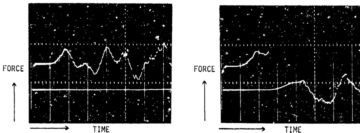
A. 3.0 mm confinement, 0.1 MPa initial pressure, fired at 573 V. Scales: upper = 8.1 MPa/div, lower = 810 MPa/div, time = 100  $\mu$ s/div.
