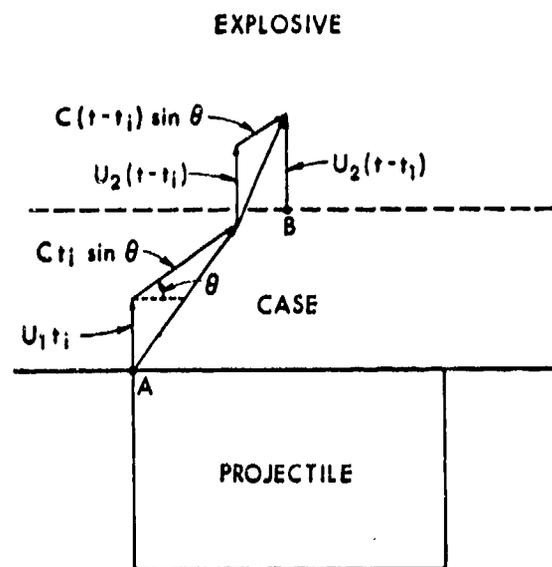
Fig. 1. Velocities to be considered in the propagation of a rarefaction from Point A to Point B are shown schematically.
