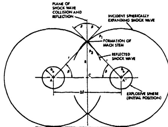
Fig. 4.1. The separated charge arrangement and a sketch of shock wave positions at the point of Mach wave formation where  $\beta = \beta_{crit}$  (after Ref. 15(a)).
