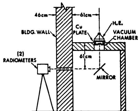
Fig. 1. Experimental arrangement for copper plate range firings.
