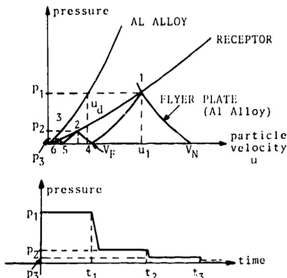
Fig. 1. Principle of generation of rectangular pressure pulses.
