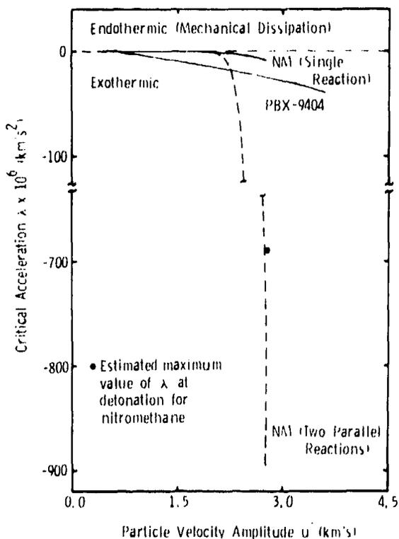
Fig. 2. Critical acceleration for steady wave propagation as a function of shock amplitude  $u^-$  for nitromethane and PBX-9404. The right end of each curve represents the detonation spike point. At the left end of the PBX-9404 curve,  $\lambda$  slightly exceeds zero.
