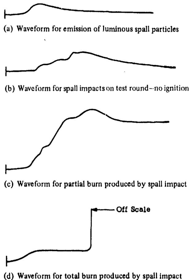
Fig. 7. Photocell waveforms from spall impact tests.
