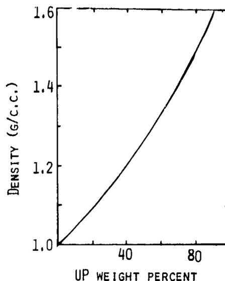
Fig. 3. Density (20°C) of aqueous solution of UP.
