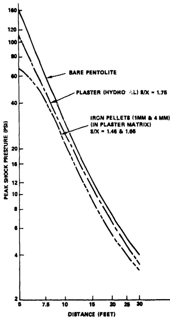
Fig. 5. Peak shock pressure vs distance for 8 lb. pentolite sphere encased in various materials.
