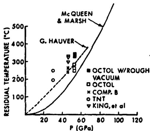
Fig. 5. Plot of experimental and theoretical data vs. the Hugoniot pressures. For the two octol points marked "Rough Vacuum", ambient pressure was near 100  $\mu\text{m}$ ; all other experimental points were obtained at less than 10  $\mu\text{m}$ .
