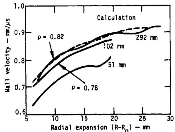
Fig. 4. Cylinder test wall velocity vs radial expansion ( $R - R_0$ ) scaled to a 25-mm cylinder. If the density ( $\rho$ ) of the 102-mm and 292-mm charges had been the same, their curves would have been virtually identical.
