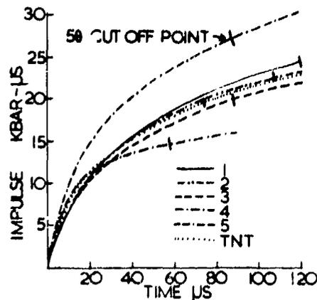
Fig. 9. Impulse flux versus time at 10 charge radii.
