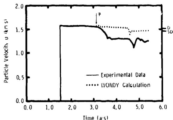
Fig. 5. Comparison of computed particle velocity history at the Cu/NM interface with Hardesty's experimental observation (9) in shot N4, where  $p^- = 7.5$  GPa and  $\theta^- = 934$  K. Velocity levels SD and D refer to boundary conditions behind superdetonation and detonation, respectively, independently calculated using TIGER (11).
