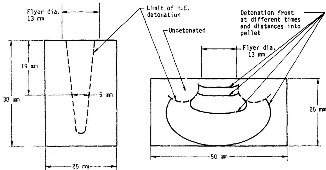
Fig. 9. Propagation of a detonation front in TATB (B-226) containing 5% binder. On the left a flyer having a velocity of 4.2 km/s detonates a hole into pressings of density 1.89 Mg/m<sup>3</sup>. No detonation breakout was observed from the 38-mm long pressings. On the right a flyer having a velocity of 5.0 km/s initiates a diverging detonation in pressings of 1.80 Mg/m<sup>3</sup>. Both figures represent compilations of a number of experiments using charges of varied sizes and shapes.
