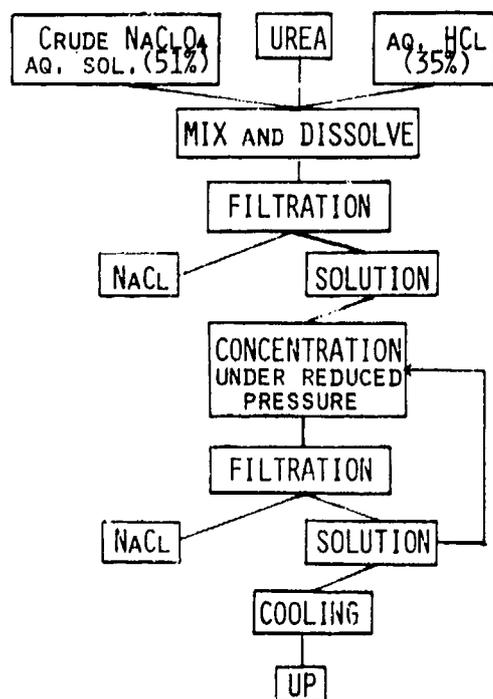
Fig. 1. Flow diagram of UP preparation.
