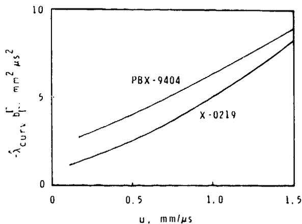
Fig. 1. Generalized critical acceleration due to curvature,  $-\hat{\lambda}_{curv}/b_F$ , as a function of shock amplitude,  $u$ , for unreactive PBX-9404 and X-0219. Note that the values are comparable for the two explosives.
