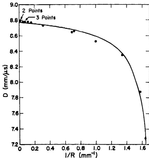
Fig. 4. Diameter-effect curve for PBX-9404;  $\rho = 1.846 \text{ g/cm}^3$ .
