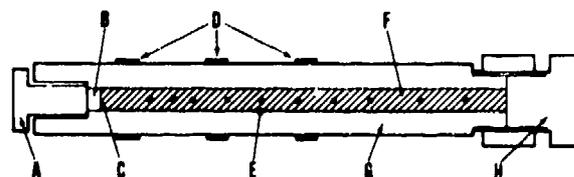
Fig. 1. Cross section of DDT tube. (A - ignitor bolt; B - ignitor; C - ignitor/explosive interface; D - strain gages; E - ionization probe location; F - explosive charge; G - tube; H - bottom closure. Inner diameter = 16.3 mm, outer diameter - 50.8 mm. Distance from ignitor/explosive interface to bottom closure = 295.4 mm.)
