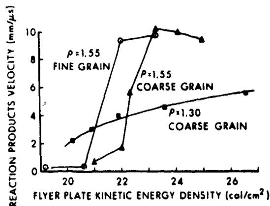
Fig. 6. Energy versus reaction response for 0.040 in. aluminum flyer.
