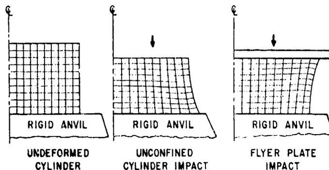
Fig. 1. Impact configurations.
