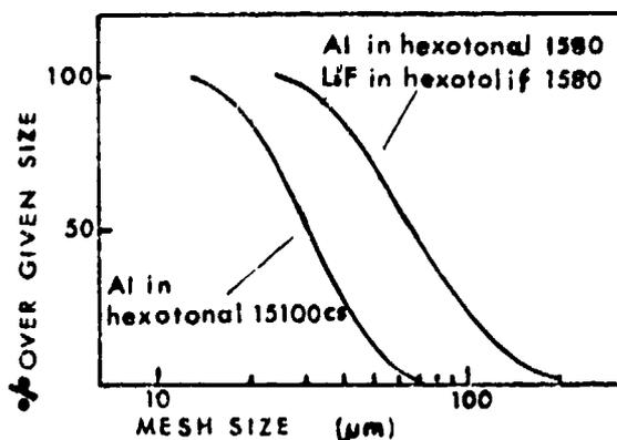
Fig. 3. Particle size distribution of Al and LiF.
