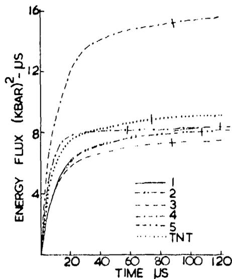
Fig. 10. Energy flux versus time at 10 charge radii.
