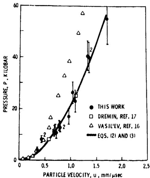
Fig. 3. Comparison of data for porous TNT.
