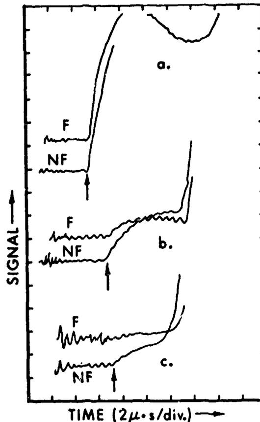
Fig. 3. Typical oscilloscope traces of the radiance signals from explosively loaded copper plates. (a) Cu/Octol; (b) Cu/comp B; (c) Cu/TNT. "F" is the 4-5.5  $\mu$ m trace at 50mV/div. sensitivity; "NF" is the 2-5.5  $\mu$ m trace at 100mV/div. The arrows indicate shock arrival.
