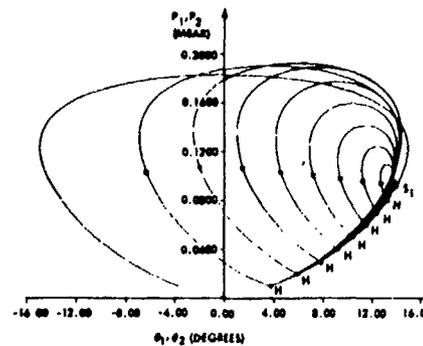
Fig. 3.10. Change in the reflected shock polars for water (S-W equation of state, Eq. 2.1) as the incident shock pressure  $p_1 = p_1'$  is increased from 10 kbar in kbar increments for fixed  $p_{1,max} = 183$  kbar. The sonic point for each polar is denoted by a \*.  $S_1$  is the sonic point for the incident shock polar.
