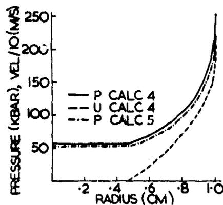
Fig. 4. Pressure and velocity distribution in detonation wave.
