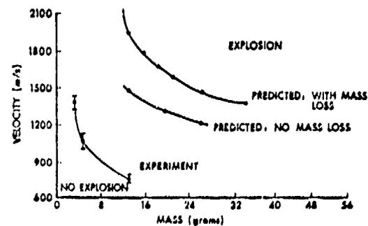
Fig. 3. The velocity for low order initiation of a PBX 9404 target is plotted as a function of projectile mass.
