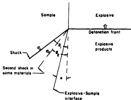
Fig. 1. Schematic of perpendicular drive. The heavy solid lines represent shocks and the small double arrows indicate their direction of propagation.
