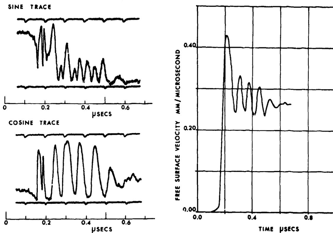
Fig. 5. Records and interpretation of foil impact on 5050B aluminium 1 mm thick. Foil velocity  $0.41 \text{ mm } \mu\text{sec}^{-1}$ . Fringe Constant  $0.20 \text{ mm } \mu\text{sec}^{-1} \text{ Fringe}^{-1}$ .
