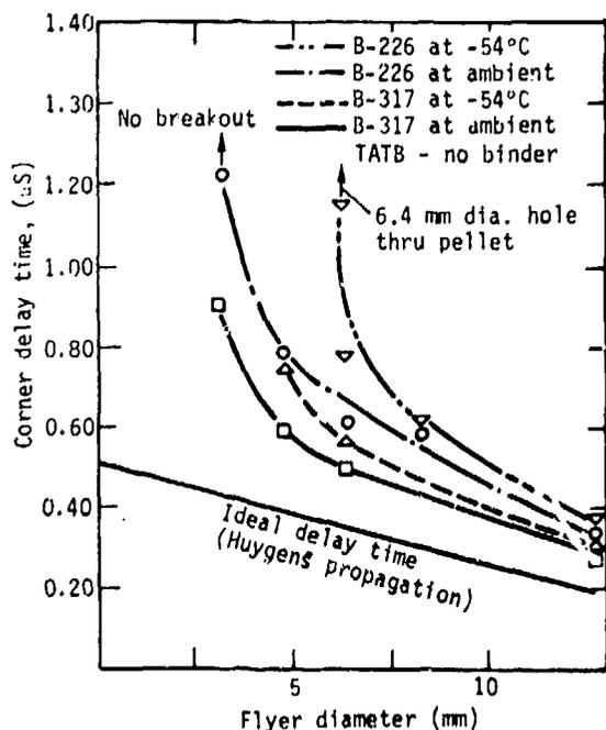
Fig. 12. Corner delay time (see Fig. 4) vs flyer diameter. The flyer velocity was  $\sim 6.5$  km/s. Blends of TATB having different particle size distributions (see Fig. 1) are compared at both ambient and low ( $-54^\circ\text{C}$ ) temperature.
