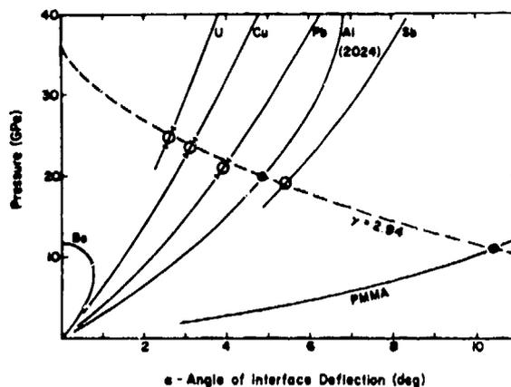
Fig. 4. Perpendicular drive by 9404. The solid lines are oblique shock solutions obtained from the reference Hugoniot. The dashed line is the Prandtl-Meyer expansion of detonation products described by a polytropic gas equation of state.
