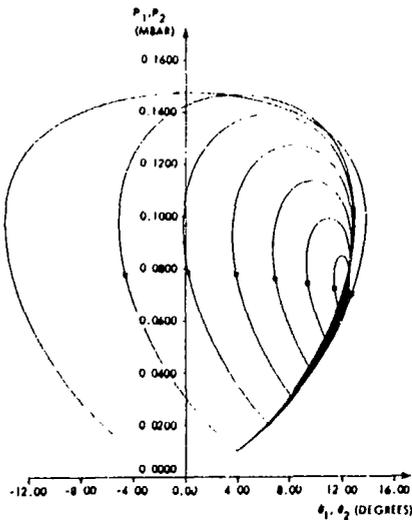
Fig. 3.11. Change in the reflected shock polars for water (S-W equation of state, Eq. 2.1) as the incident shock pressure  $p_1$  is increased from 10 kbar in 10 kbar increments for fixed  $p_{1,max} = 147.3$  kbar. The sonic point for each shock polar is denoted by an asterisk \*.
