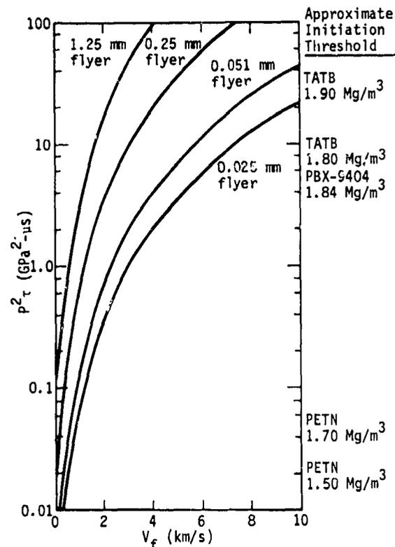
Fig. 9.  $P^2\tau$  vs flyer velocity for the impact of a PET flyer on a KEL-F target, where  $P$  is the peak pressure and  $\tau$  is the pulse duration.  $P^2\tau$  was calculated using energy conservation principles and the Hugoniot data from (8).
