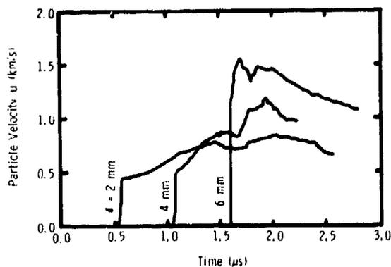
Fig. 3. Particle velocity histories observed in a window material behind a shock-loaded PBX-9404 sample of thickness  $\delta$ . The input pulse duration was  $1.1 \mu\text{s}$  (6).
