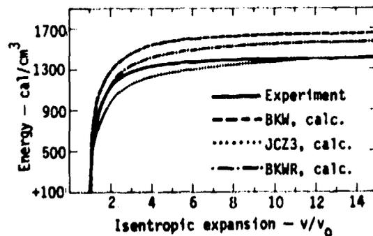
Fig. 9. RX-23-AA, Hydrazine Nitrate/Hydrazine 79/21, isentropic expansion.
