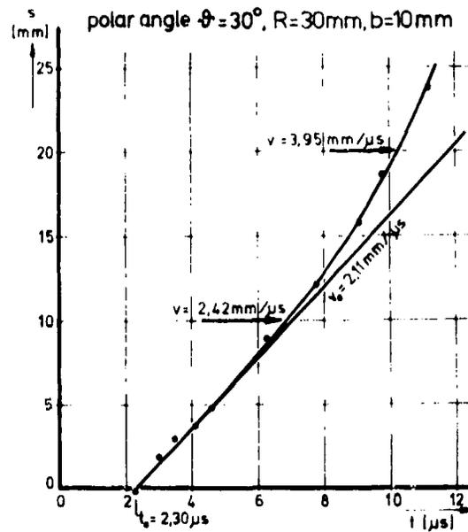
Fig. 5. Definition of initial liner velocity  $v_0$ .
