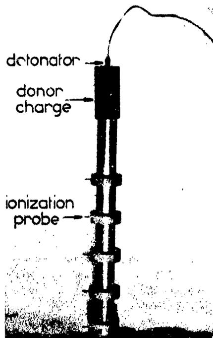
Fig. 1. Standard detonation tube.
