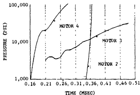
Fig. 6. Maximum pressure-time plots for 6-inch HMX motors
