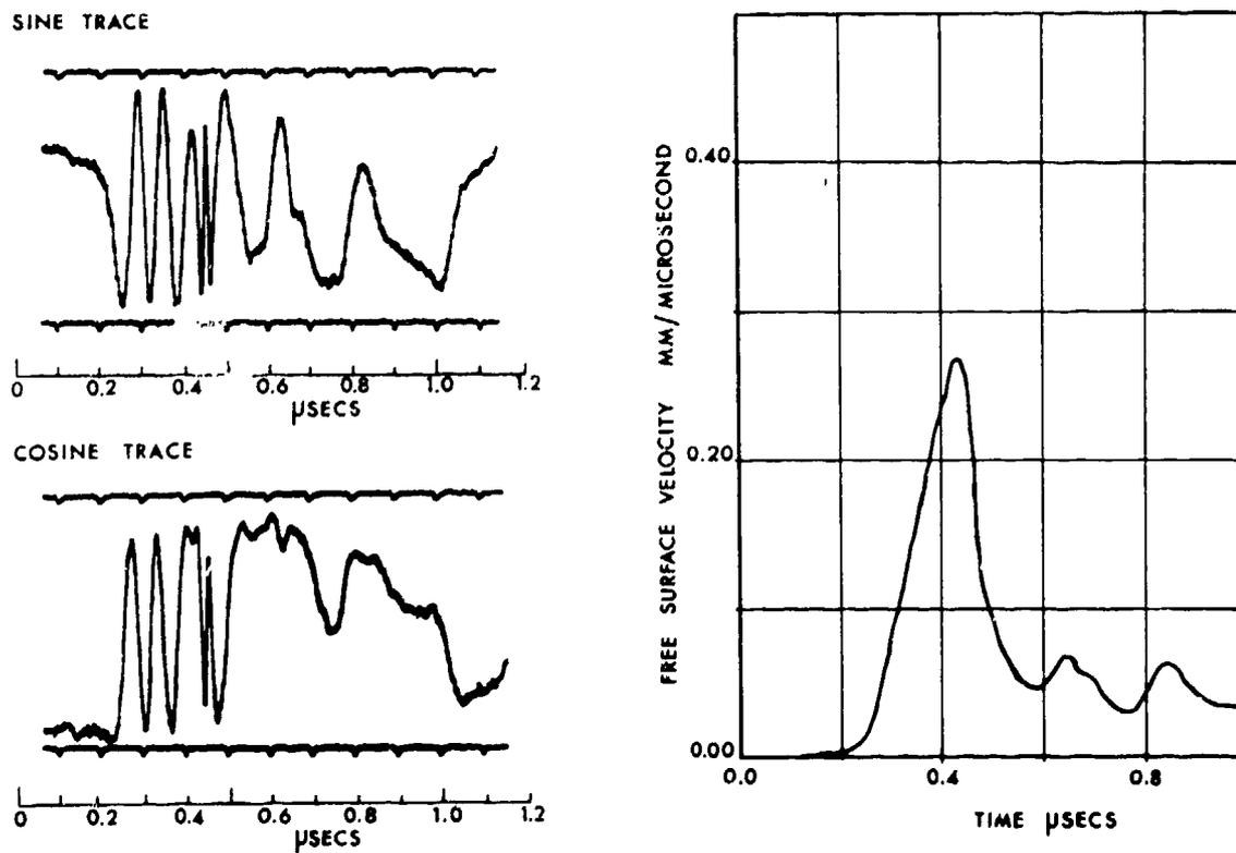
Fig. 7. Records and interpretation of foil impact on Three Dimensional Quartz-fibre Resin Composite (3DQP) 6 mm thick. Foil impact velocity  $0.41 \text{ mm } \mu\text{sec}^{-1}$ . Fringe Constant  $0.10 \text{ mm } \mu\text{sec}^{-1} \text{ Fringe}^{-1}$ .
