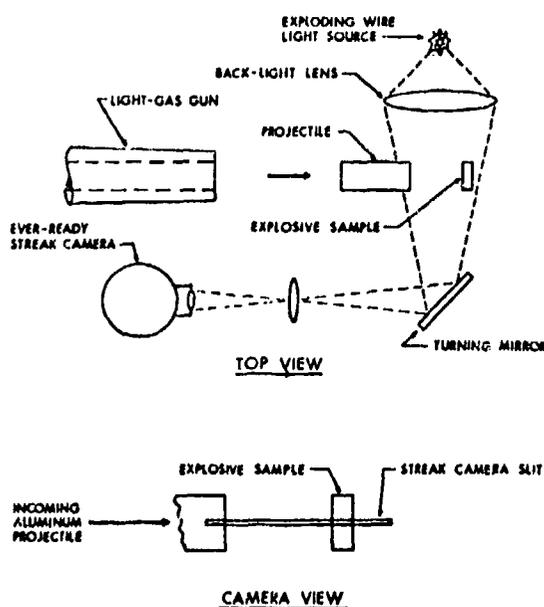
Fig. 1. Experimental arrangement.
