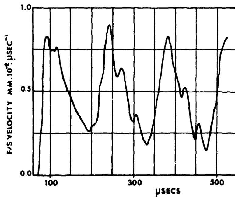
Fig. 8. Records and velocity-time interpretation of low strain rate experiment on CS Carbon. Interferometer Fringe Constant  $0.0088 \text{ mm } \mu\text{sec}^{-1} \text{ Fringe}^{-1}$ .
