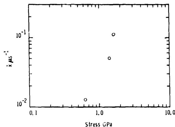
Fig. 6. Calculated decomposition rate vs. stress for HNS at  $\rho_0 = 1.01 \text{ Mg/m}^3$ .
