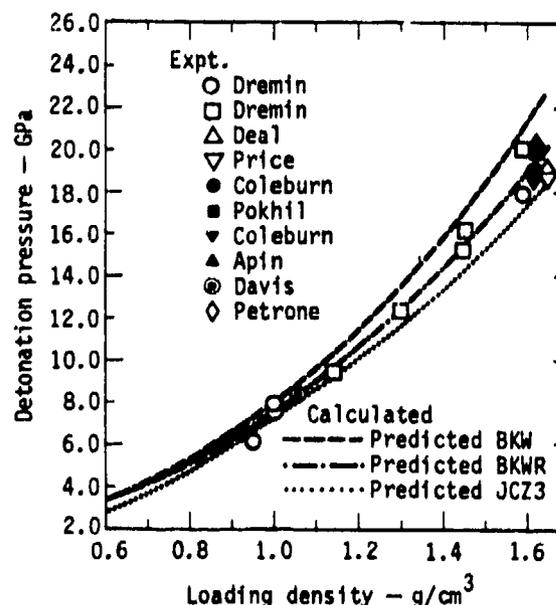
Fig. 2. TNT C-J pressure dependence on loading density.
