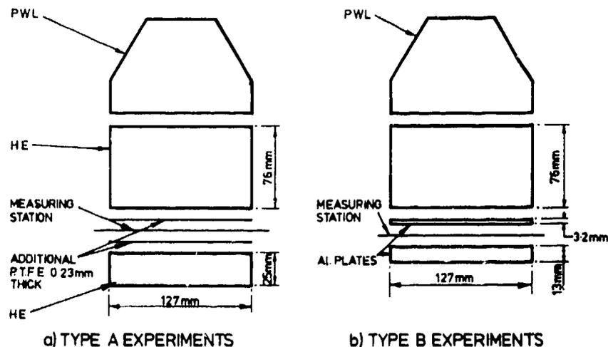
Fig. 2. Experimental layout.
