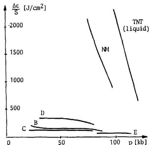
Fig. 10. Energy threshold vs shock pressure.
