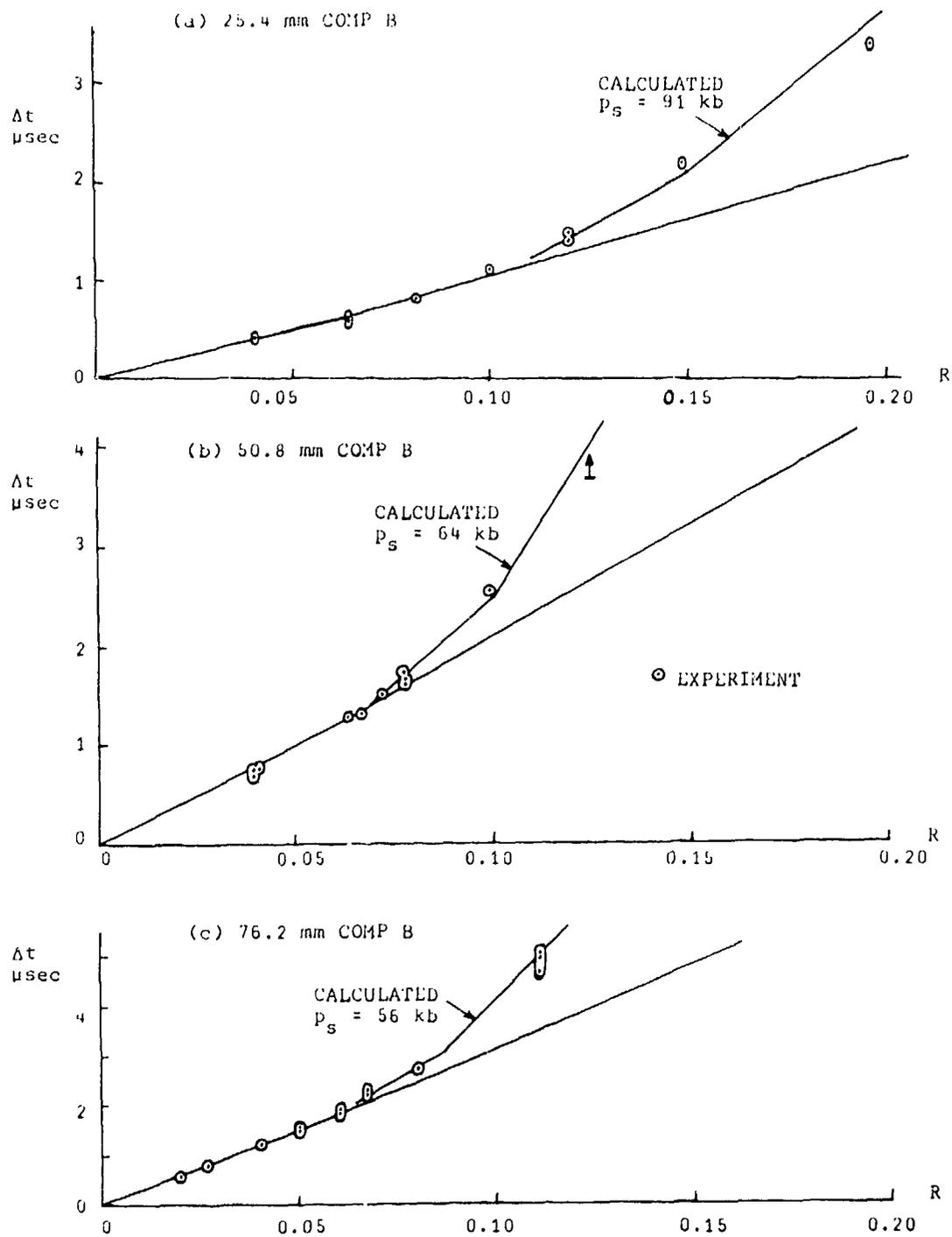
Fig. 10. Reverberation time in non-spalled and spalled plates.
