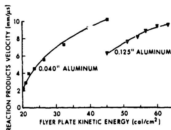
Fig. 7. Energy versus reaction response for 1.30 gm/cc TNT.
