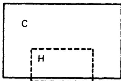
Fig. 1. Explosive charge assembly—schematic view of an explosive disc (H) (28.6 mm diameter X 14.3 mm thick) mounted in a steel or aluminium alloy cup (C) (height 31.8 mm, thickness of base 19.0 mm). The HE protruded 1.5 mm from the metal cup. The wall thickness of the cup was varied as described in the text.
