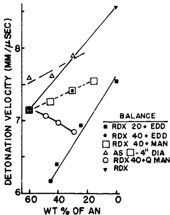
Fig. 2. Detonation velocity results for confined small scale test (9.65 mm).
