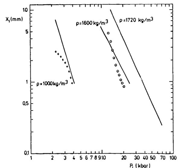
Fig. 2. Log-Log plot of initiation distance vs. initiation pressure for shock wave initiation of pressed PETN with densities of  $1000$ ,  $1600$  and  $1720 \text{ kg/m}^3$ . Full lines represent fitted curves for experimental data (6), the crosses and open dots were calculated.
