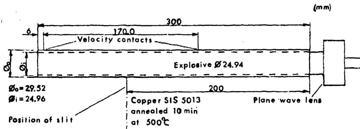
Fig. 1. Specifications on cylinder test arrangement.
