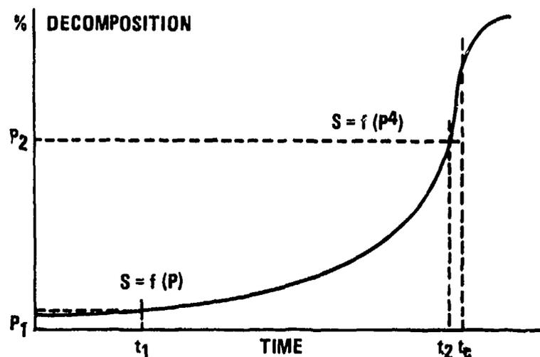
Fig. 2. Explosive decomposition as a function of time
