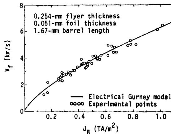
Fig. 4. Flyer velocity vs burst current density.
