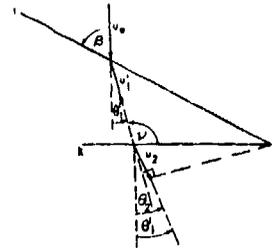
Fig. 3.4. A forward-facing reflected shock  $Ro$ ;  $\nu < 90^\circ$ .
