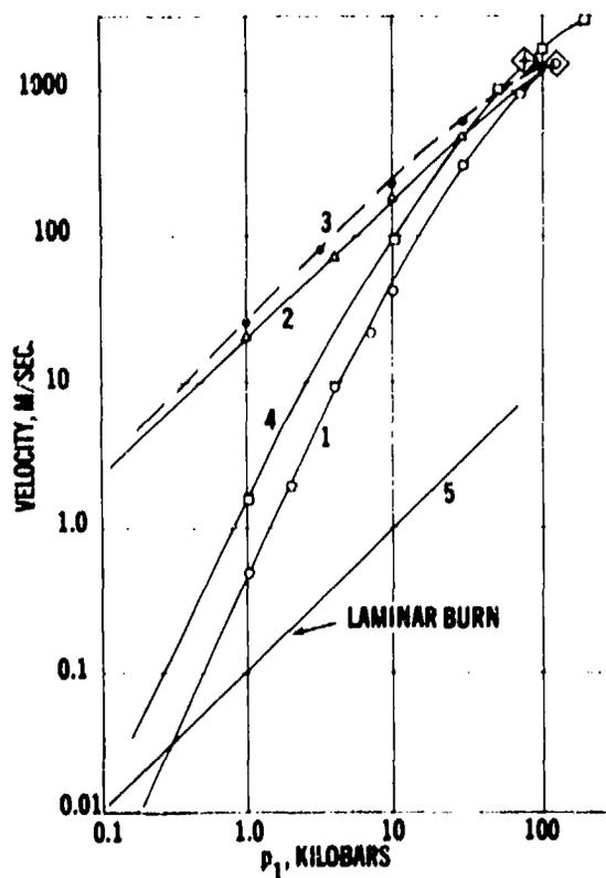
Fig. 11. Deflagration and Particle Velocities. 1).  $W - u_1$  ( $u_2 = 0$ ); 2).  $W - u_1$  (CJ); 3).  $u_1$ ; Tarver, et al. 4).  $W - u_1$  ( $u_2 = 0$ ), Coffey and Jacobs. 5). Laminar flame velocity (approximate).
