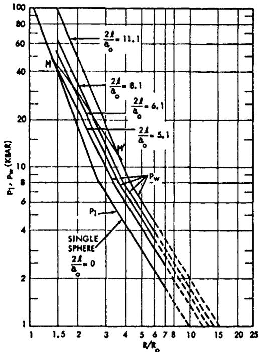
Fig. 6.4. Underwater shock wave pressure  $p_1$  versus  $R/R_0$  curves from a single pentolite sphere, mass  $2M_1$ ; and  $p_W$  versus  $R/R_0$  from separated twin pentolite spheres, each of mass,  $M_1$ .  $2l/a_0$  is the dimensionless separation distance between the twin spheres (after Ref. 15(a) and (c)).
