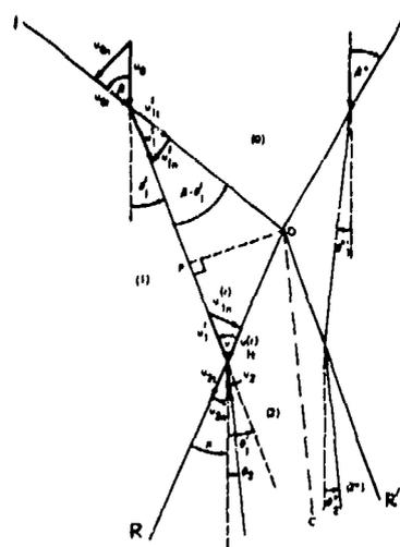
Fig. 3.3. Four-shock configuration.
