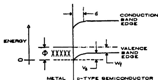
Fig. 1. Energy band diagram for a p-type semiconductor-metal Schottky-barrier contact with thickness  $d$ , barrier height  $\Phi$ , surface potential  $V_s$  and Fermi energy  $W_f$ .
