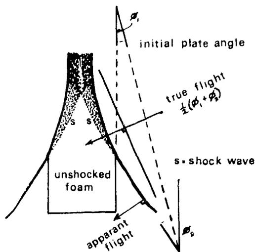
Fig. 2b. Plate flight direction from dynamic radiograph.
