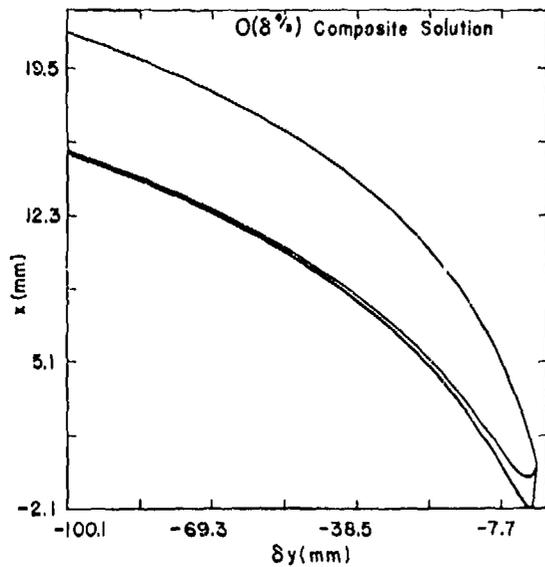
Fig. 3.6.  $O(\delta^{4/3})$  composite solution. The shock locus (upper curve), composite sonic locus (middle curve), and outer sonic locus (lower curve) in edge fixed coordinates. The parameter values are  $D = 8 \text{ mm}/\mu\text{s}$ ,  $\gamma = 3$ ,  $k = 2 \mu\text{s}^{-1}$ , and  $\delta = 0.1$ .
