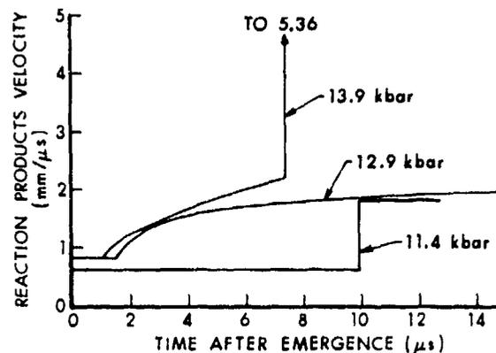
Fig. 5. Reaction products velocity versus time.
