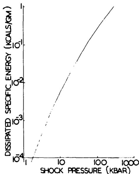
Fig. 1. Variation of energy dissipation with shock pressure.
