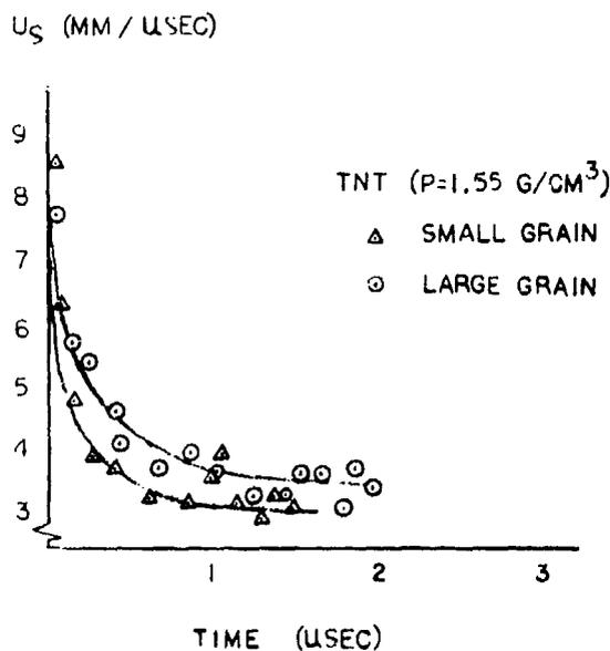
Fig. 9. Shock velocity versus time to detonation for pressed TNT.
