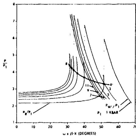
Fig. 3.21.  $p_R/p_1$  and  $p_{W'}/p_1$  versus  $\omega = \beta - \chi$  at different values of  $p_1$  for water using the S-W equation of state.  $RR'$  is the locus of points at which regular reflection fails.
