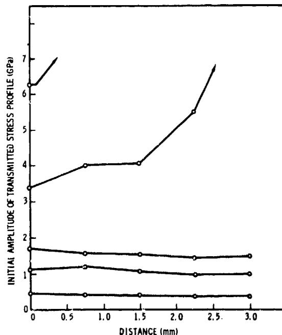
Fig. 13. Variation of stress amplitude with propagation distance for high-density HNS.
