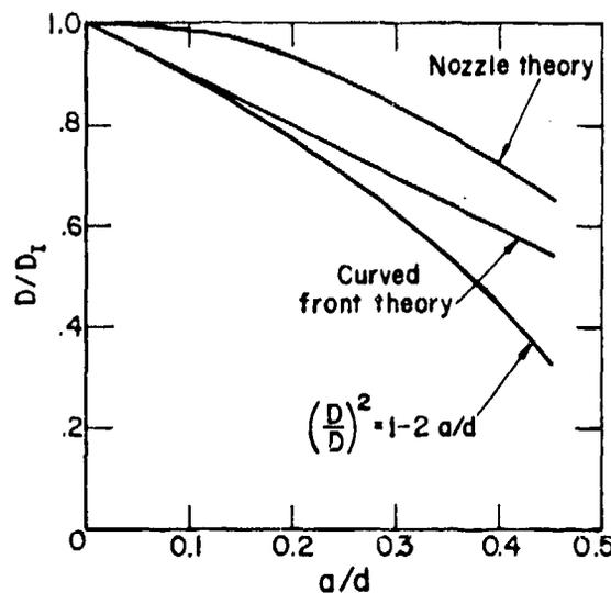
Fig. 1.  $D/D_I$  vs.  $a/d$  for Various Failure Theories.
