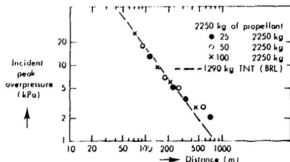
Fig. 4. Peak pressure versus distance diagram.
