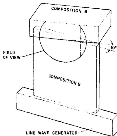
Fig. 4a. Corner turning in Composition B. The line detonation in the thin ( $\sim 4$  mm) slab of explosive intersects the thick piece above at an angle, so the wave can be seen by multiple exposure at several different distances from the intersection.
