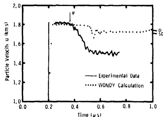
Fig. 6. Comparison of computed particle velocity history at the Cu/NM interface with Hardesty's experimental observation (9) in shot N8, where  $p^- = 9.2$  GPa and  $\theta^- = 1101$  K. Velocity levels SD and D refer to boundary conditions behind superdetonation and detonation, respectively, independently calculated, using TIGER (11).
