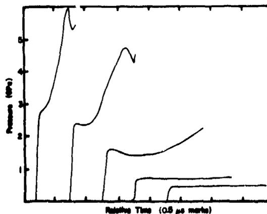
Fig. 5. Typical impact-face pressure histories measured with quartz gauges.
