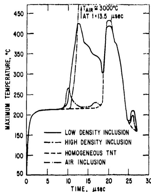
Fig. 6. Effect of inclusions on maximum temperature (hydrodynamic).
