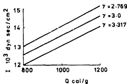
Fig. 2. Dependence of pulse width  $\theta$  on  $Q$  and  $\gamma$  at  $R = 10.3 \text{ cm}$  ( $\rho_o = 1.6 \text{ gm}^{-3}$ ).
