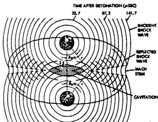
Fig. 4.2. Experimental time profiles of the collision of two equal spherically expanding underwater shock waves showing Mach wave formation; 10.9  $\mu\text{sec}$  between successive wave fronts;  $2\ell = 7.6a_0$ ; bubble motion not shown (after Ref. 15(a)).
