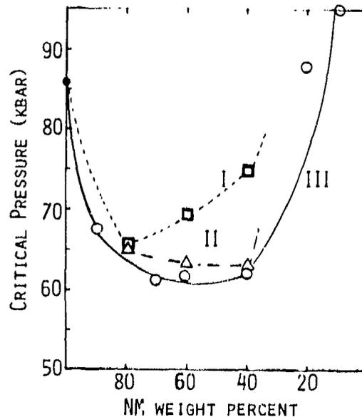
Fig. 5. Critical initiation pressures of NM-UPS-water mixtures.
