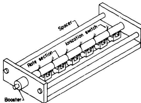
Fig. 1. Schematic of a typical rate-stick assembly.
