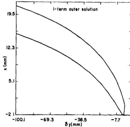
Fig. 3.3. 1-term outer solution. The shock locus (upper curve) and the sonic locus (lower curve) in edge fixed coordinates. The parameter values are  $D = 8 \text{ mm}/\mu\text{s}$ ,  $\gamma = 3$ , and  $k = 2 \mu\text{s}^{-1}$ .
