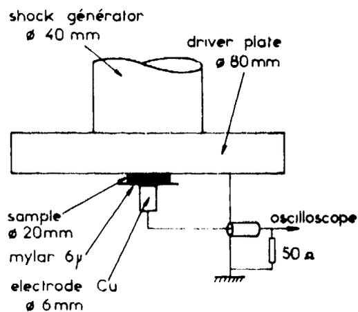
Fig. 1. Schematic of an experimental arrangement for shock behavior investigation of lamellar Al-Cu composites.
