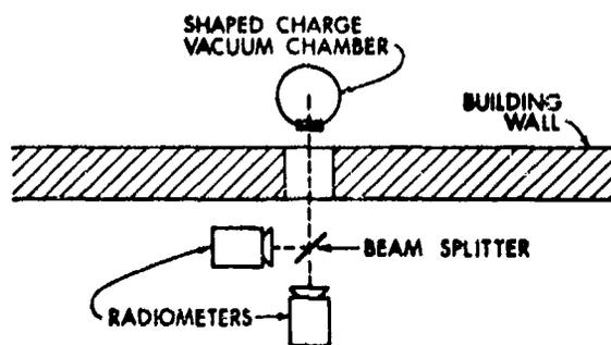
Fig. 12. Schematic of the experimental arrangement used to produce two colinear optical paths.
