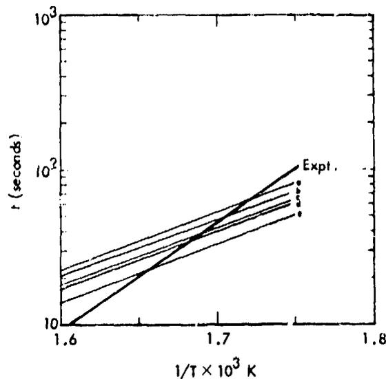
Fig. 10. The effect on predicted times to explosion by variation of heat capacity ( $C$ ) and thermal conductivity ( $\lambda$ ) in equation 1. (a)  $C = 0.5 - 0.6$ ,  $\lambda = .0005 - .0001$ ; (b)  $C = 0.5$ ,  $\lambda = .0005 - .0001$ ; (c)  $C = 0.5 - 0.6$ ,  $\lambda = .0005 - .0003$ ; (d)  $C = 0.5 - 0.7$ ,  $\lambda = .0005$ ; (e)  $C = 0.5$ ,  $\lambda = .0005$ .
