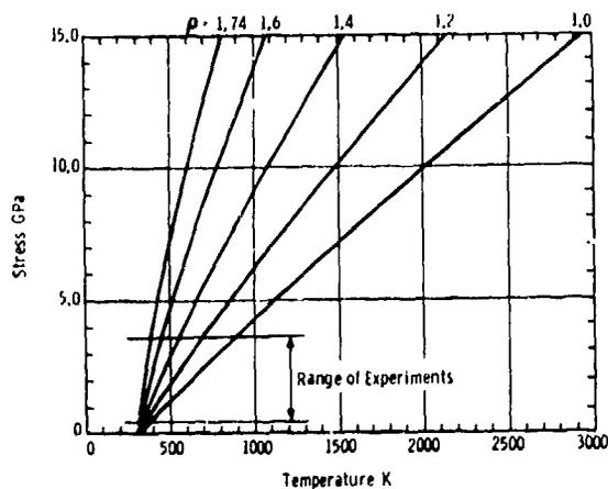
Fig. 4. Calculated stress-temperature Hugoniot for HNS at various initial densities.
