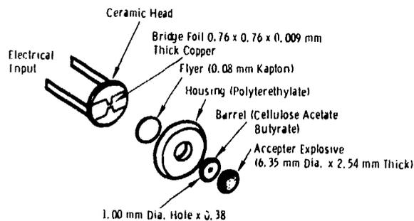
Fig. 1. Exploded view of the test device.
