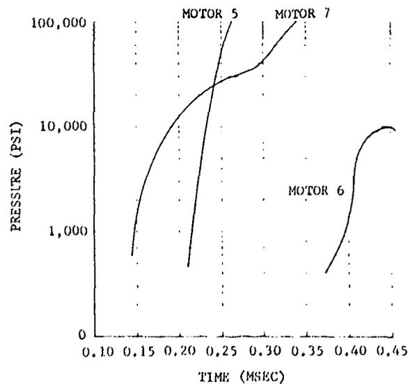
Fig. 8. Maximum pressure-time plots for Motors 5, 6, and 7
