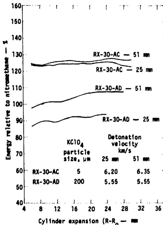
Fig. 14. Relative energy of RX-30-AC and AD.
