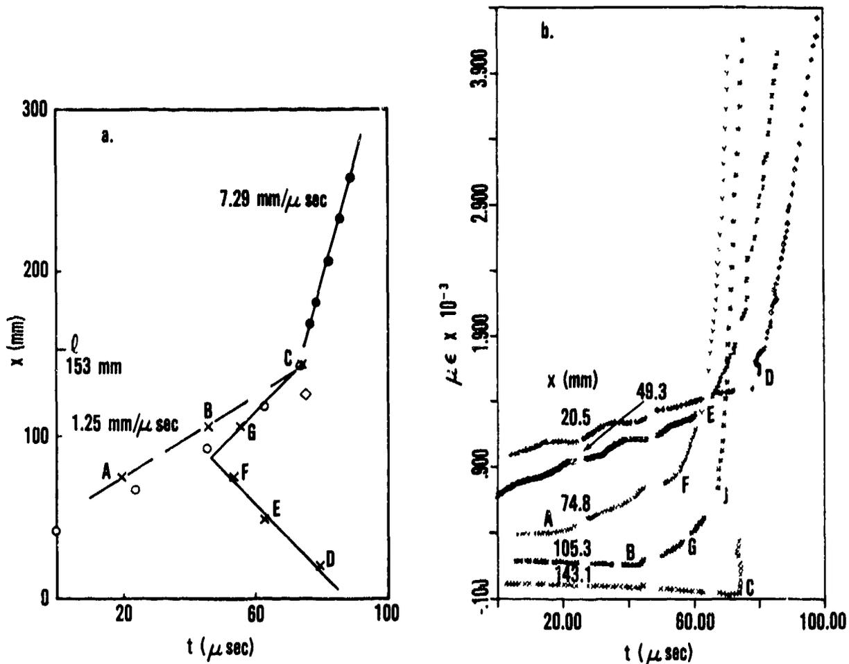
Fig. 2. Data for shot 613 on  $470\mu$  tetryl at 85% TMD,  $\rho_0 = 1.47 \text{ g/cc}$ . [a. distance-time plot ( $\circ$  custom-made probes,  $\bullet$  commercial probes,  $\times$  change in slope of  $e$ - $t$  curve of b,  $\diamond$  coalescence of isobars); b. strain-time plots (change of slope shown by letters which also appear in a. Each curve except the lowest has been raised  $0.2 \times 10^{-3} \mu \epsilon$ , or an integral multiple thereof, for better data display.)]
