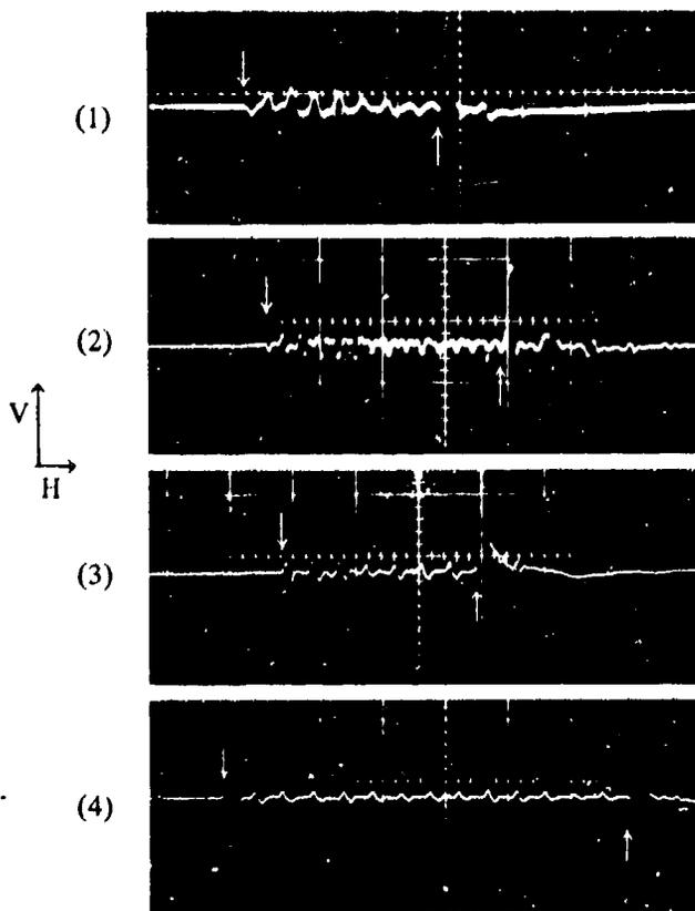
Fig. 2. Typical records of the shock wave propagation in lamellar Al-Cu samples.
