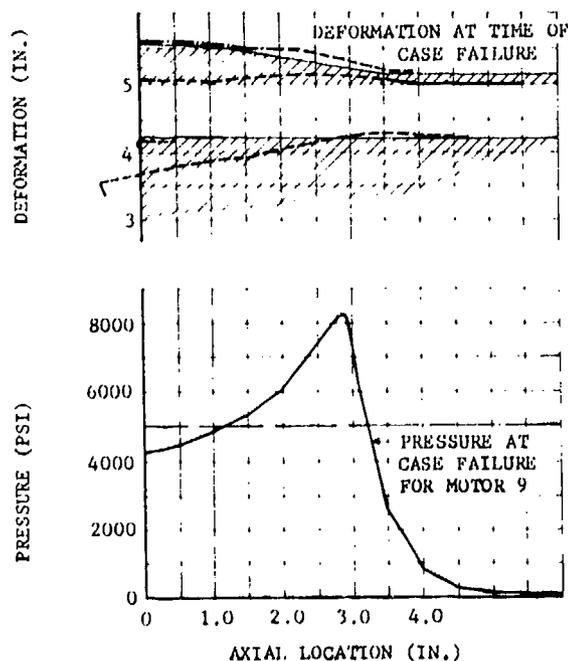
Fig. 9. Pressure and deformation of lightweight case
