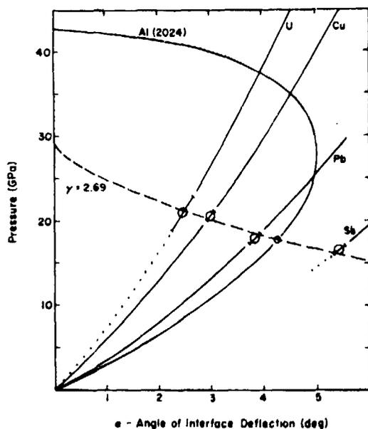
Fig. 3. Perpendicular drive by Composition B-3. The solid lines are the oblique solutions obtained from the reference Hugoniots. The dotted lines cover ranges into which the reference Hugoniots have been extrapolated. The dashed line is the Prandtl-Meyer expansion of detonation products described by a polytropic gas equation.
