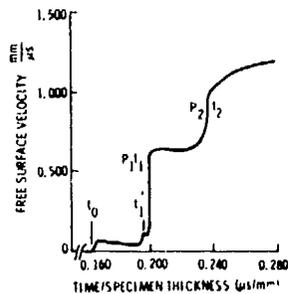
Fig. 6. Free surface velocity history of iron impacted at 25 GPa. Data from Barker<sup>3</sup>.
