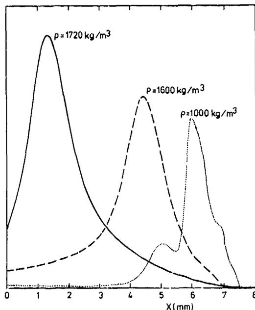
Fig. 3. Reacted fraction  $f$  ( $f$  between 0 and 1 and different scale uni's for the three curves) as a function of distance in explosive, 0.04, 0.03 and 0.02  $\mu$ s before detonation sets in, for the densities 1720, 1600 and 1000  $\text{kg/m}^3$  respectively.
