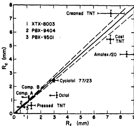
Fig. 7. Correlation between  $R_f$  and  $R_c$ . The hashed lines correspond to plus or minus one standard deviation of the slope of the line. Where no error bars are indicated they are less than the dot size; where error bars are indicated they are those of Table I. The equation of the straight line is  $R_c = (0.877 \pm 0.054) R_f$ . An arrow to the left of an entry indicates that no sticks that failed were fired.
