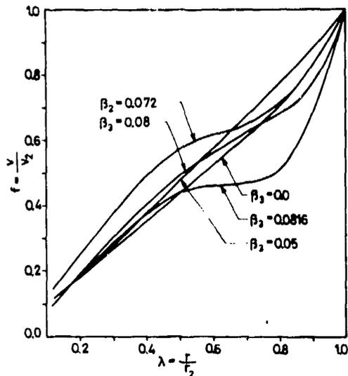
Fig. 5. Graphs of  $f(\lambda)$ , the dimensionless gas velocity for various  $\beta_3$  ( $\gamma = 1.4$ ).
