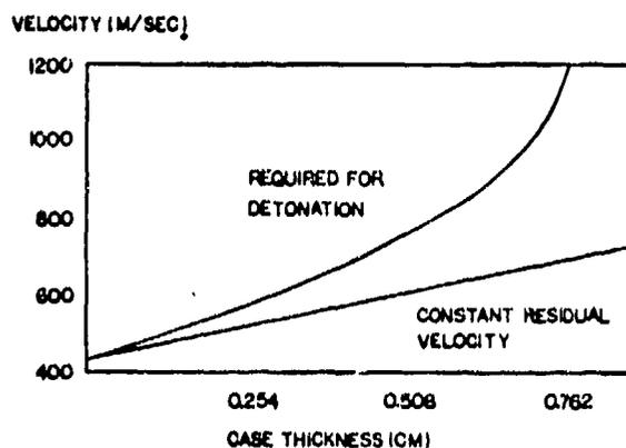
Fig. 2. The impact velocity required for detonation and the impact velocity required to maintain a constant residual velocity are shown as a function of case thickness. The explosive is tetryl, and the projectile is 1.27 cm long and 1.27 cm in diameter. The case and the projectile are steel.
