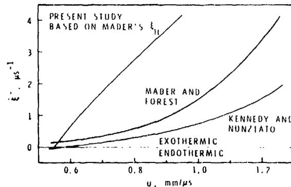
Fig. 4. Reaction rate,  $\xi^-$ , immediately behind the shock front as a function of shock amplitude for several models of shock response of PBX-9404. Kennedy and Nunziato (20) adopted the ZND model, i.e.,  $[\xi] = 0$ . We used Mader's function  $\xi_{II}$  together with the data of Kennedy and Nunziato to derive the upper curve, via (4.2).
