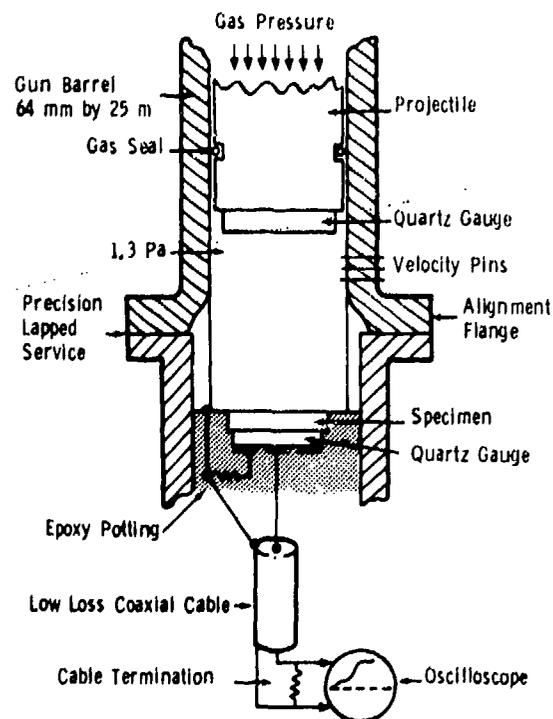
Fig. 1. Experimental configuration, slightly modified from Ref. 5.
