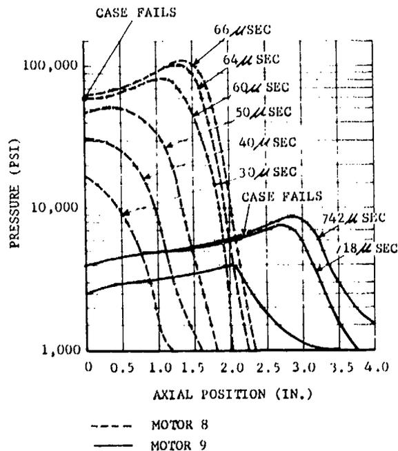
Fig. 10. Comparison of pressure-distance traces of Motors 8 and 9
