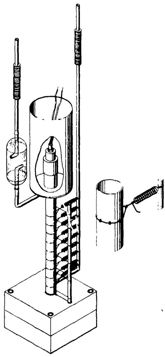
**Fig. 3. Shot Assembly for Measuring the Detonation Velocity of Nitric Oxide.**
