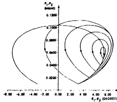
Fig. 3.13. Change in the reflected shock polars for water ( $\gamma$ -law equation of state, Eq. 2.2,  $\gamma = 7.15$ ) as the incident pressure  $p_1$  is increased from 10 kbar in 10 kbar increments for fixed  $p_{1,max} = 103.5$  kbar. The sonic point for each polar is denoted by an asterisk \*.
