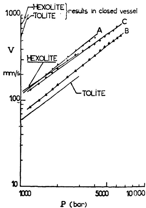
Fig. 11. Regression rate curves on high explosives.
