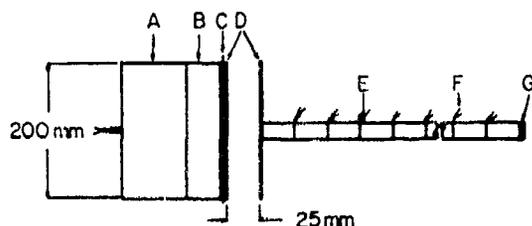
Fig. 10. Diagram of overboosted rate stick assembly.
