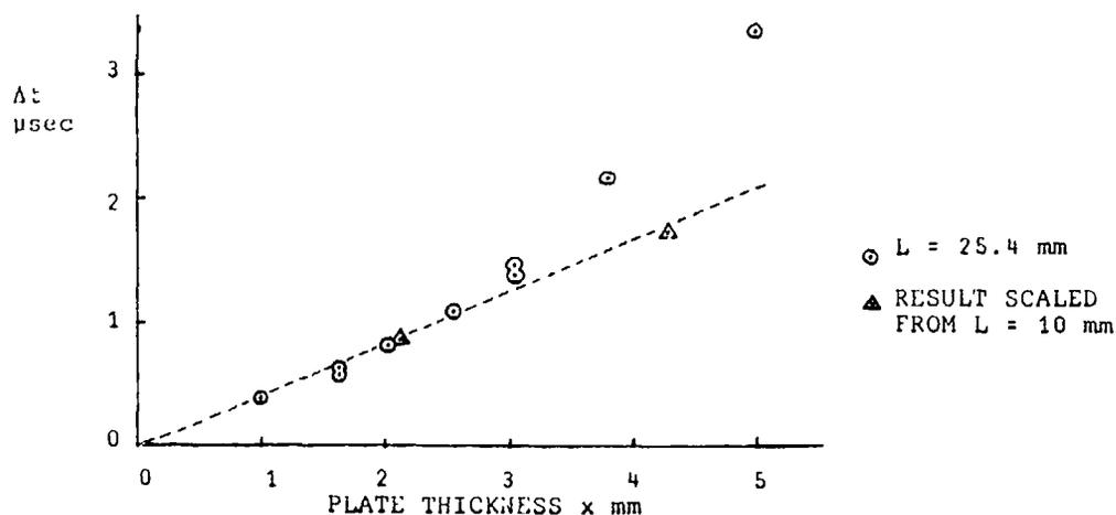
Fig. 2.  $\Delta t$  versus  $x$  for stainless steel plate on Comp. B,  $L = 25.4 \text{ mm}$ .
