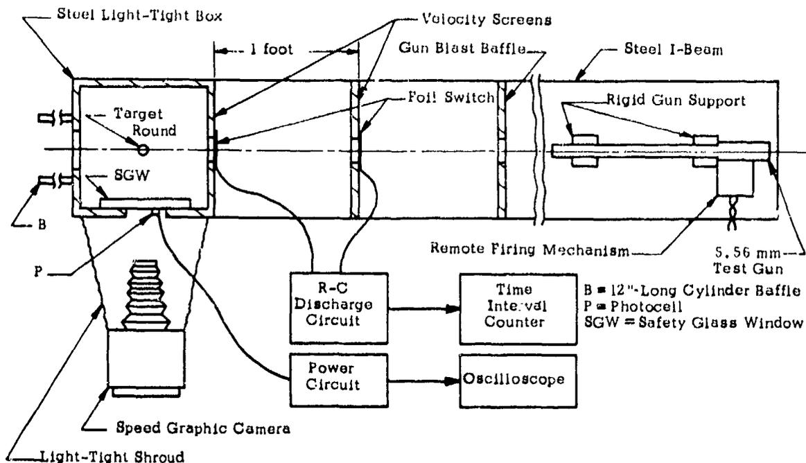
Fig. 3. Experimental configuration for bullet impact tests.
