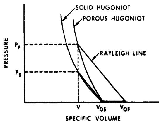
Fig. 2. Shock compression of solid and porous explosives.
