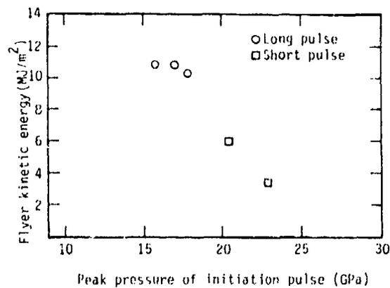
Fig. 7. Threshold flyer kinetic energy is shown for 92.5/7.5 TATB/KEL-F,  $\rho = 1.90 \text{ Mg/m}^3$ .
