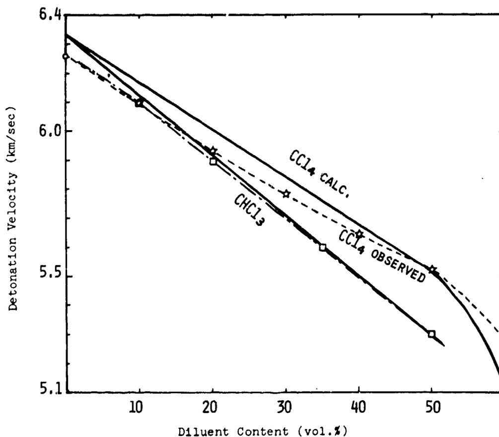
Fig. 7. Detonation velocity at infinite diameter against diluent content for the mixtures NM with  $CHCl$  and  $CCl$ .
