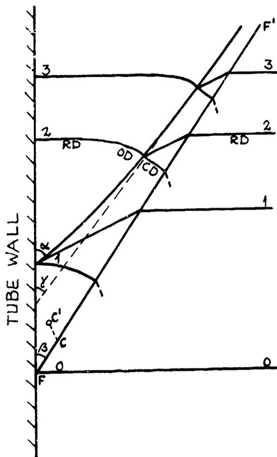
Fig. 3. Schematic diagram of triple wave interactions in a single convergent dark wave.  $F-F'$ : failure line,  $R-R'$ : strong reinitiation line,  $RD$ : regular detonation front,  $OD$ : overdriven detonation front,  $CD$ : detonation front in shock compressed material,  $S$ : shock front.
