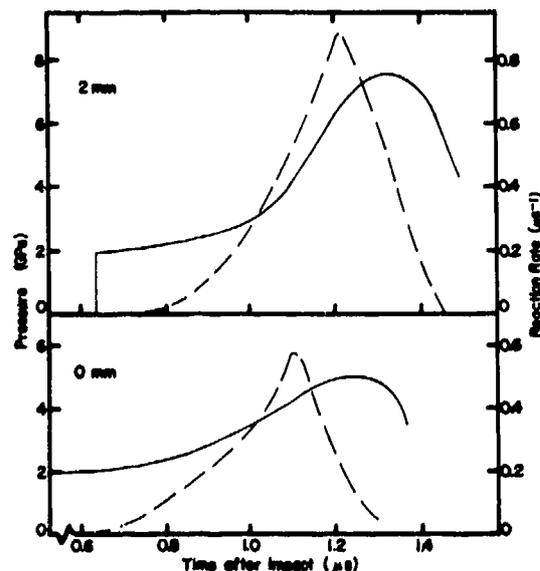
Fig. 11. Pressure histories and calculated reaction rates at the impact face and at 2-mm depth.
