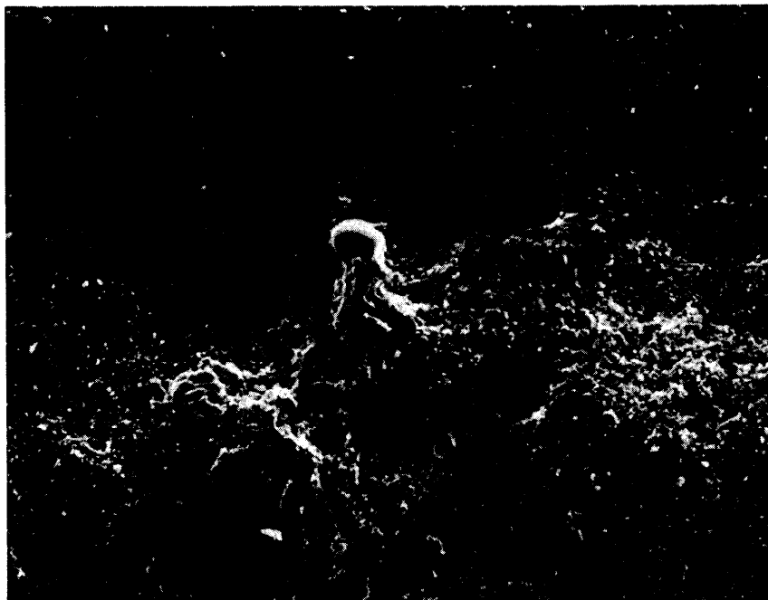
Figure A-9B. Fracture origin (iron inclusion) in specimen B-Fe-F-3 at 50X (above) and 200X (below). Note presence of slow crack growth and liquid formation.
