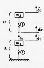
$$\mu_{\sigma}\omega_{\sigma}^{2} = \phi_{\sigma}^{T}K_{\sigma}\phi_{\sigma} = \begin{bmatrix} 0 & 0 \\ 0 & k_{2} \end{bmatrix}, \quad \mu_{S} = m_{1}; \quad \omega_{S}^{2} = k_{1}/m_{1}; \quad \overline{\phi}_{S} = 1$$
