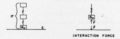
There are a number of advantages in considering the main structure separately, and accounting for the substructure by means of the constraint forces. First, the computer core (central memory) required to solve a given problem is reduced, since no total system modal stiffness matrix is needed. Second, once the constraint modes have been determined, only those rows of  $K_{\sigma}$  (the unconstrained stiffness matrix of  $\sigma$ ) that correspond
