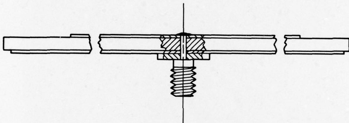
FIG. 3 DETAIL OF PATCH RADIATOR REAR FEED STRUCTURE
