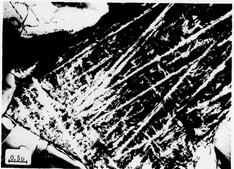
Figure 4. TEM taken from the 2 inch thick specimen showing the martensite laths.
