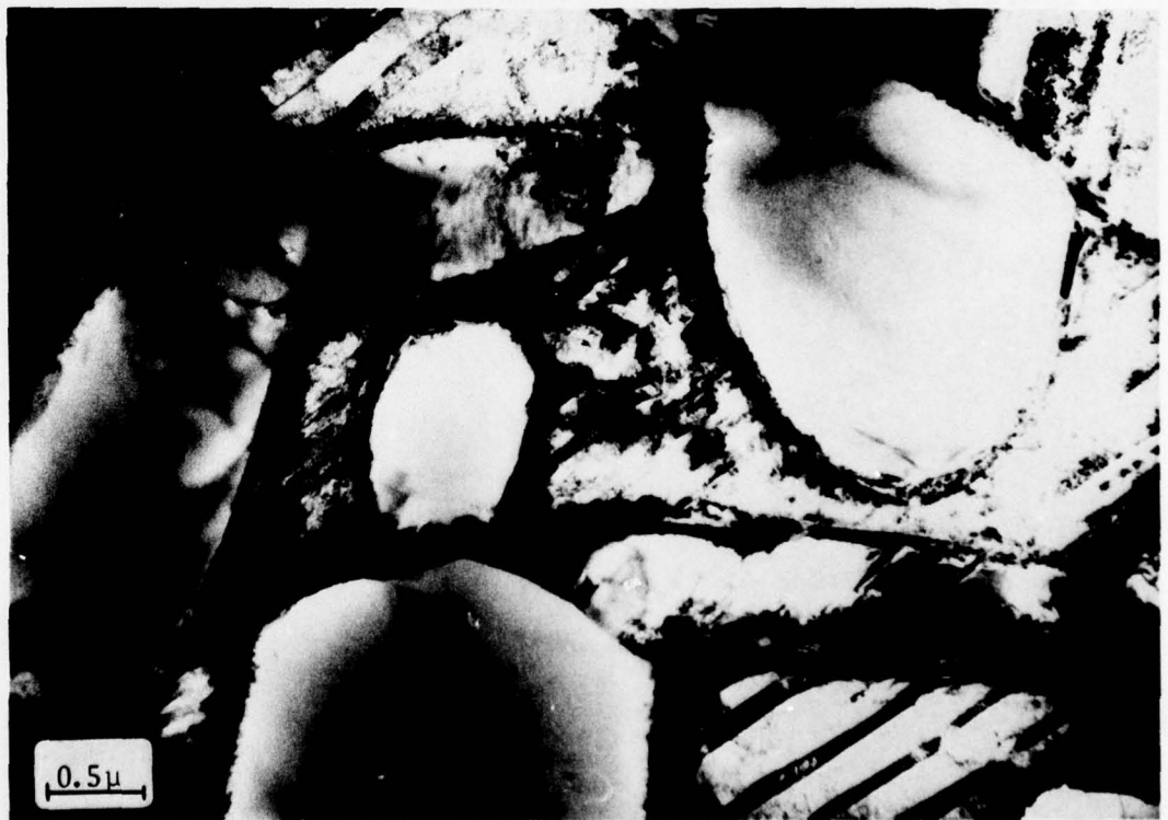
Figure 2. Transmission electron micrograph of Ti-6Al-4V after heat treating at 900°C for 10 minutes followed by a water quench.
