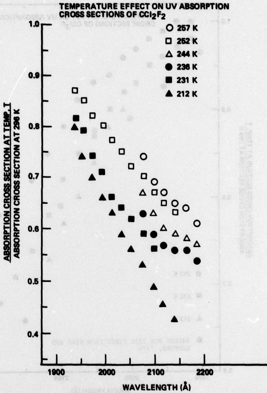
Figure 12: Ratio of the Absorption Cross Section of  $\text{CCl}_2\text{F}_2$  at Temperature T to that at 296K. (T= 257, 252, 244, 236, 231, 212K)
