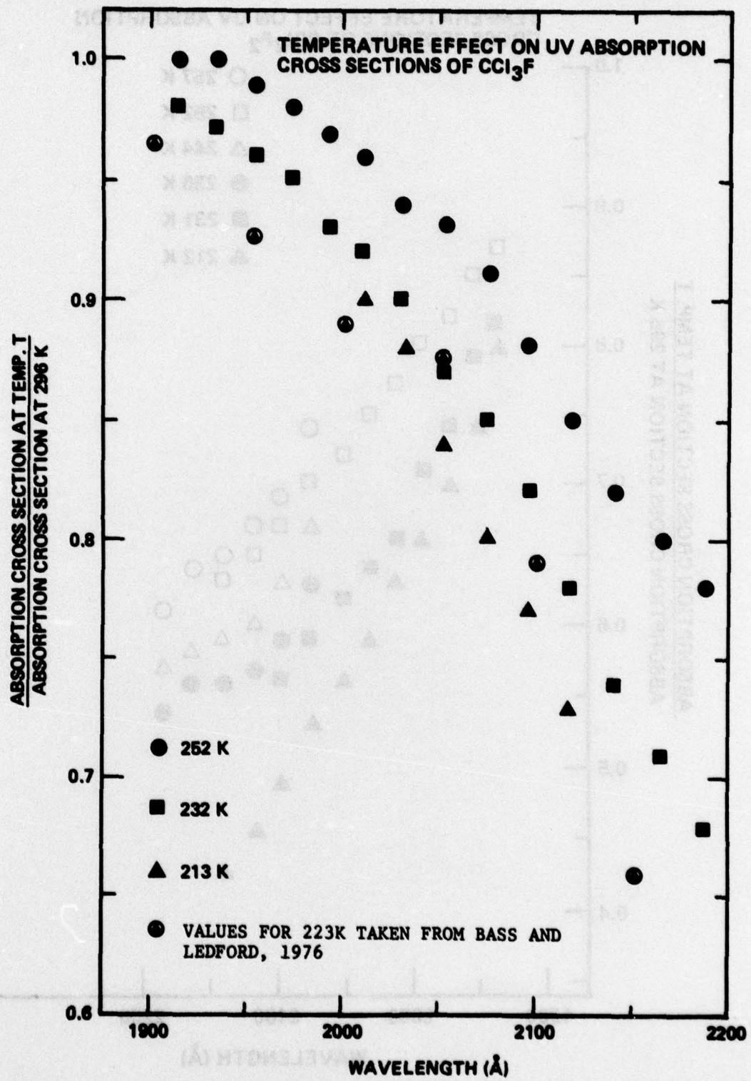
Figure 13: Ratio of the Absorption Cross Section of  $\text{CCl}_3\text{F}$  at Temperature T to that at 296K. (T=252, 232, 213K)
