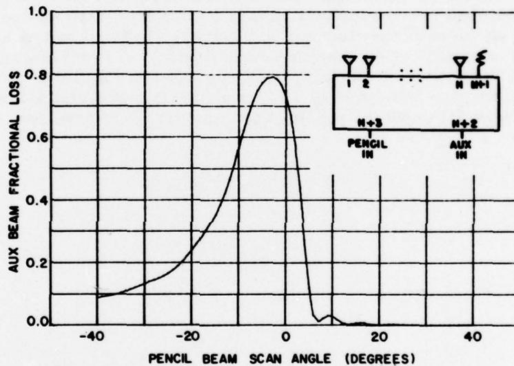
Fig. C1 - Power dumped when the  $\text{csc}^2$  beam and the scanning pencil beam use a common aperture
