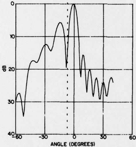
Fig. 10a - Auxiliary-beam pattern with elements 44 through 61 driven for  $\lambda_0 = 0.95$  and  $\lambda = 1.03$  (directivity = 15.6 dB, 29.7 percent of the input power dumped, and gain = 14.1 dB)
