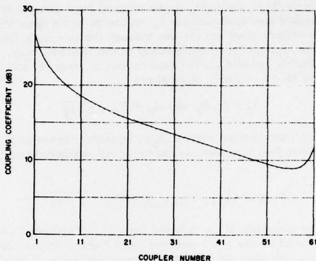
Fig. 3 — Coupling coefficients for a 61-element sinuous feed
