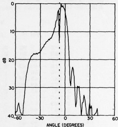
Fig. 5b - Auxiliary-beam pattern with elements 1 through 18 driven for  $\lambda_0 = 1.01$  and  $\lambda = 1.01$  (directivity = 15.3 dB, 0.3 percent of the input power dumped, and gain = 15.3 dB)
