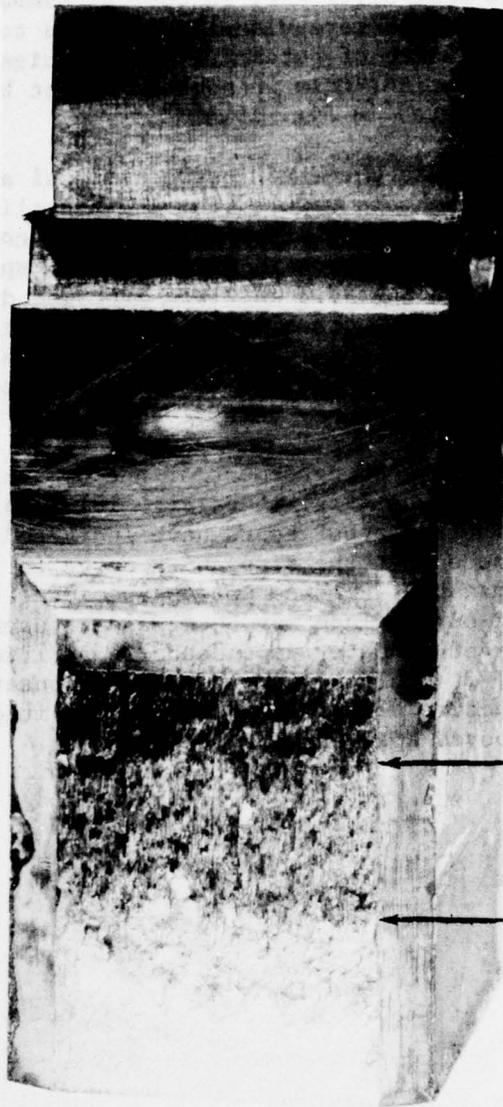
**Fig. 17 - Fracture surface of a specimen that has been face-grooved. This specimen illustrates the crack front shape at two points in the loading history (indicated by arrows). Face grooving effectively eliminates the crack-front curvature that was illustrated in Fig. 16.**
