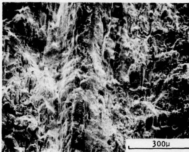
FIGURE 28. FRACTOGRAPH OF DIFFUSION BONDED 7475 A1/1100 A1 LAMINATE DA4 CT FAILURE SURFACE SHOWING INTERLEAF REGION.
