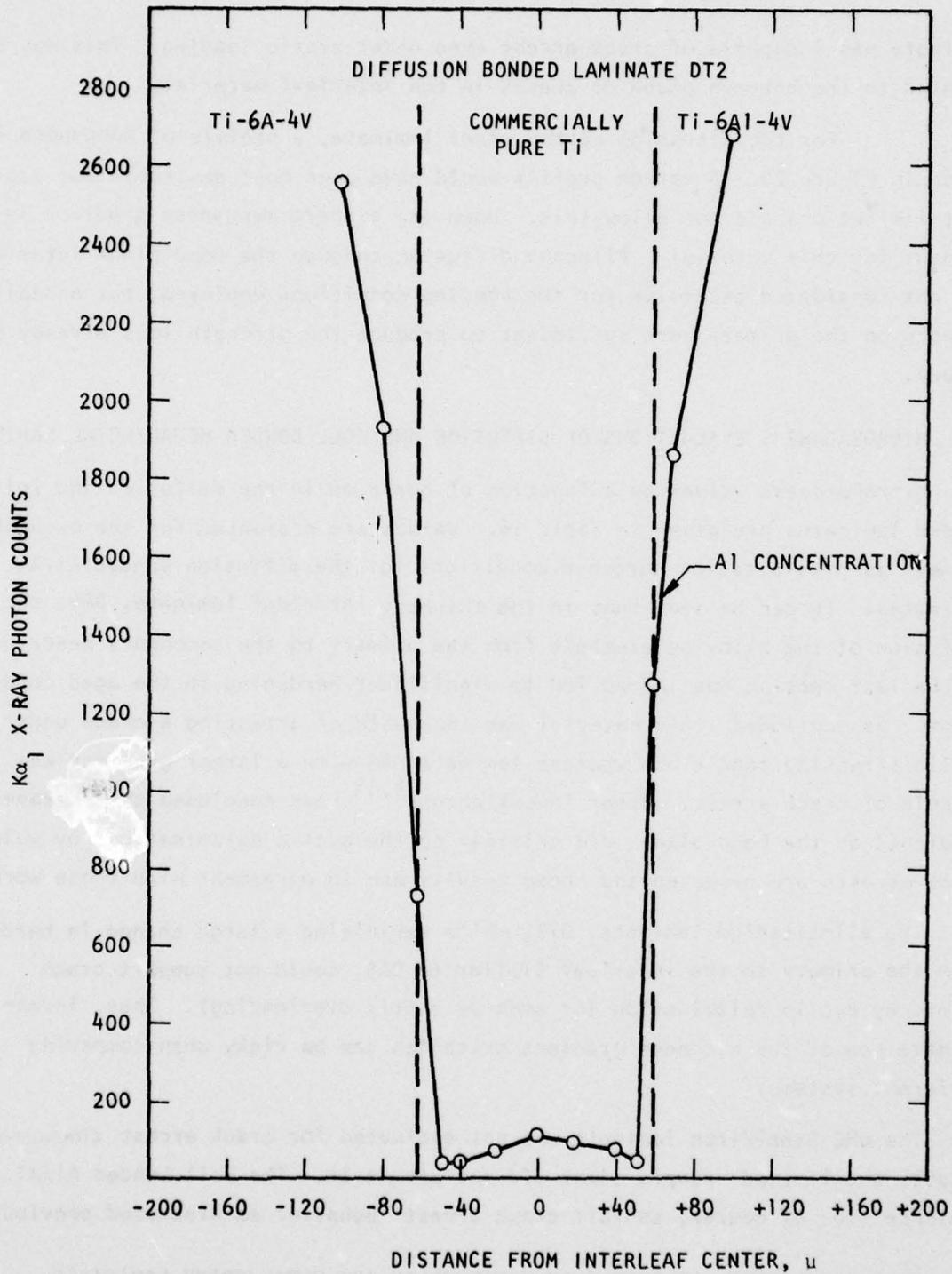
FIGURE 19. Al DIFFUSION PROFILE ACROSS 0.13 mm (0.005 in.) COMMERCIALY PURE Ti INTERLEAF IN DIFFUSION BONDED Ti-6Al-4V/CPTi LAMINATE DT2.
