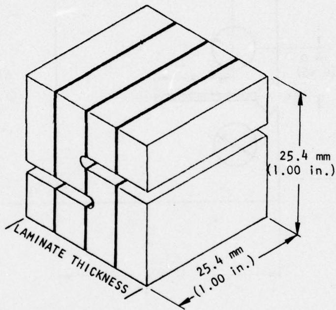
FIGURE 3. COMPACT COMPRESSIVE LAP SHEAR SPECIMEN.
