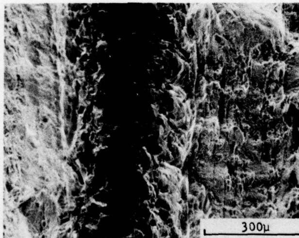
FIGURE 29. FRACTOGRAPH OF DIFFUSION BONDED 7475 A1/1100 A1 LAMINATE DA5 CT FAILURE SURFACE SHOWING INTERLEAF REGION.
