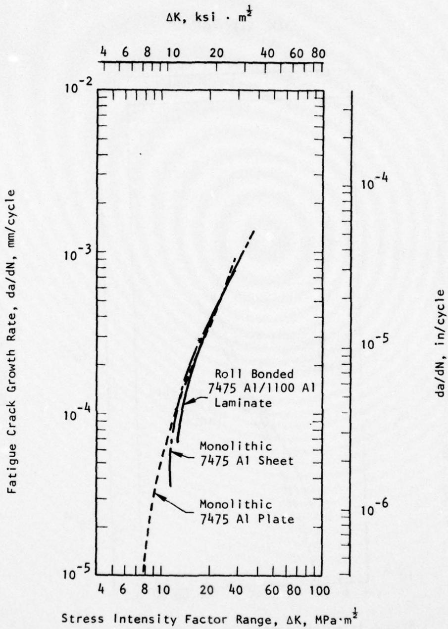
FIGURE 38. FATIGUE CRACK PROPAGATION RATES FOR MONOLITHIC 7475-T651, -T7651 AL SHEET AND PLATE AND ROLL BONDED RA4, CRACK DIVIDER, L-T ORIENTATION, OVERLOAD RATIO = 1.5.
