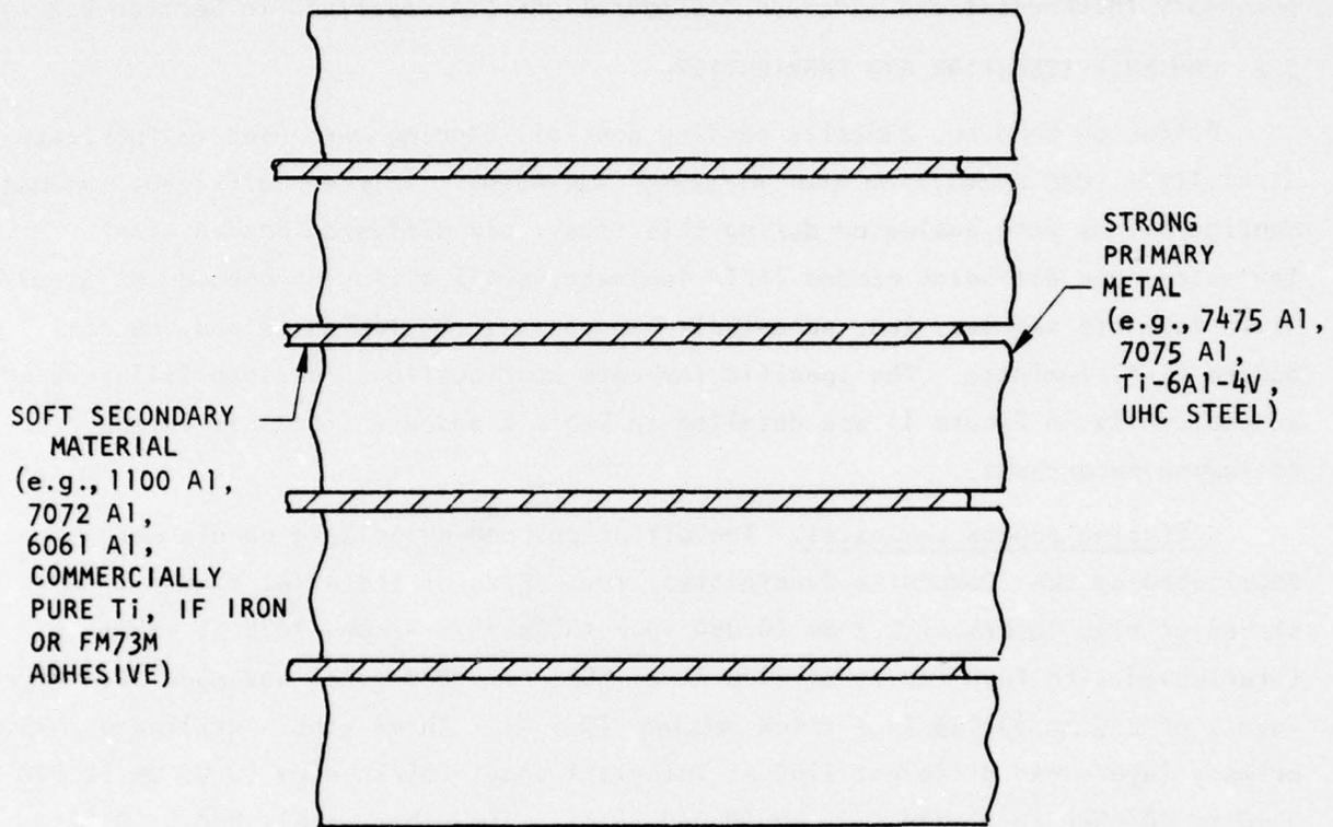
FIGURE 1. SCHEMATIC OF METAL/METAL LAMINATE INVESTIGATED.
