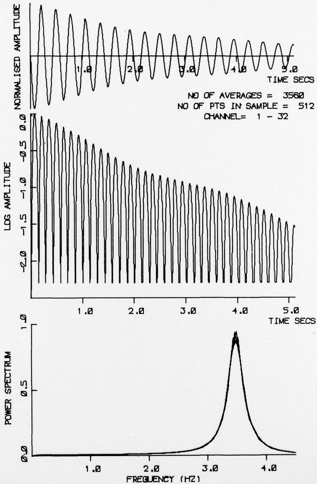
FIG. 11 RANDOM DECREMENT ANALYSIS (absorber locked)
