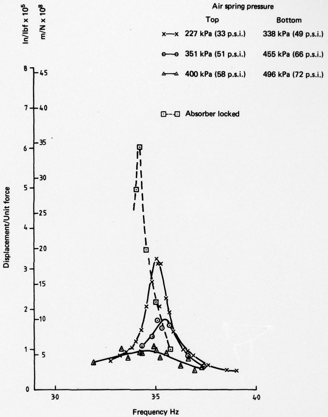
FIG. 8 EFFECT OF ABSORBER TUNING ON SHIP RESPONSE
