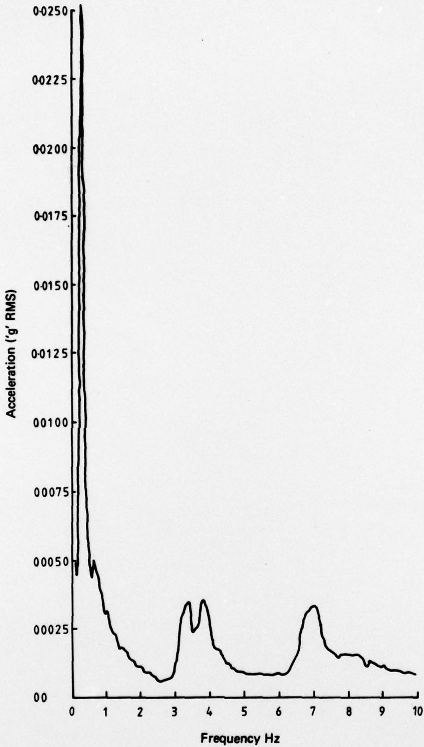
FIG. 17 FREQUENCY SPECTRUM OF RESPONSE (absorber correctly tuned)
