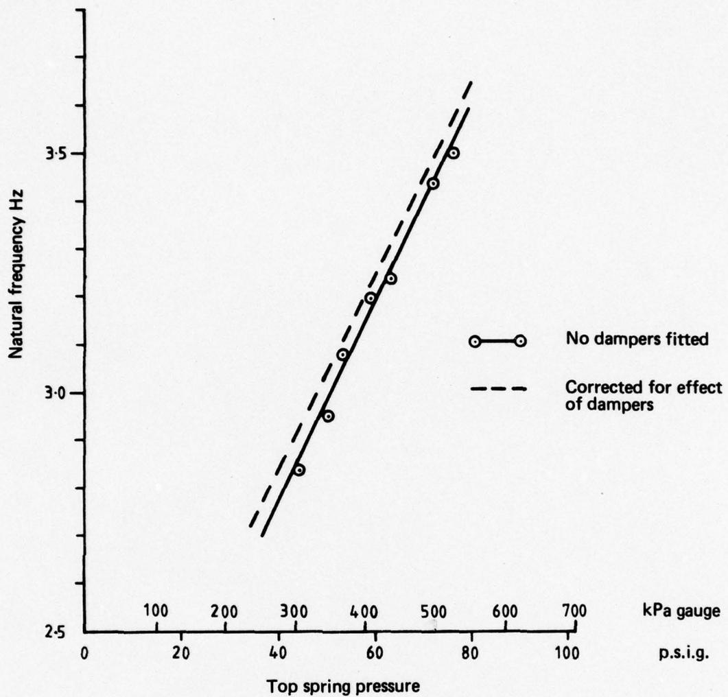
FIG. 5 VARIATION OF ABSORBER NATURAL FREQUENCY WITH PRESSURE
