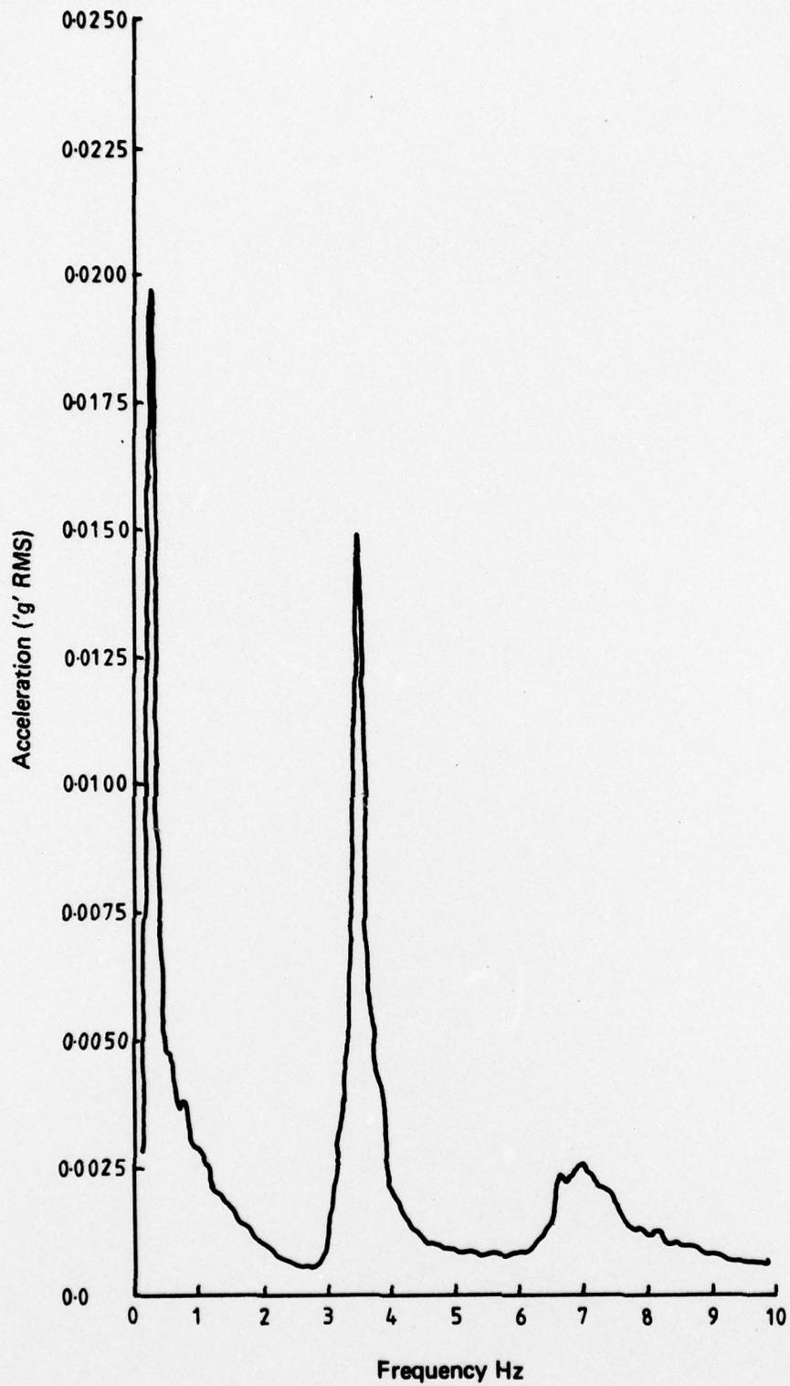
FIG. 16 FREQUENCY SPECTRUM OF RESPONSE (absorber locked)
