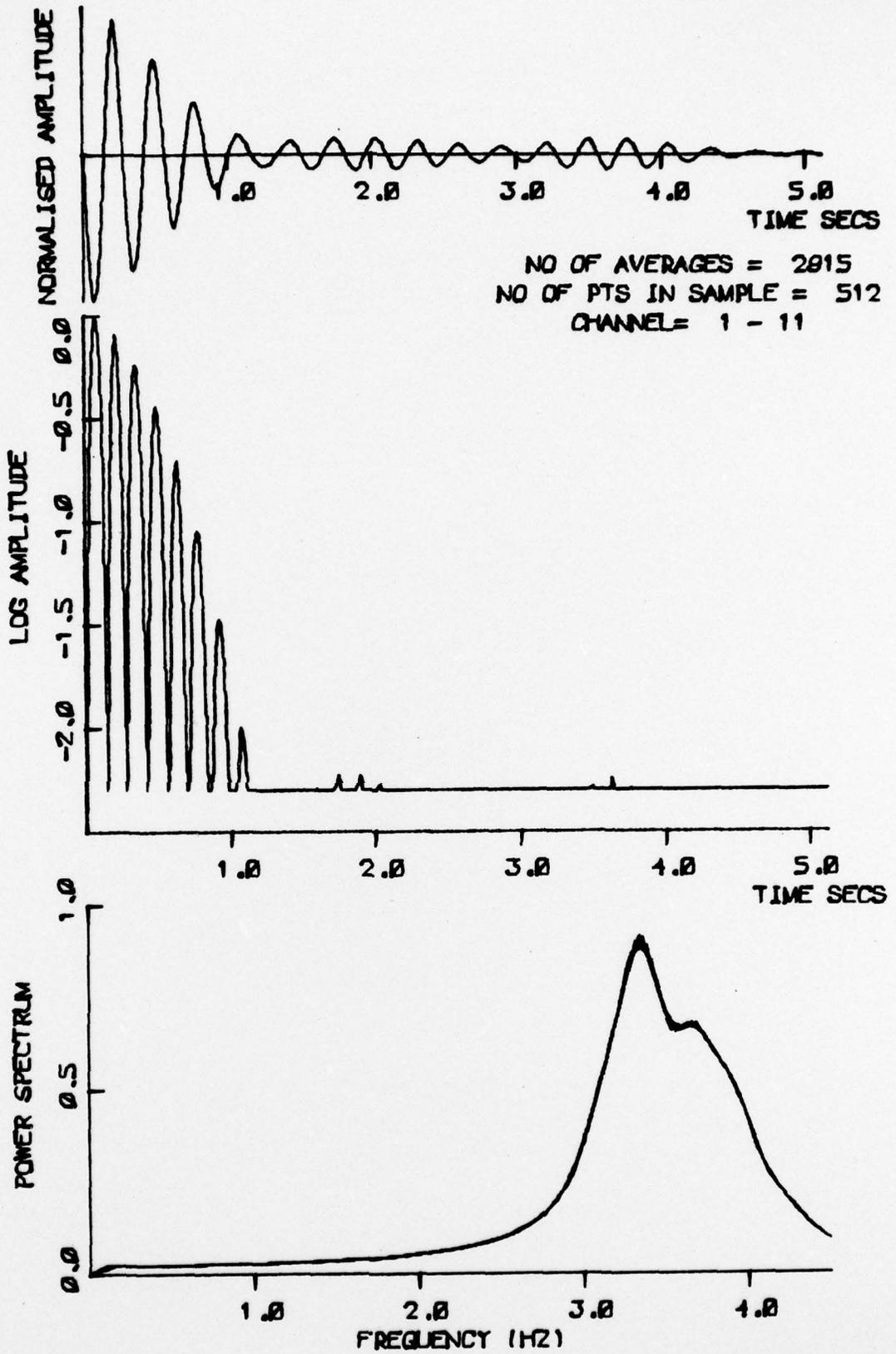
FIG. 12 RANDOM DECREMENT ANALYSIS (absorber correctly tuned)
