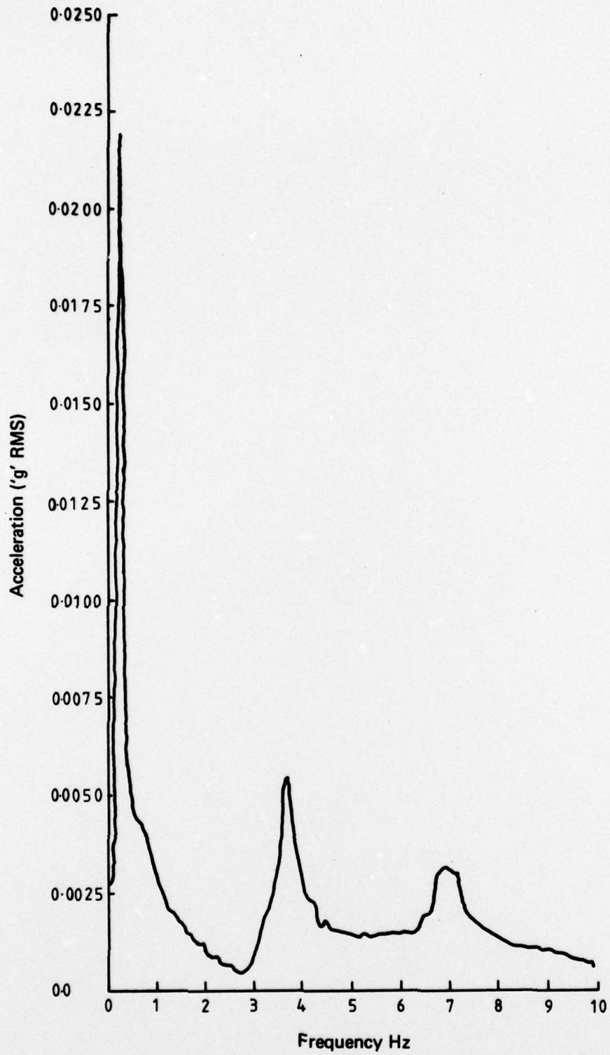
FIG. 18 FREQUENCY SPECTRUM OF RESPONSE (absorber detuned 10 p.s.i.)
