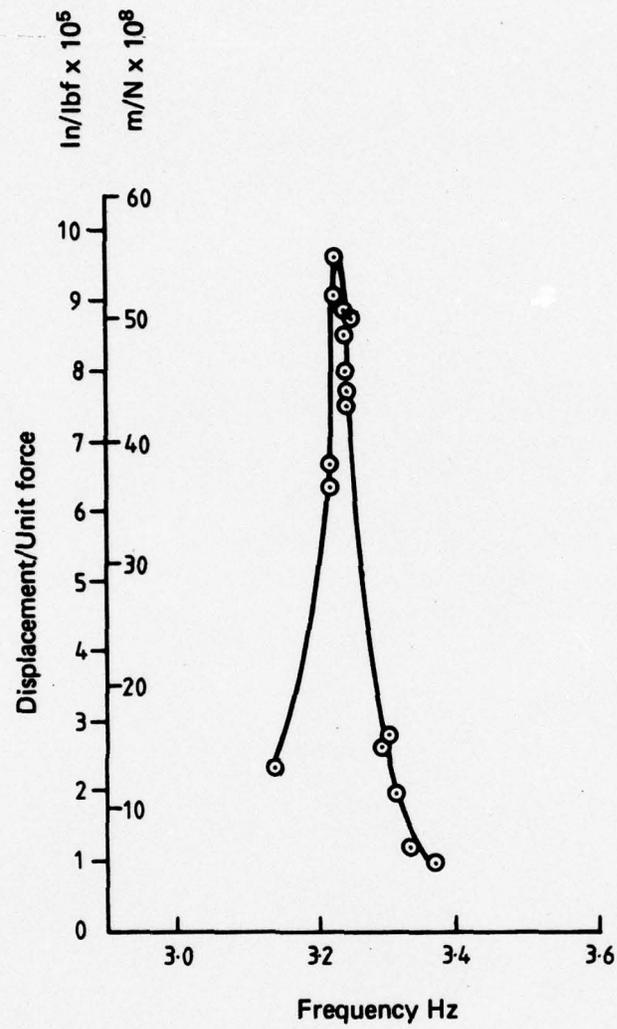
FIG. 3 VARIATION OF SHIP RESPONSE WITH FREQUENCY
