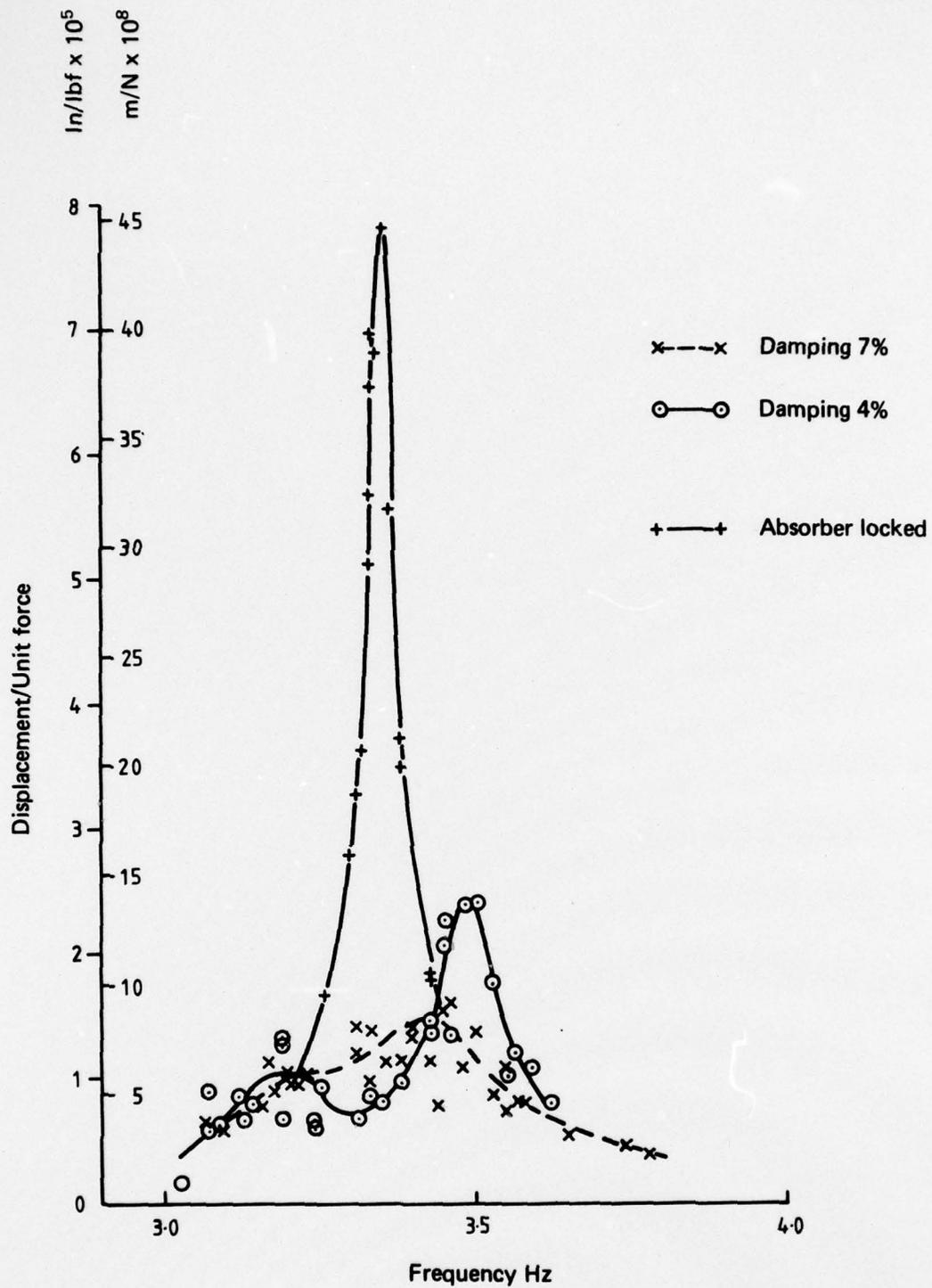
FIG. 9 EFFECT OF ABSORBER DAMPING ON SHIP RESPONSE
