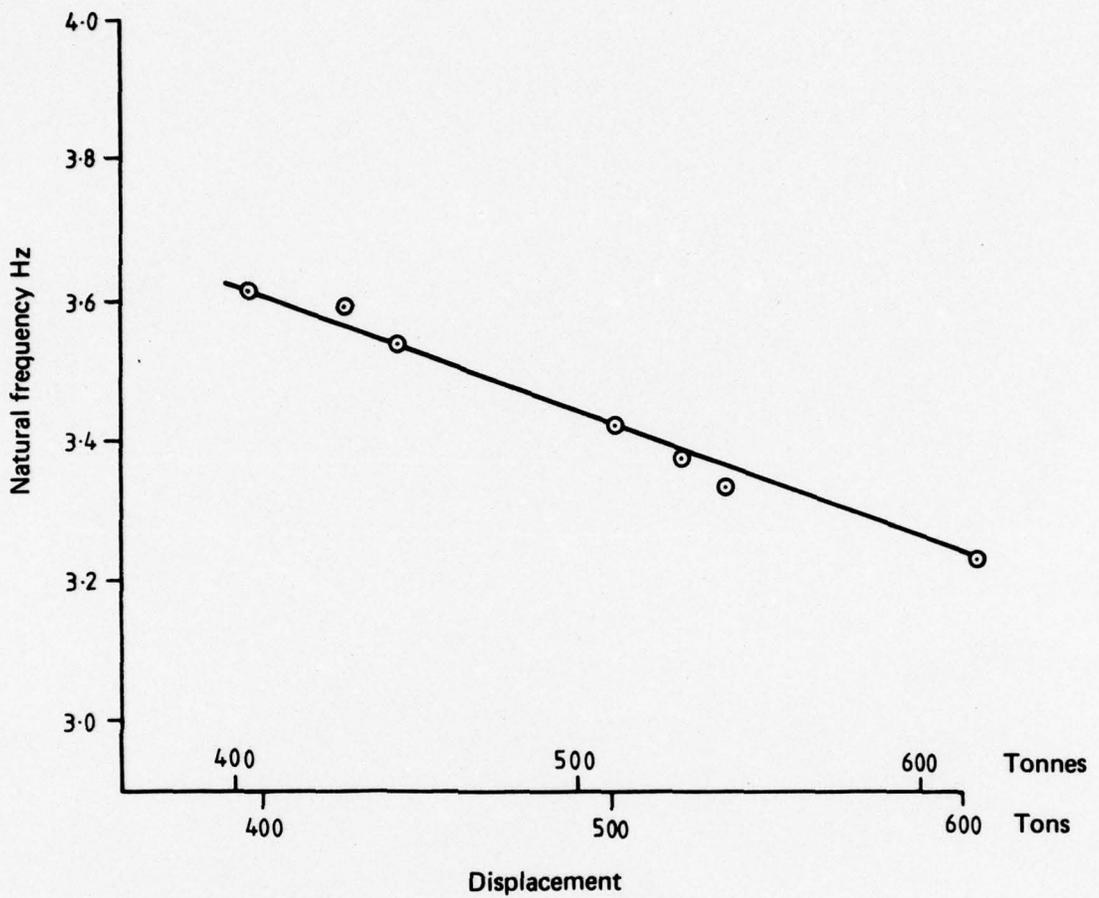
FIG. 4 VARIATION OF SHIP NATURAL FREQUENCY WITH DISPLACEMENT
