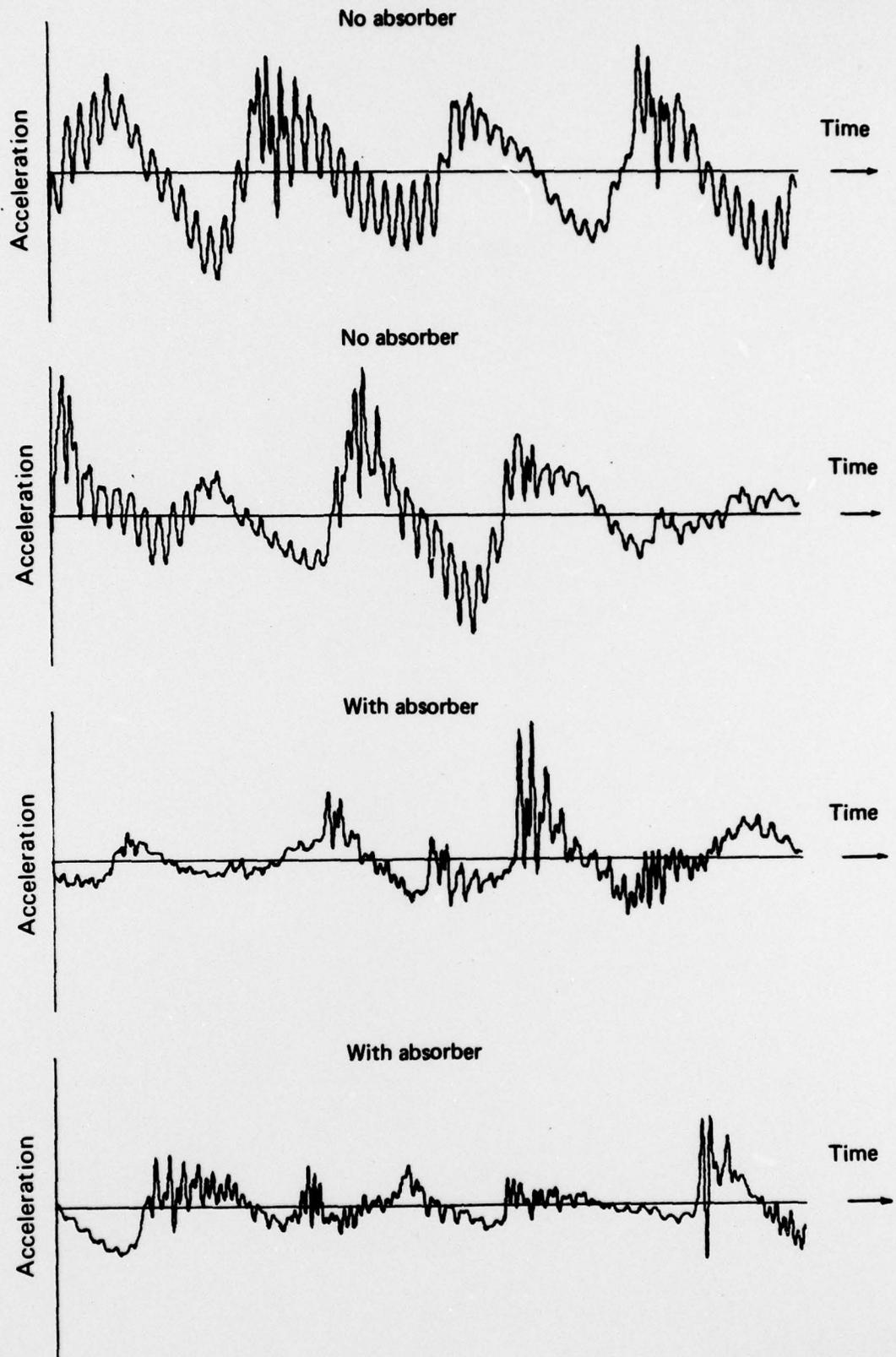
FIG. 15 COMPARISON OF SHIP RESPONSE WITH AND WITHOUT ABSORBER
