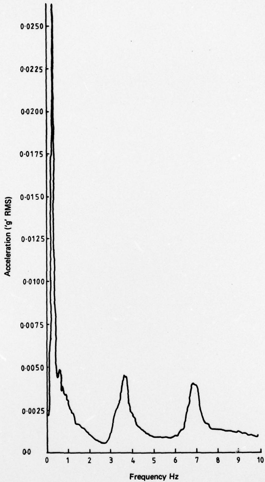
FIG. 19 FREQUENCY SPECTRUM OF RESPONSE (absorber detuned 20 p.s.i.)
