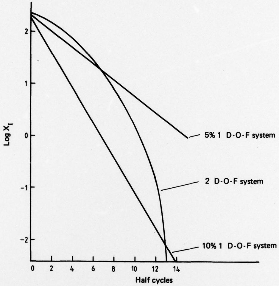
FIG. 21 COMPARISON OF ENERGY ABSORBED IN THREE SYSTEMS
