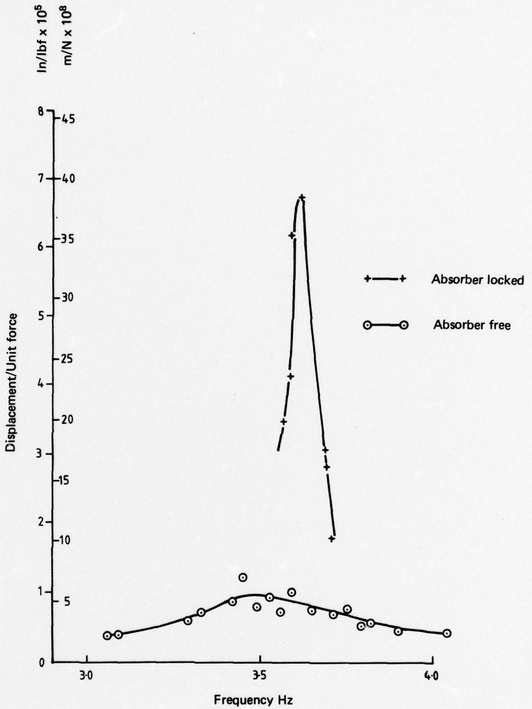
FIG. 7 EFFECT OF ABSORBER ON SHIP RESPONSE
