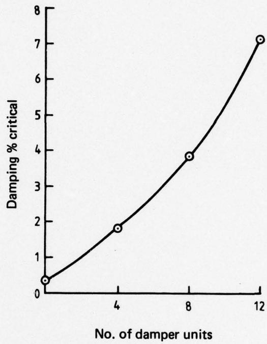
FIG. 6 VARIATION OF ABSORBER DAMPING WITH NUMBER OF DAMPERS
