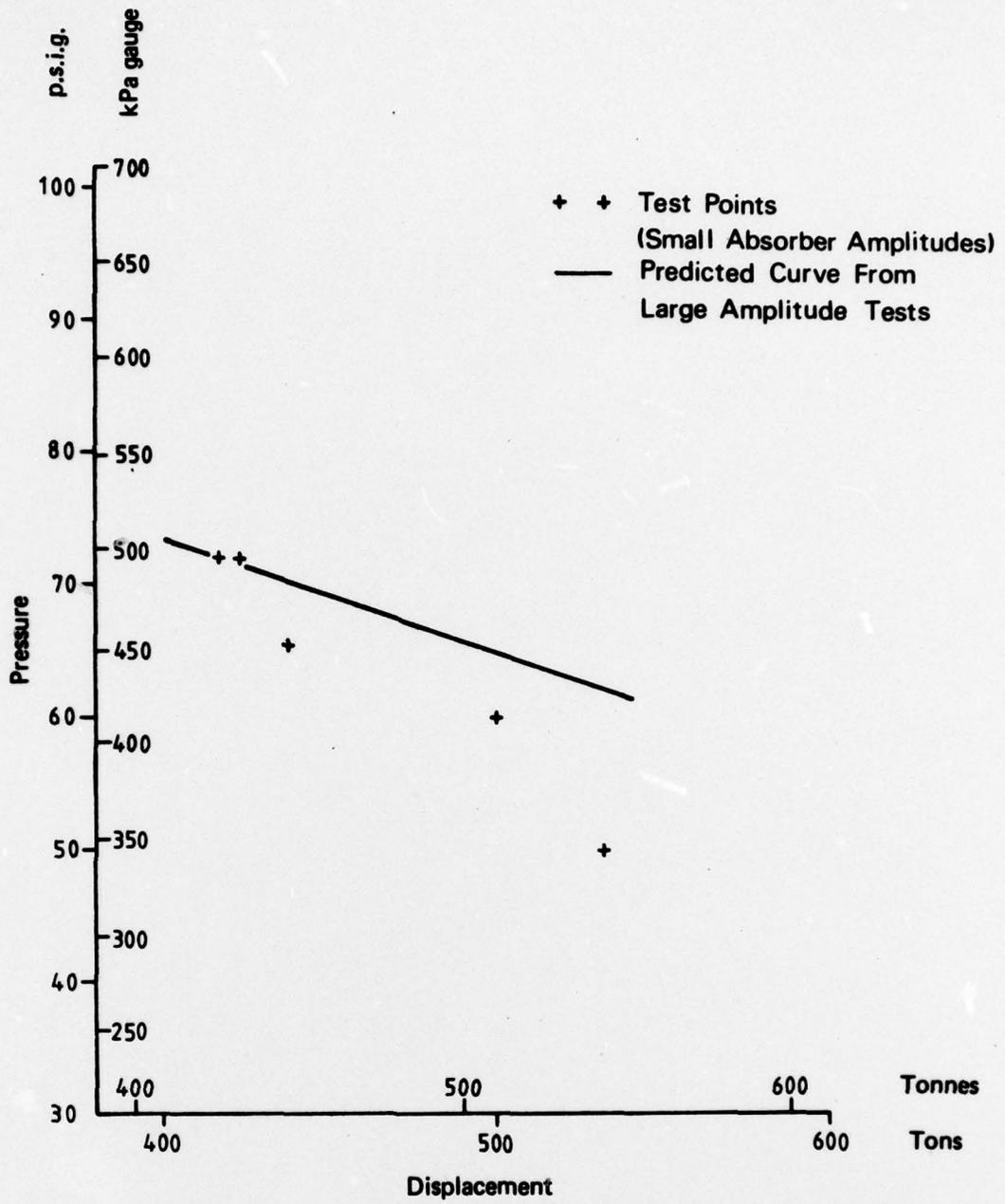
FIG. 10 RECOMMENDED AIR SPRING PRESSURE VERSUS SHIP DISPLACEMENT
