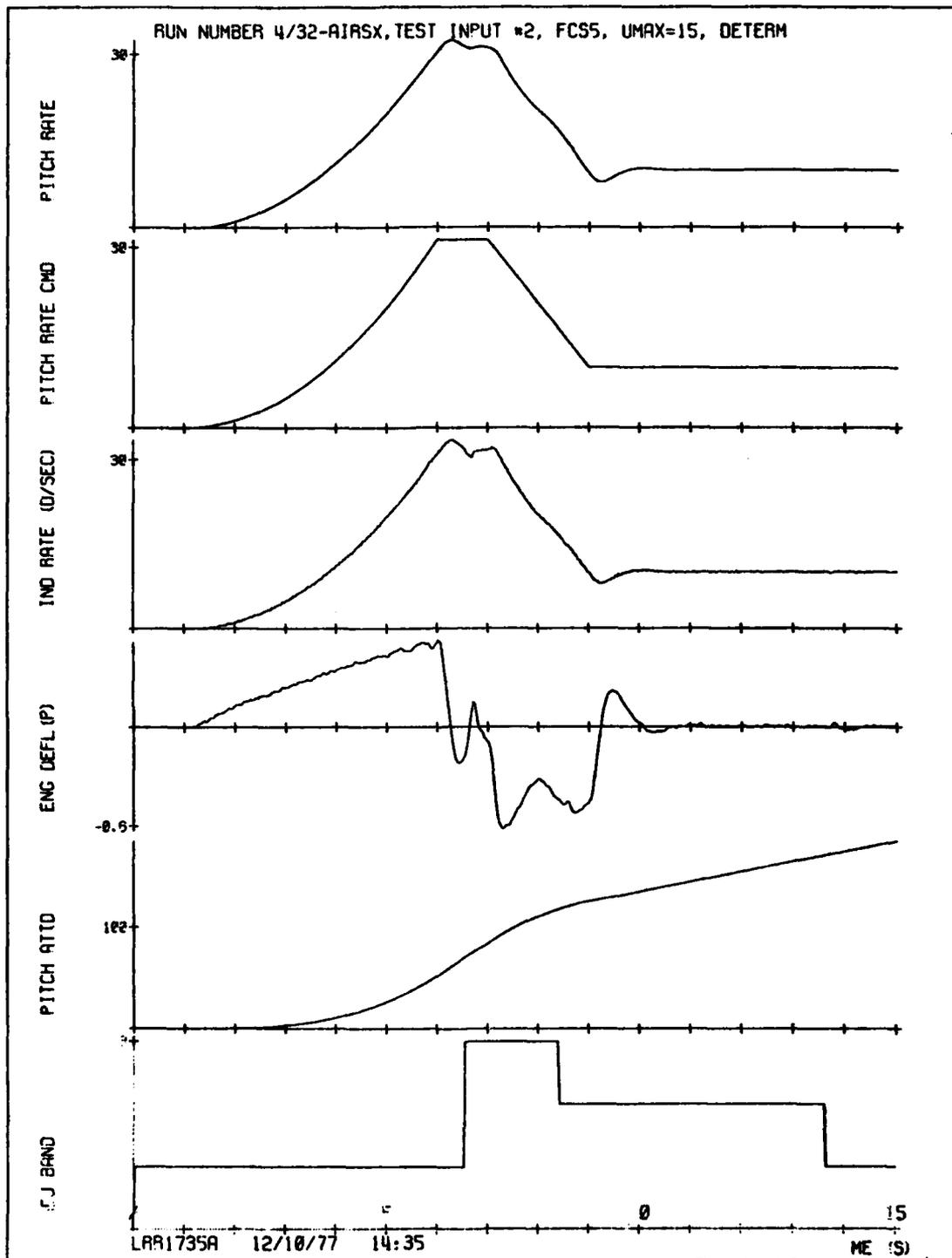
Figure 53. AIRSX attitude feedback with deterministic errors, UMAX = 15.
