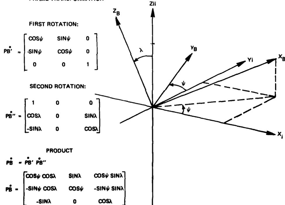
Figure B-1. Body frame to inertial frame transformation.
