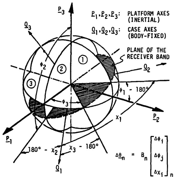
Figure 36. Definition of the AIRS band angles and body-angle increment relationship.
