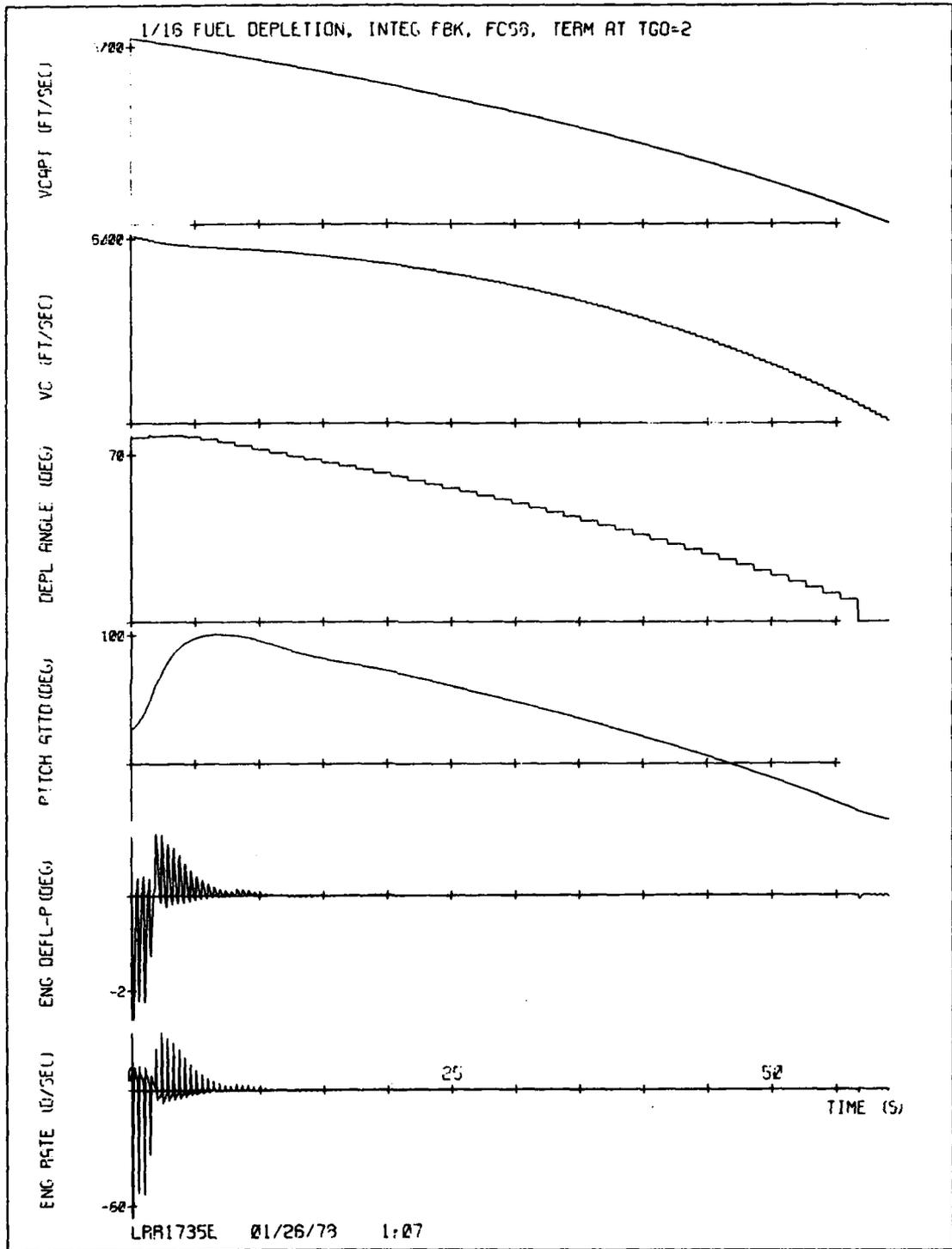
Figure 76-2. STEER, fuel depletion steering, 8 rad/sec autopilot, integral feedback,  $T_{PR} = 2$ .
