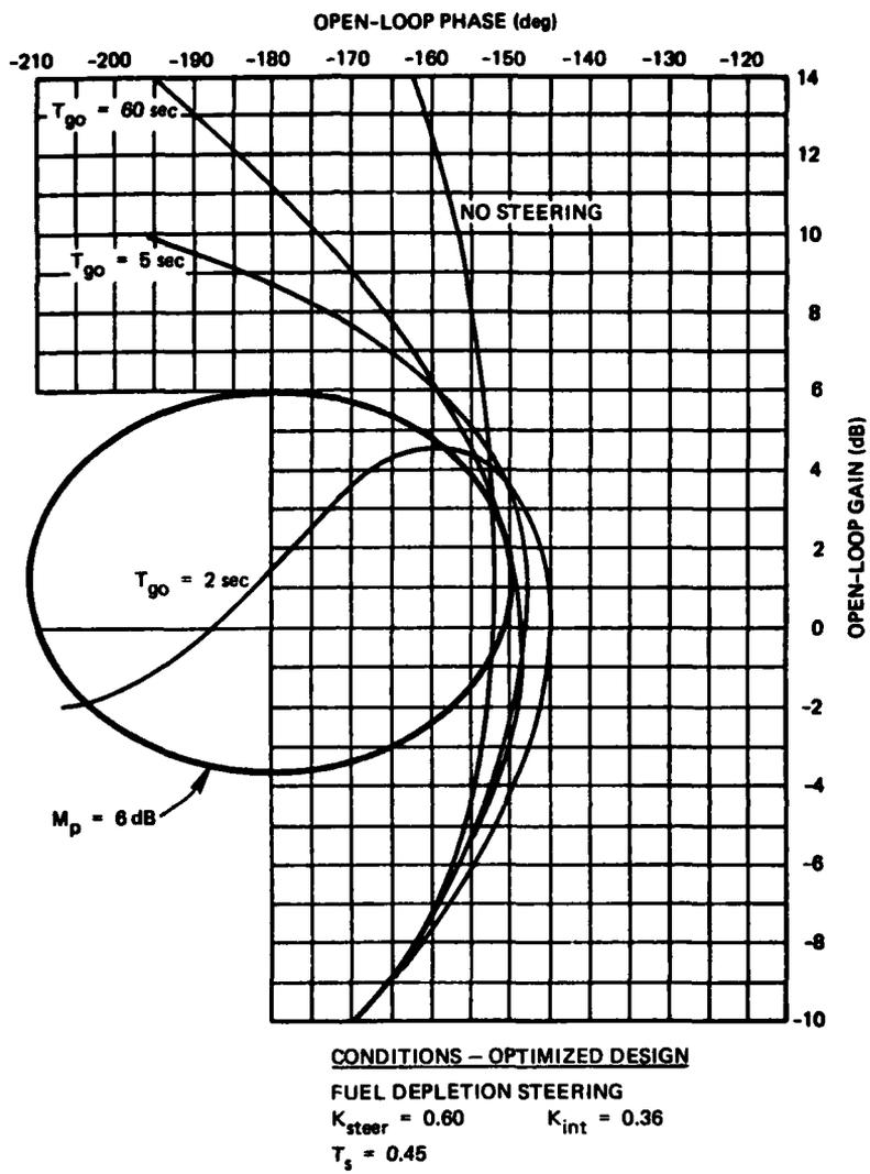
Figure 32. Effect of  $T_{go}$ , STEER02.
