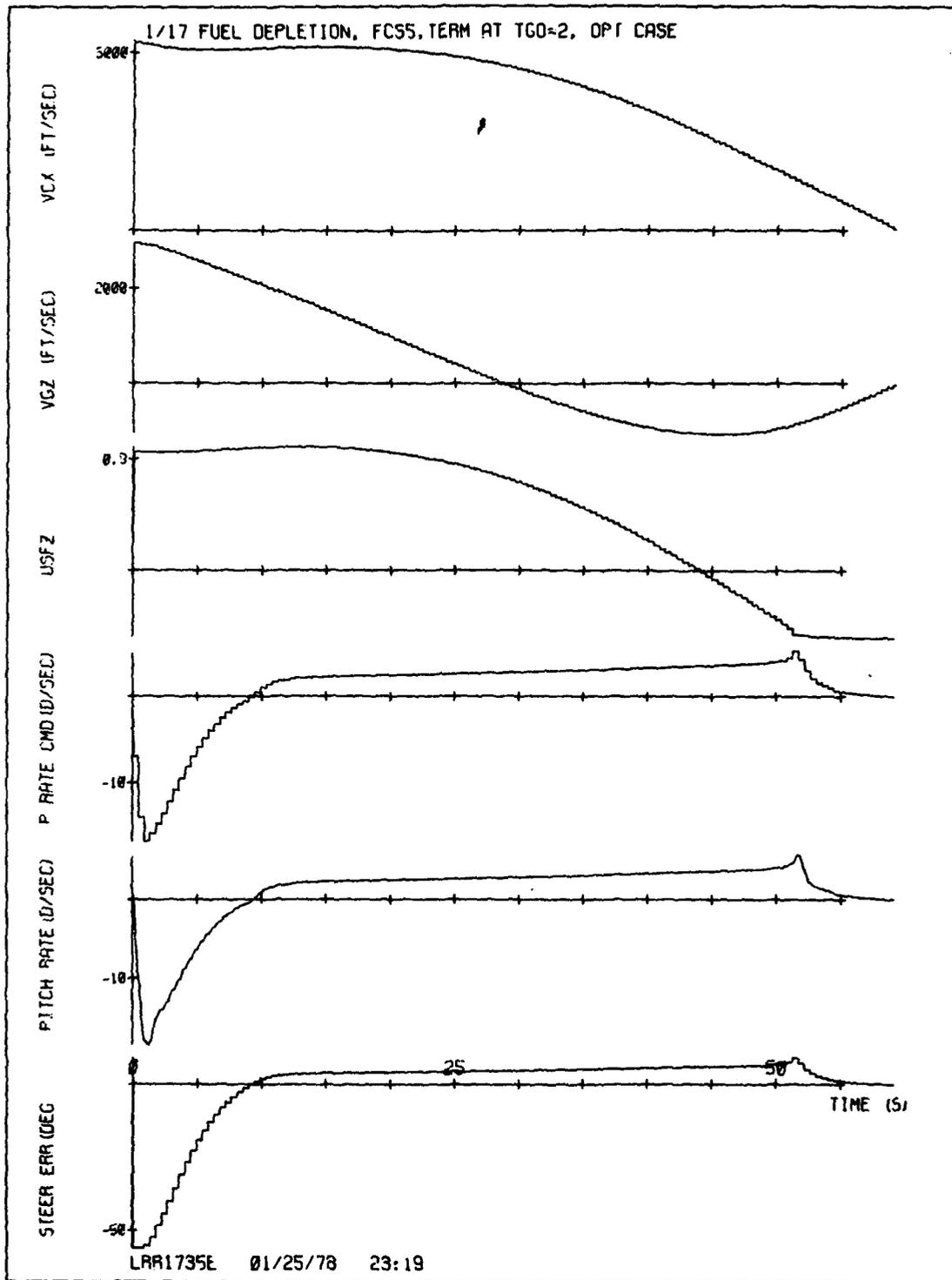
Figure 77-1. STEER, fuel depletion steering, optimized design,  $T_{FR} = 2$ .
