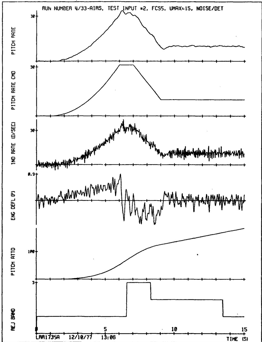
Figure 54. AIRS attitude feedback with random noise and deterministic errors, UMAX = 15. 105
