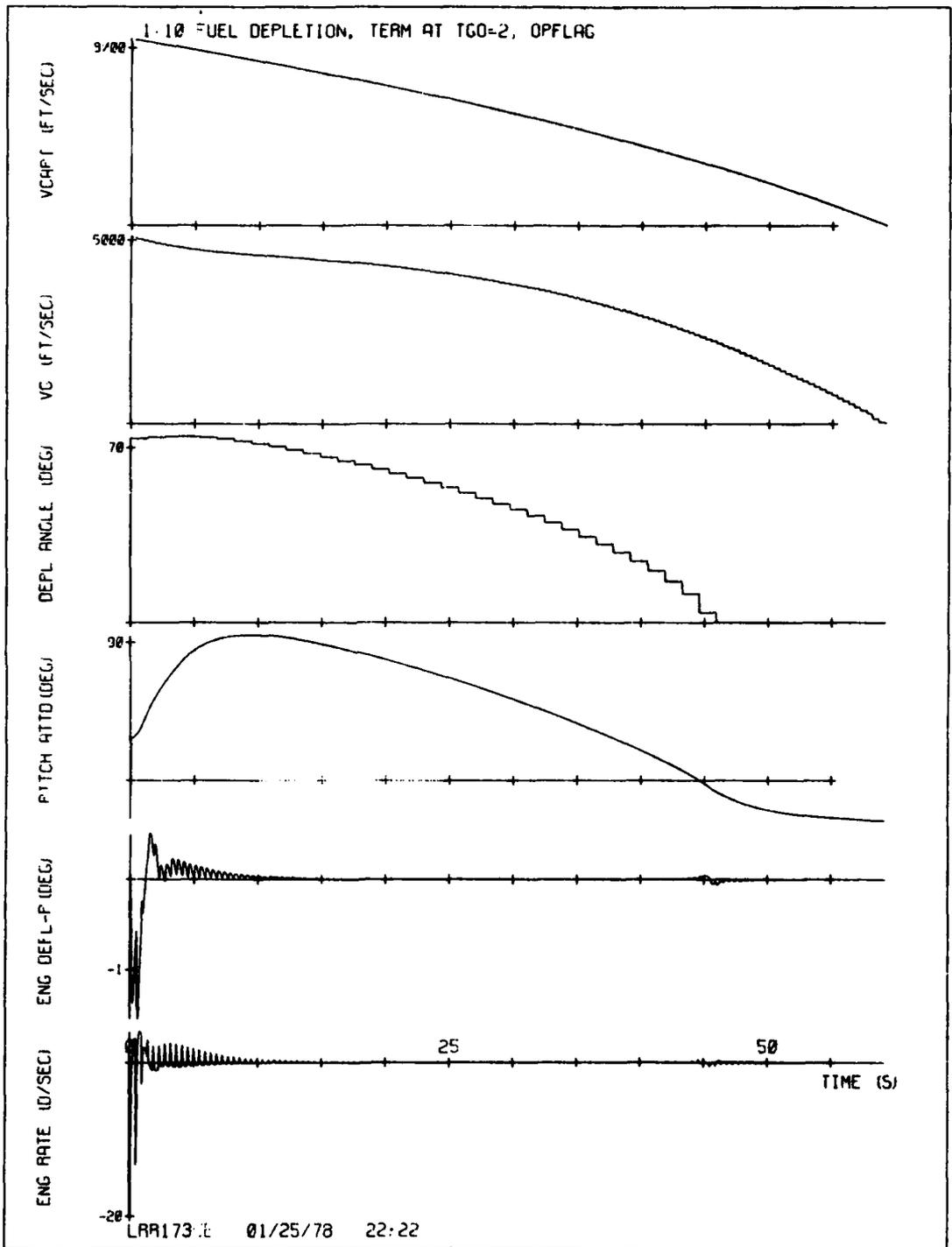
Figure 70-2. STEER, fuel depletion steering,  $T_{FR} = 2$ , simplified  $\theta$  calculation.
