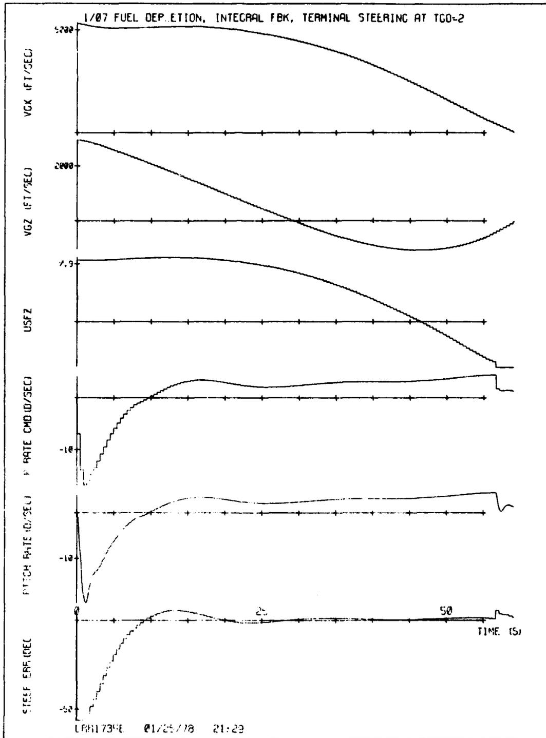
Figure 67-1. STEER, fuel depletion steering, integral feedback,  $T_{FR} = 2$ .
