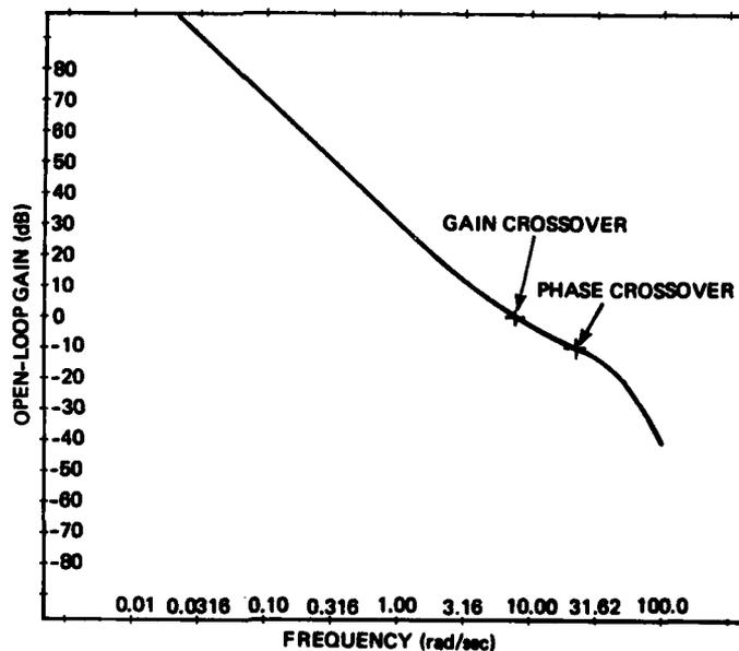
Figure 20. Gain vs frequency -  $\omega_{x0} = 8$  rad/sec.
