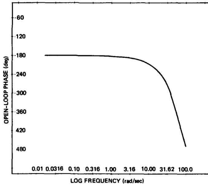
Figure 12. Phase vs frequency - uncompensated system.
