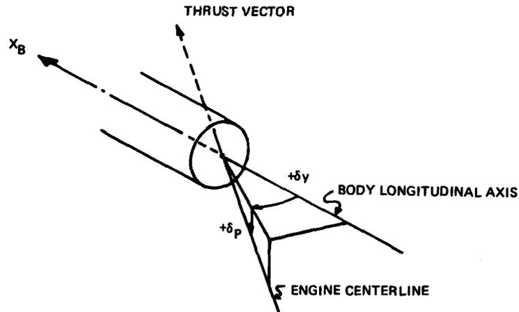
The direction of the thrust vector is referenced to the vehicle body axes using the  $\bar{E}NG$  vector where
