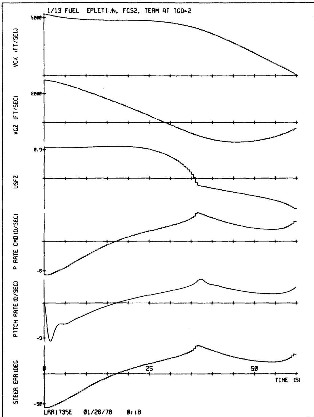
Figure 73-1. STEER, fuel depletion steering, 2 rad/sec autopilot,  $T_{FR} = 2$ .
