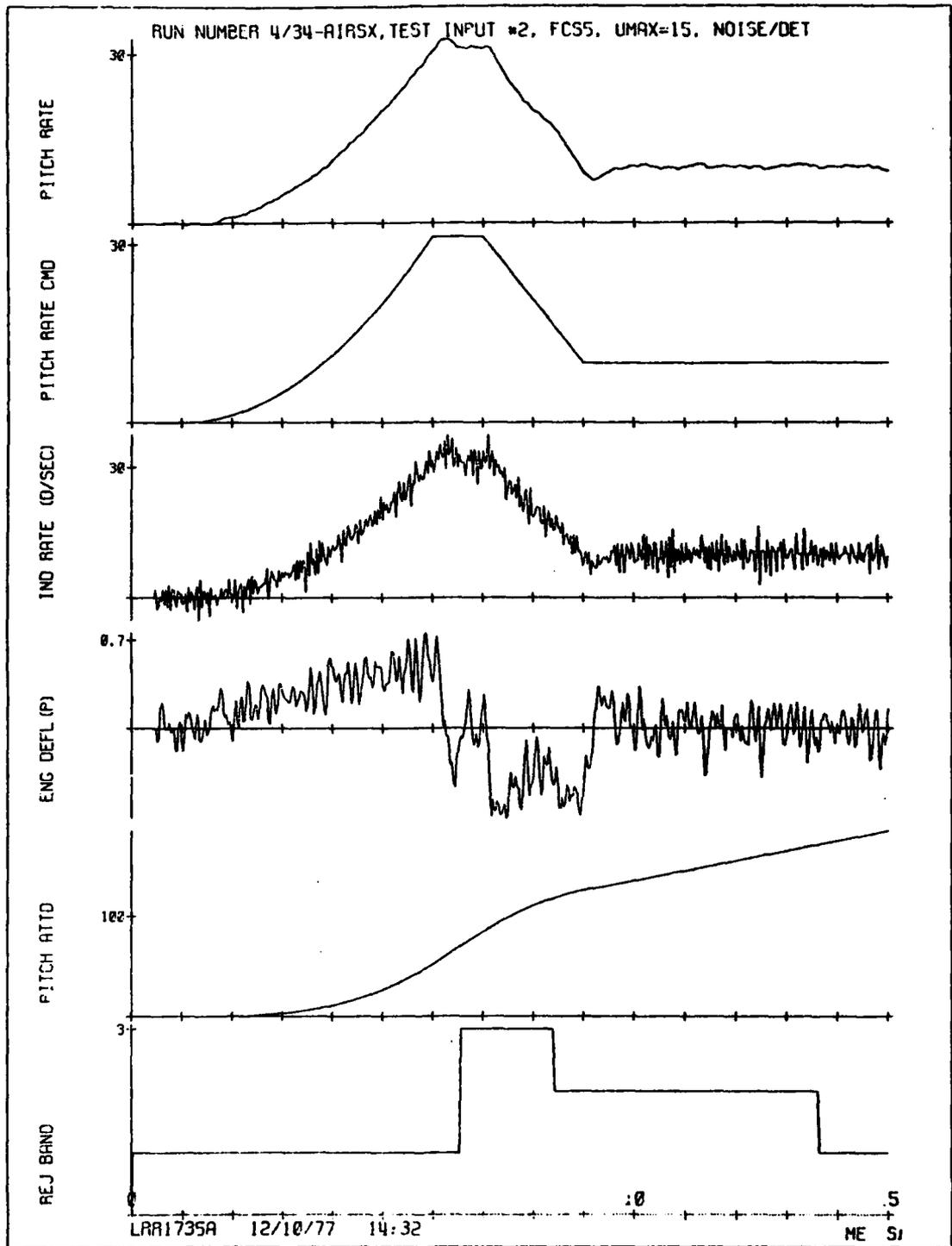
Figure 55. AIRSX attitude feedback with random noise and deterministic errors, UMAX = 15.
