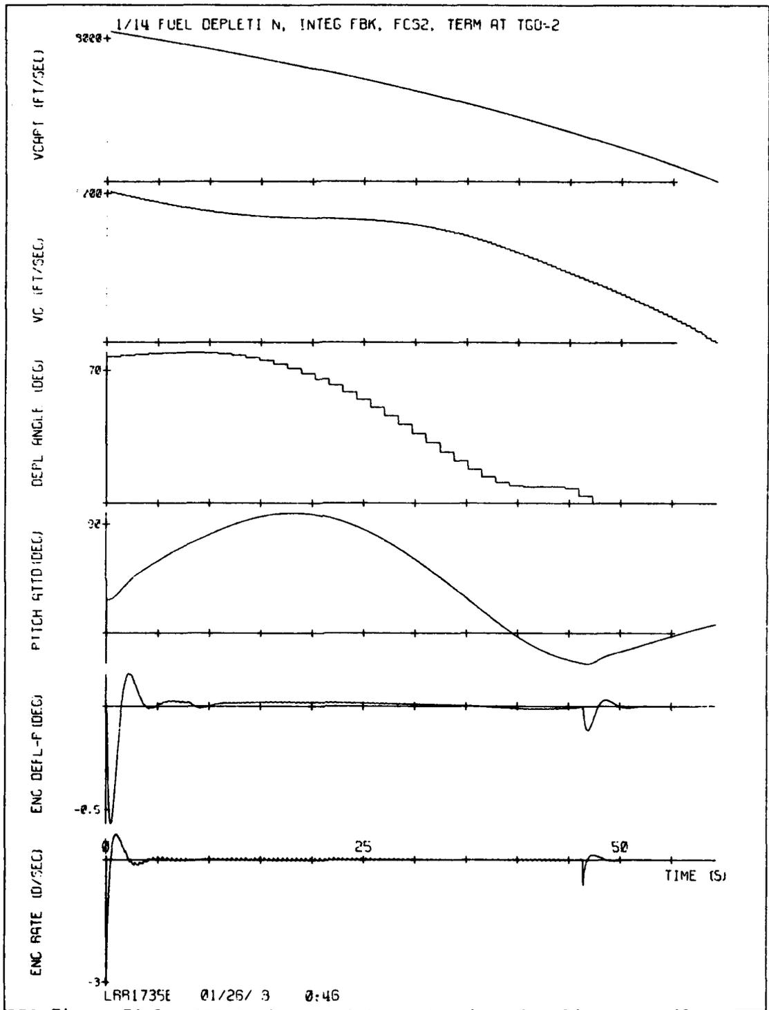
Figure 74-2. STEER, fuel depletion steering, 2 rad/sec autopilot, integral feedback,  $T_{FR} = 2$ .
