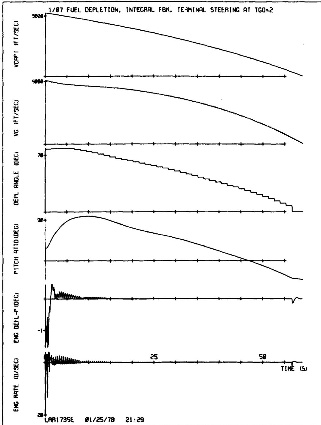
Figure 67-2. STEER, fuel depletion steering, integral feedback,  $T_{FR} = 2$ .
