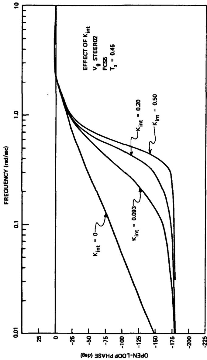
Figure 25. Effect of  $K_{int}$ , phase vs frequency.
