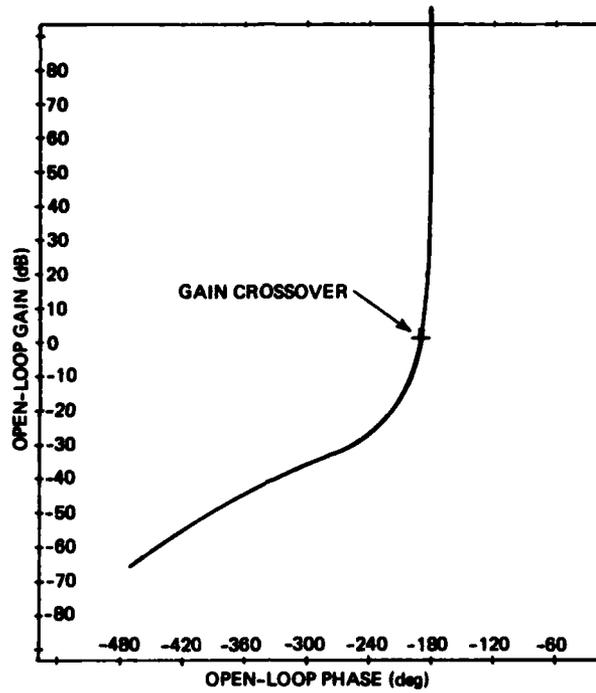
Figure 13. Gain vs phase - uncompensated system.
