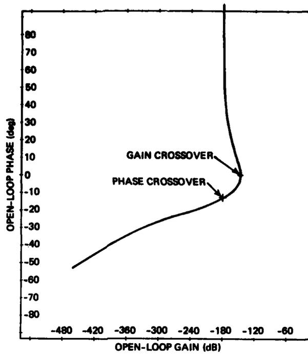
Figure 19. Gain vs phase -  $\omega_{x0} = 5$  rad/sec.
