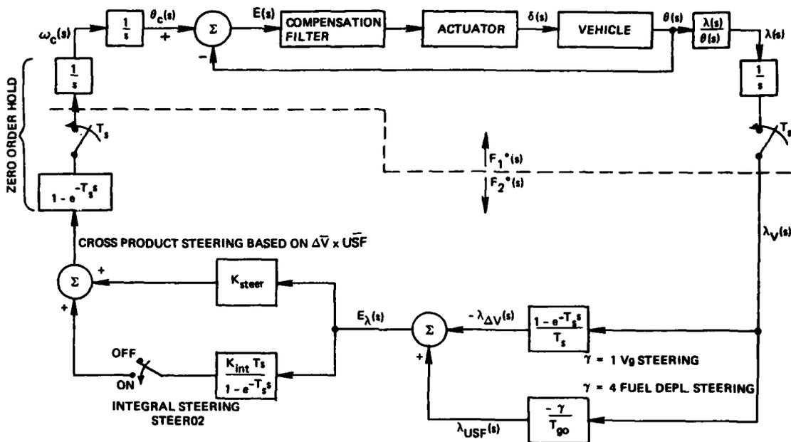
Figure 5. Autopilot and steering loop analytical model.
