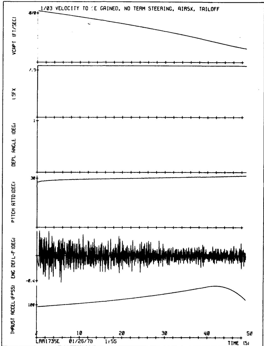
Figure 63-2. STEER,  $V_g$  steering with AIRSX and thrust tailoff.
