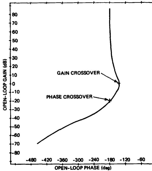
Figure 16. Gain vs phase -  $\omega_{XO} = 2$  rad/sec.
