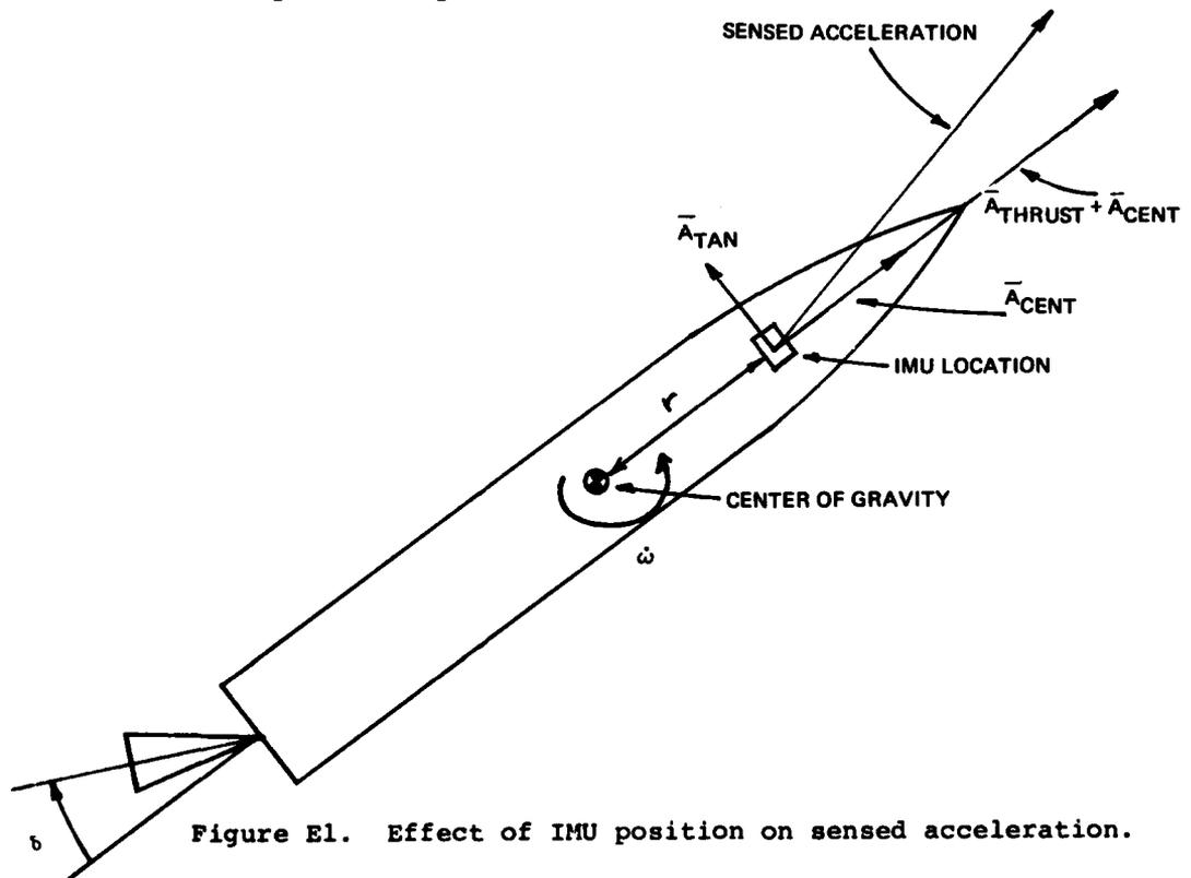
Figure E1. Effect of IMU position on sensed acceleration.
