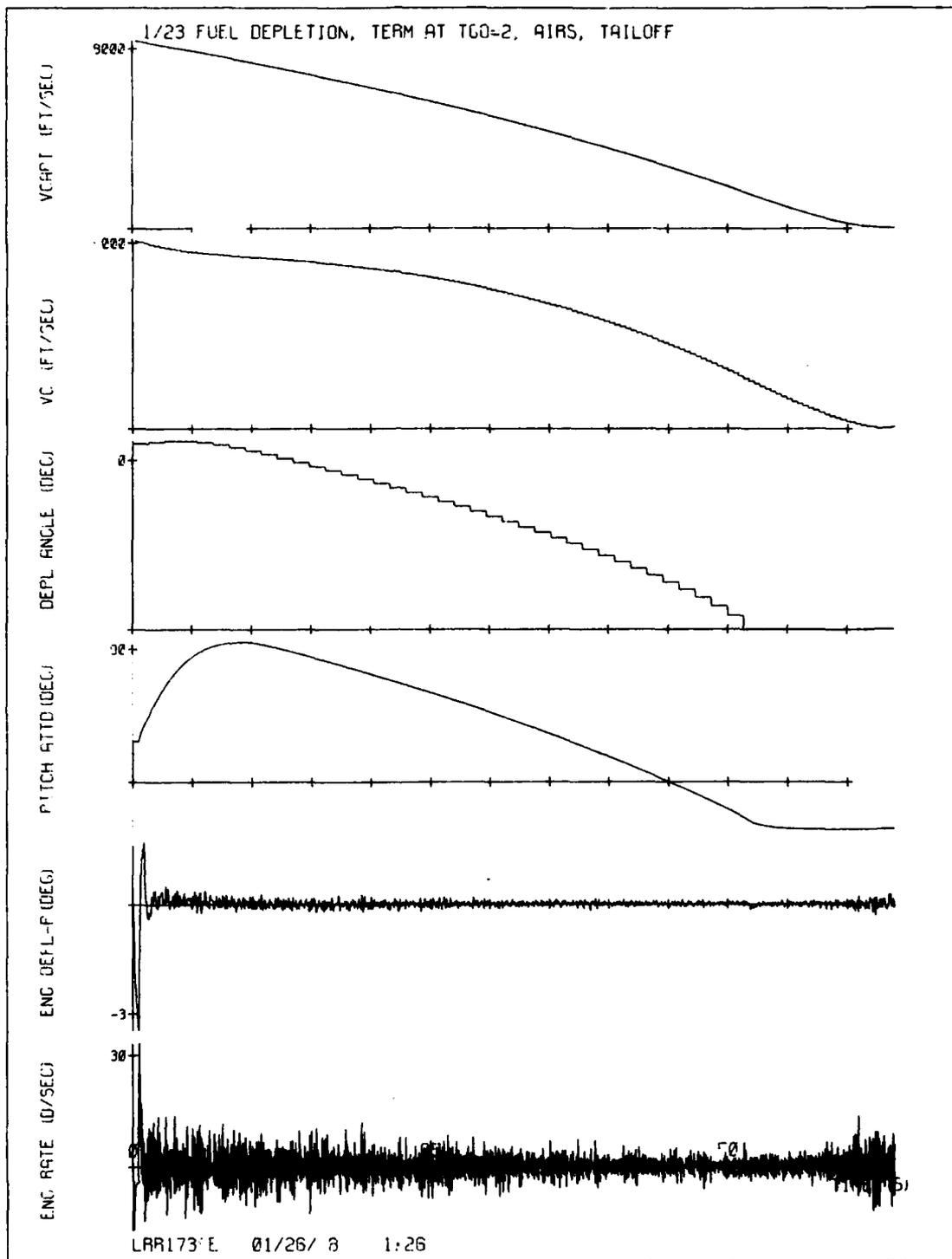
Figure 83-2. STEER, fuel depletion steering, optimized design, AIRSX, thrust tailoff,  $T_{FR} = 2$ . 163
