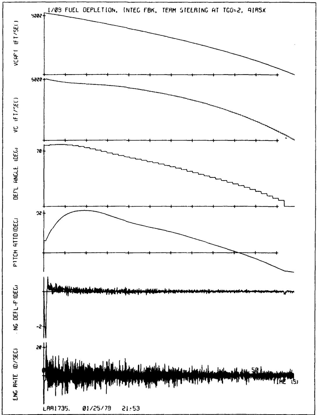
Figure 68-2. STEER, fuel depletion steering, integral feedback,  $T_{FR} = 2$ , AIRSX.
