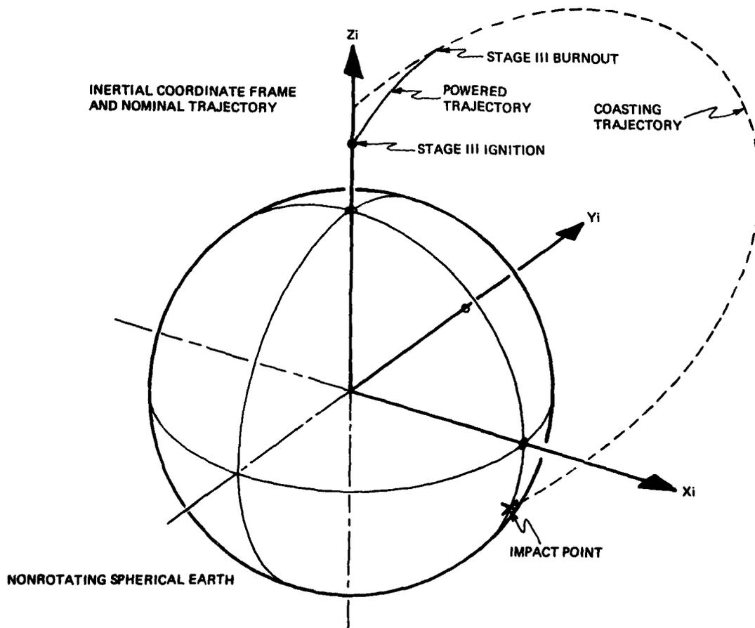
Figure 3. Inertial coordinate frame and nominal trajectory.
