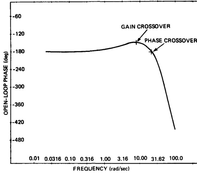
Figure 21. Phase vs frequency -  $\omega_{x0} = 8$  rad/sec.
