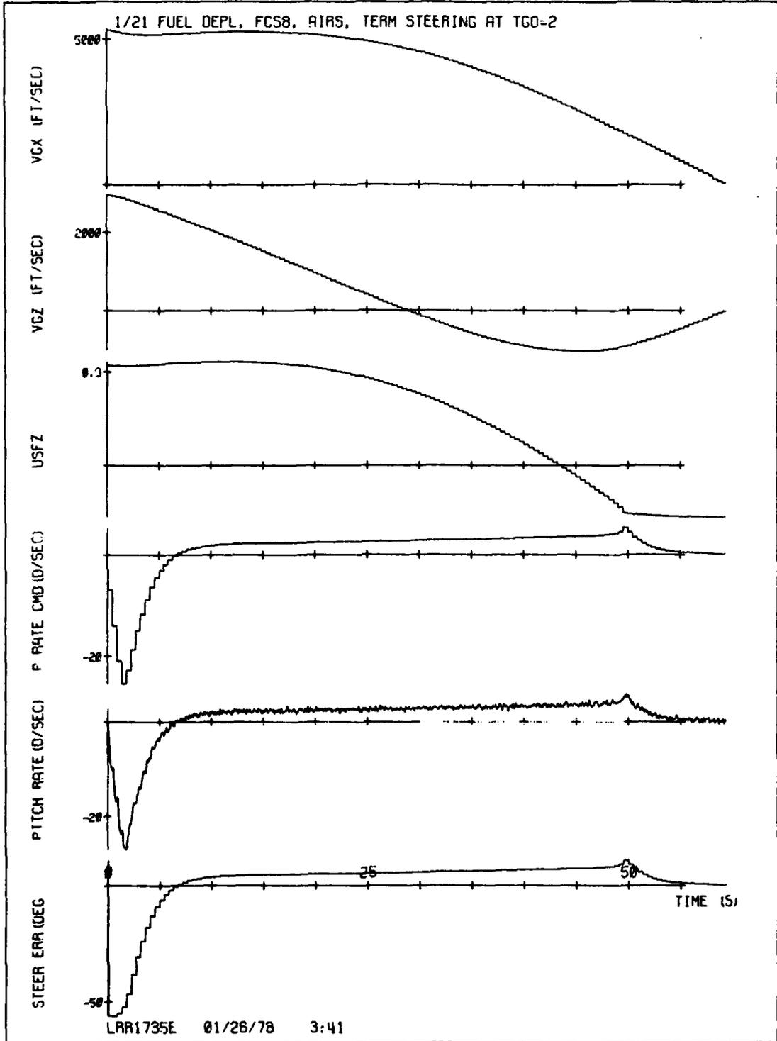
Figure 81-1. STEER, fuel depletion steering, 8 rad/sec autopilot, AIRS,
