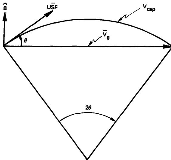
Figure 4. Geometry of the fuel depletion arc.
