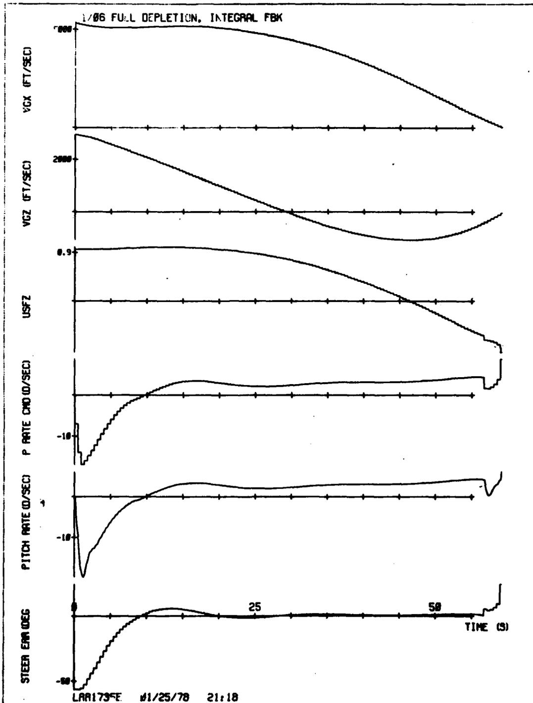
Figure 66-1. STEER, fuel depletion steering, integral feedback.
