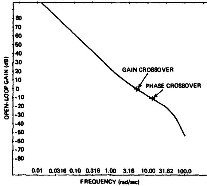
Figure 17. Gain vs frequency -  $\omega_{x0} = 5$  rad/sec.
