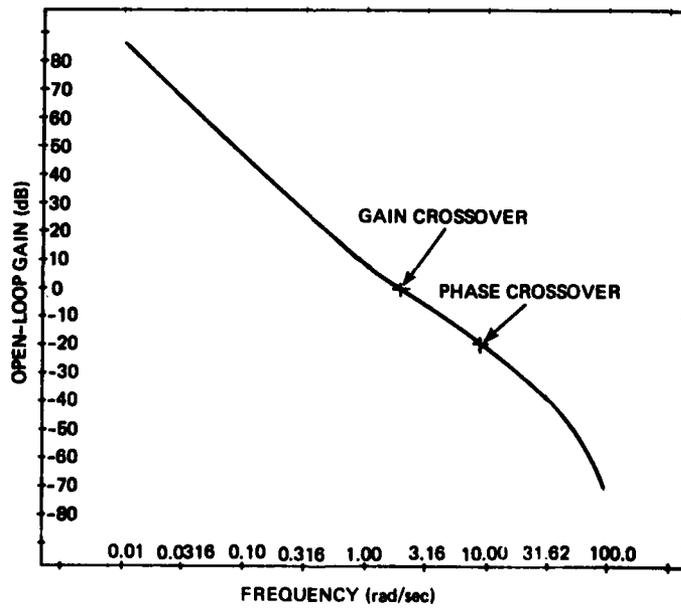
Figure 14. Gain vs frequency -  $\omega_{x0} = 2$  rad/sec.
