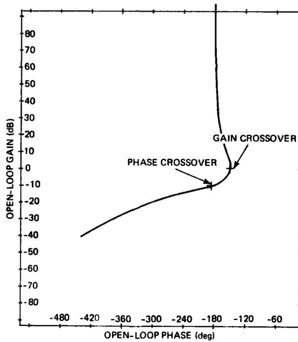
Figure 22. Gain vs phase -  $\omega_{x0} = 8$  rad/sec.
