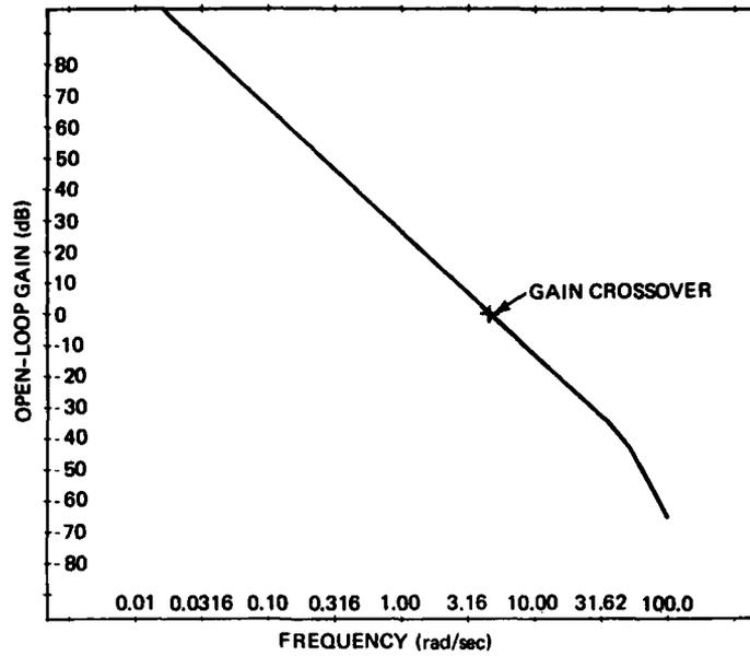
Figure 11. Gain vs frequency - uncompensated system.
