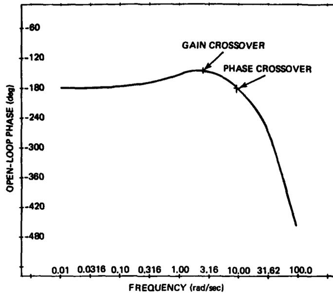
Figure 15. Phase vs frequency -  $\omega_{XO} = 2$  rad/sec.
