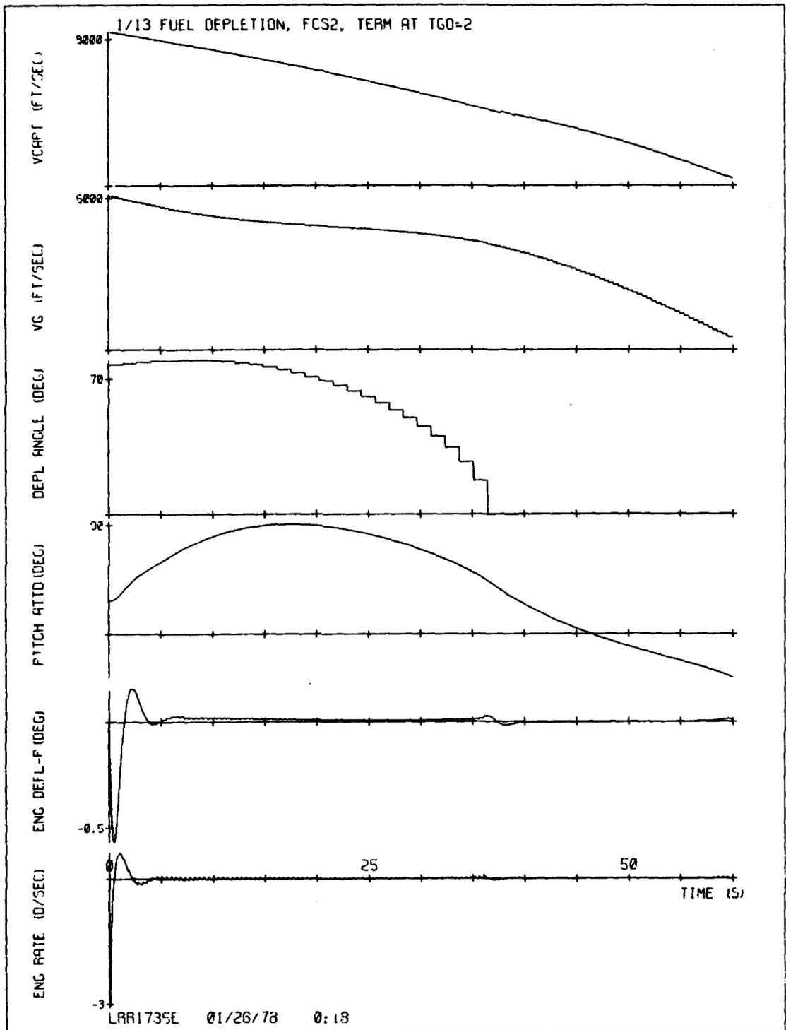
Figure 73-2. STEER, fuel depletion steering, 2 rad/sec autopilot,  $T_{FR} = 2$ .
