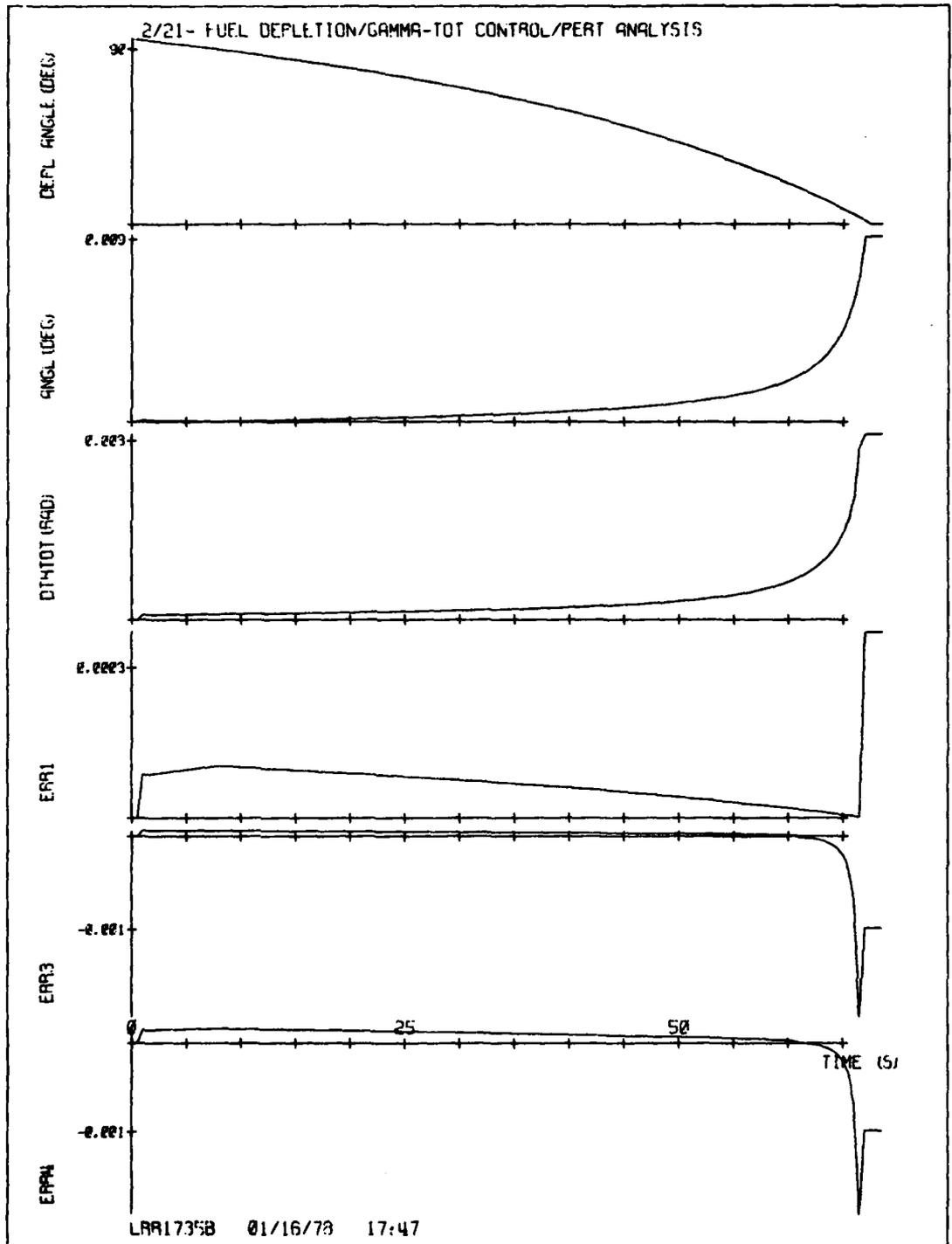
Figure 60-1. OFFSETT, fuel depletion steering with Gamma/TOT control, perturbation analysis. 115
