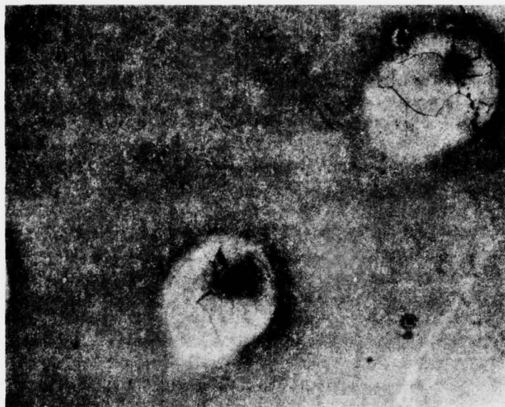
Figure 51. Examples of the type of pits analyzed by scanning Auger in Figure 7; note the etched area surrounding the pits.
