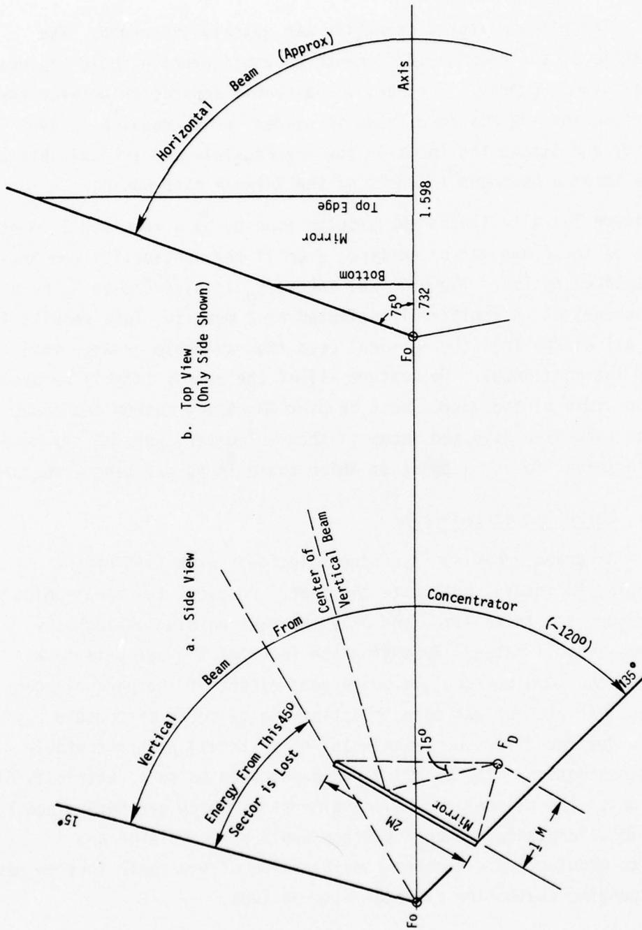
Figure 2-1. Plane Mirror Diverter
