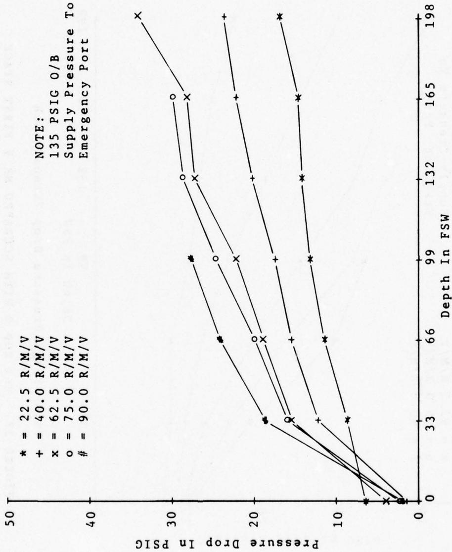
First Stage Pressure Drop Versus Depth
