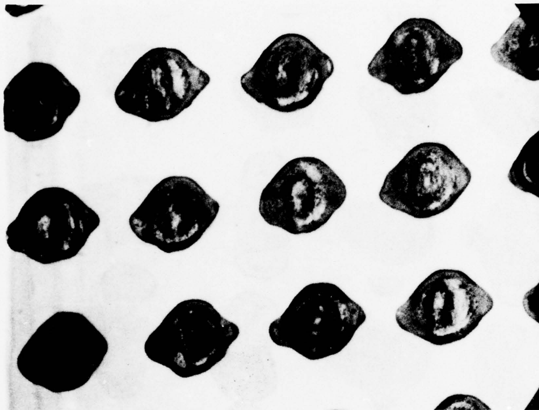
Figure 35. Photomicrograph of the Spots Formed by the Laser at the Third Power Setting. The Elliptical Shape of the Spots is Due to the Defocused State of the Laser. Two of these Spots are Profiled in Figures 39 and 40 and are Listed in Table 4 as Samples with Suffix B. Spot Spacing is 100 \mu m
