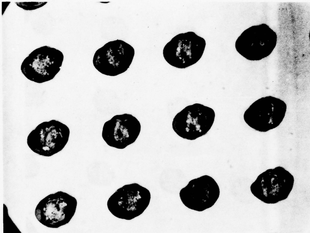
Figure 34. Photomicrograph of the Spots Formed by the Laser at the Second Lowest Power Setting. These Spots were not Profiled but the Sample was Used to Profile the "matrix" (the Al-Si Profile off a Spot). The Result is Shown in Figure 41, and on Table 4. Spot Spacing is 100 \mu m
