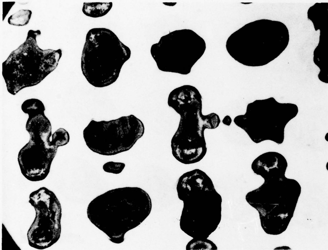
Figure 36. Photomicrograph of the Spots Formed by the Laser at the Highest Power Setting. The Laser Operation is Somewhat Unstable at this Setting as is Evident from the Surface Pattern. Two of these Spots are profiled in Figures 37 and 38 and are Listed in Table 4 as Samples with Suffix A. Spot Spacing is 100\mu\text{m}
