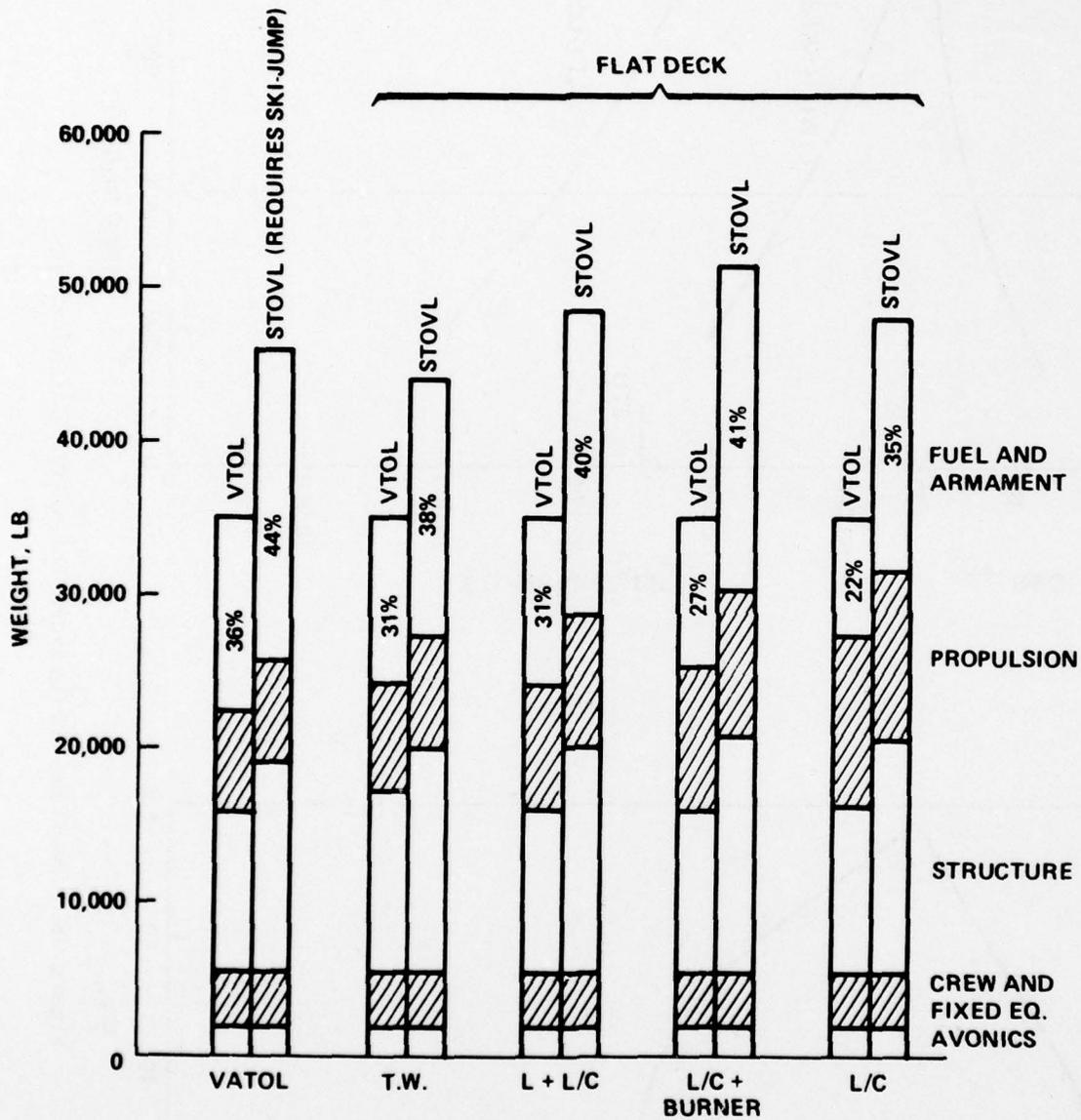
Figure 29 - Comparison of V/STOL and STOVL Weight Breakdowns
