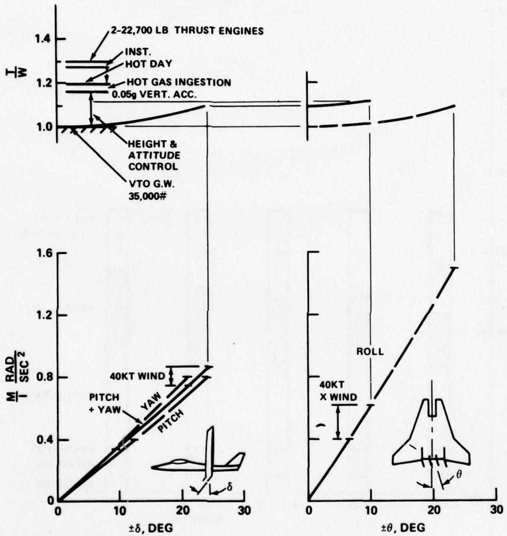
Figure 16 - Tilt Wing Thrust Vector Control
