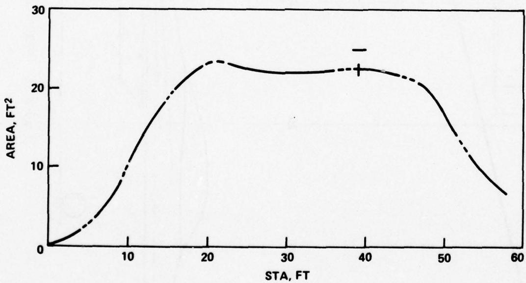
Figure 12 - VATOL Configuration Effect on Aerodynamic Lines
