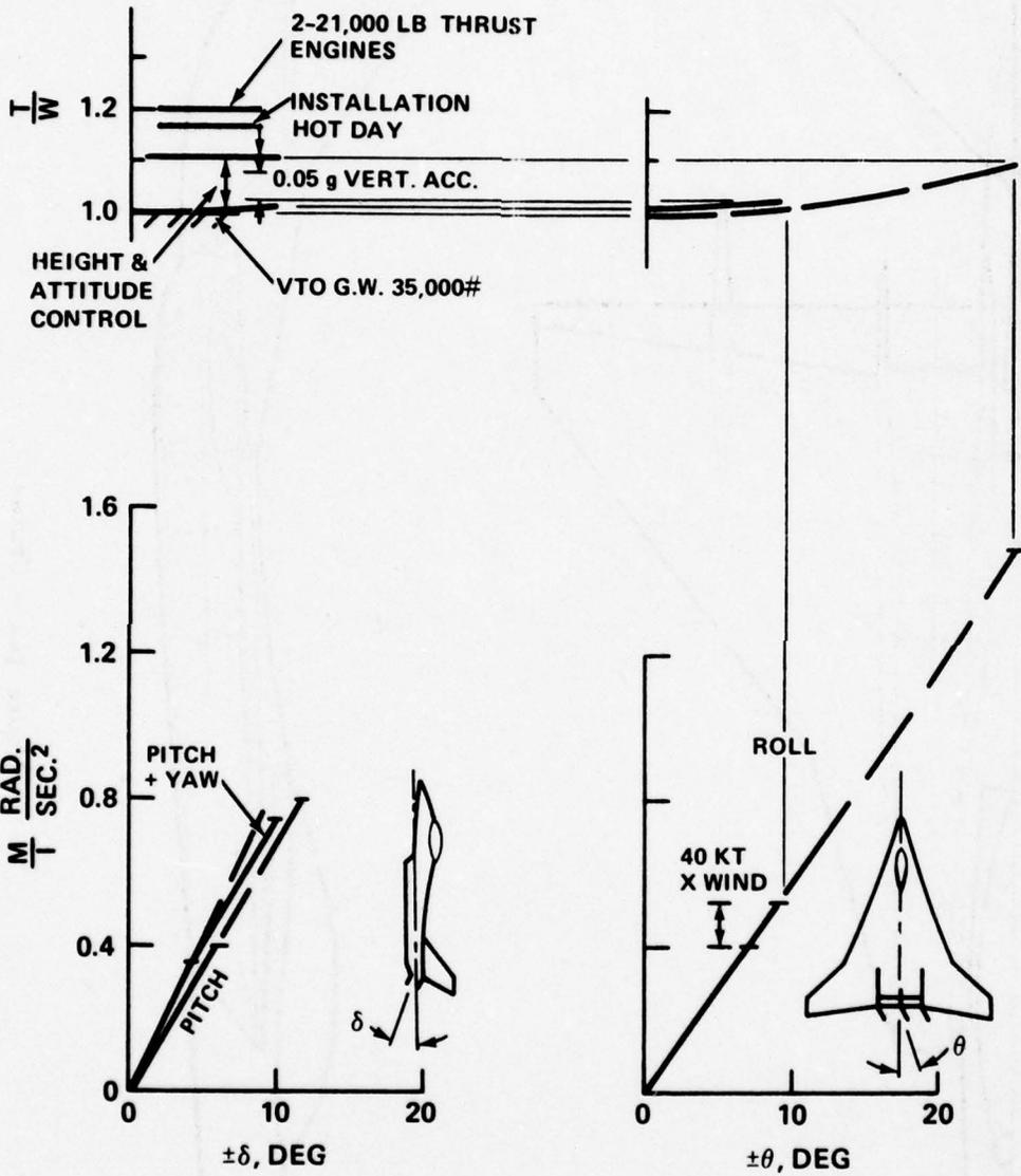
Figure 13 - VATOL Thrust Vector Control
