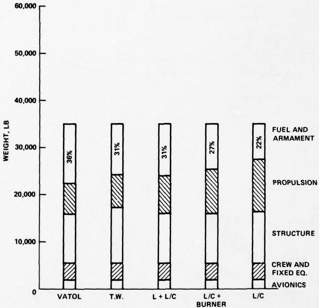
Figure 17 - Weight Breakdown of VTOL Configurations
