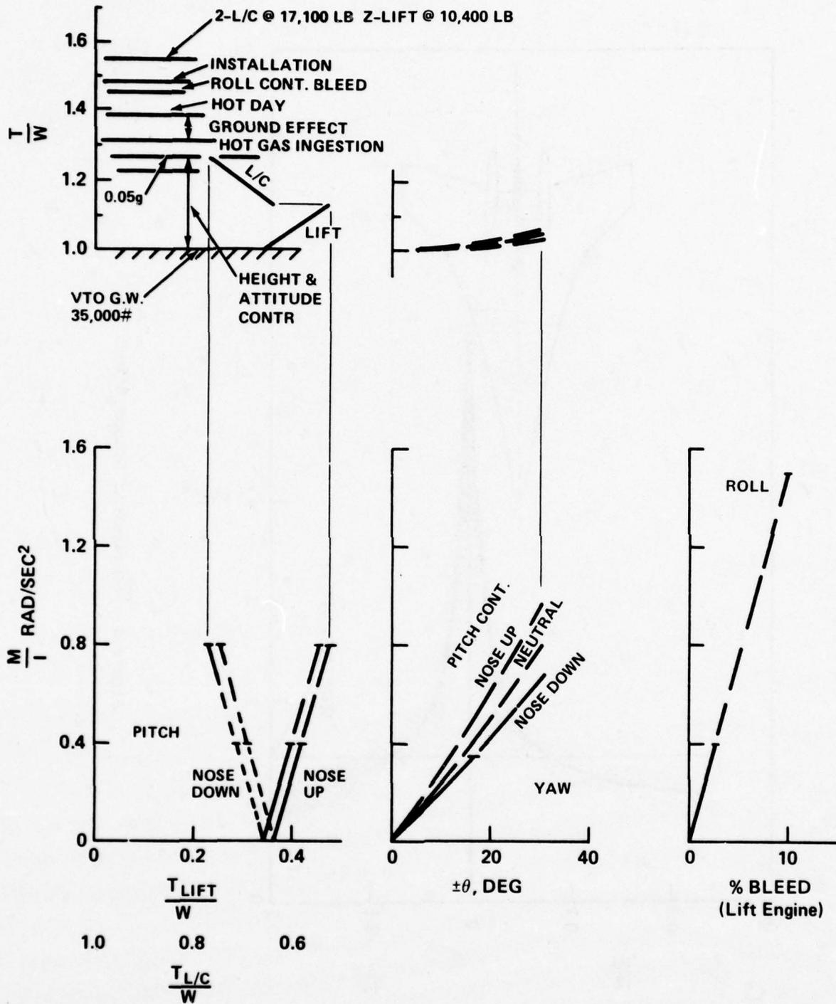
Figure 3 - Lift Plus Lift/Cruise Control and Thrust Buildup
