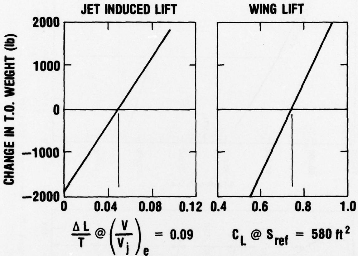
Figure 23 - STO Performance Sensitivity for Lift Cruise Plus Remote Burner Concept Sized for STO
