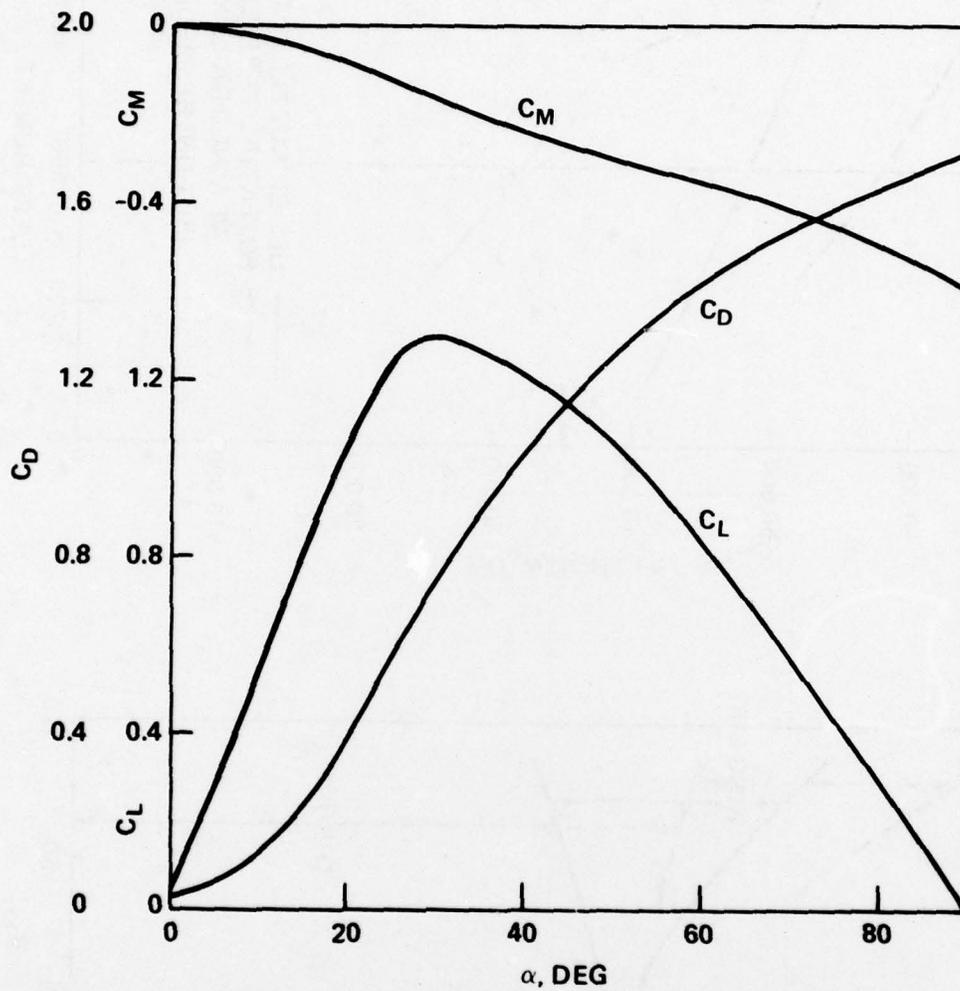
Figure 25 - Low-Speed Aerodynamic Characteristics for VATOL and Tilt Wing Configurations
