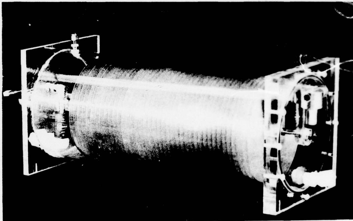
Figure 14. Photograph of gas stripper removed from the system.
