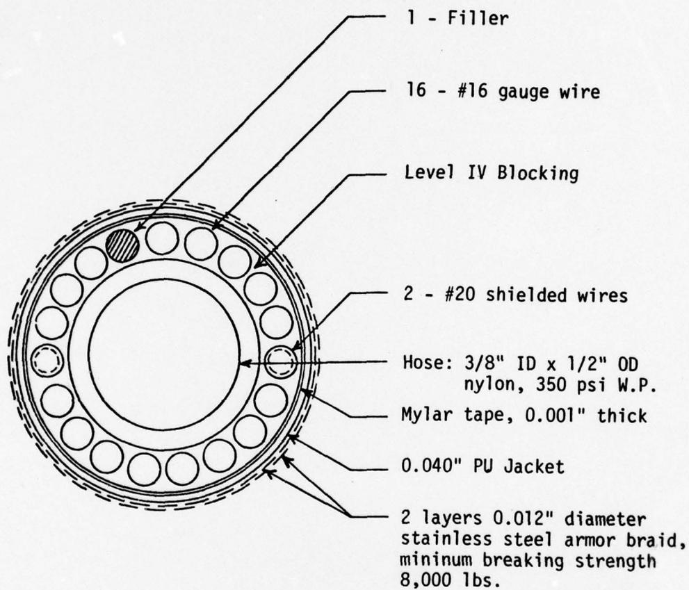
Figure 3. Schematic diagram of the towing cable,
