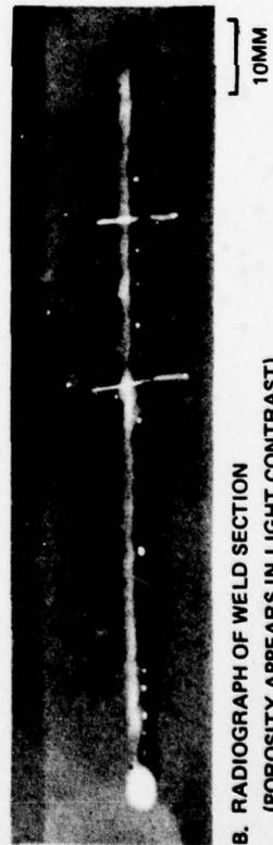
B. RADIOGRAPH OF WELD SECTION
