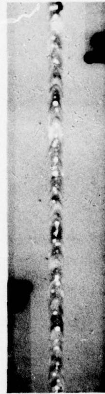
B. RADIOGRAPH OF WELD SECTION
