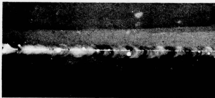
C. RADIOGRAPH OF WELD SECTION
