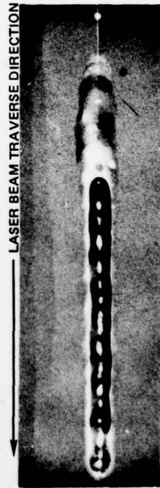
B. RADIOGRAPH OF WELD SECTION
