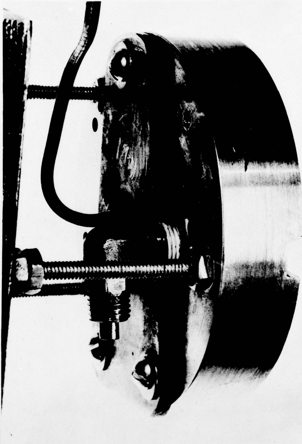
LONG SCREWS ATTACH SHIELD TO MOUNTING BRACKET
