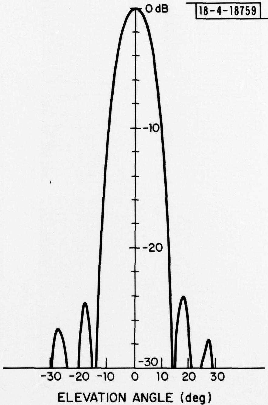
Fig. 5.4. Measured elevation pattern at 1.3 GHz.
