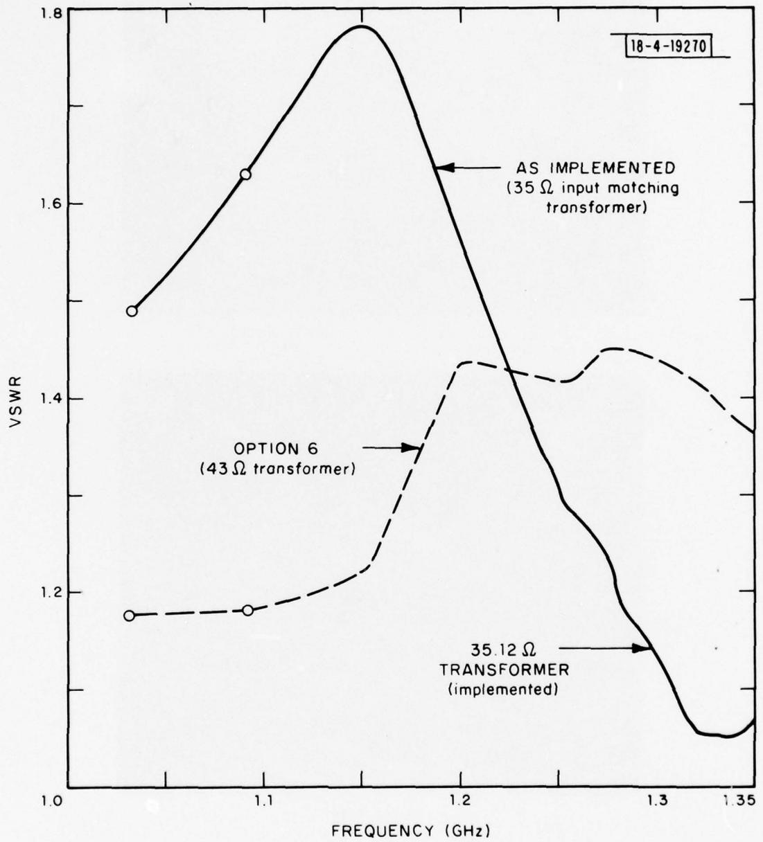
Fig. 2.6. Measured VSWR of dipole in simulator.
