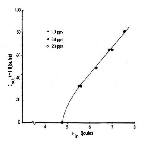
Figure 3. Input-output energy characteristics for the M=2 unstable resonator.
