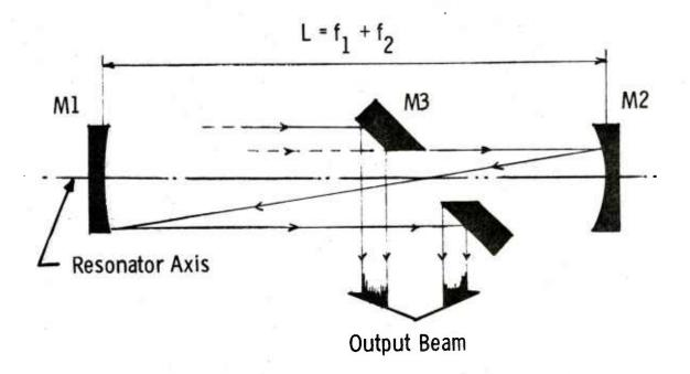
Figure 2. Negative-branch unstable resonator.
