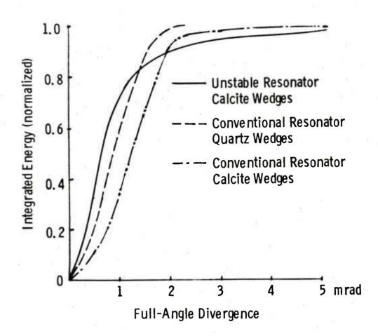
Figure 9. Divergence. Conventional resonator and M=2 unstable resonator, 1 pps, 90 mJ output.
