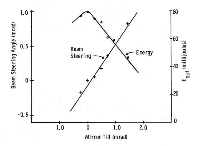
Figure 6. Energy, beam steering vs. mirror tilt M = 2 unstable resonator, 10 pps.
