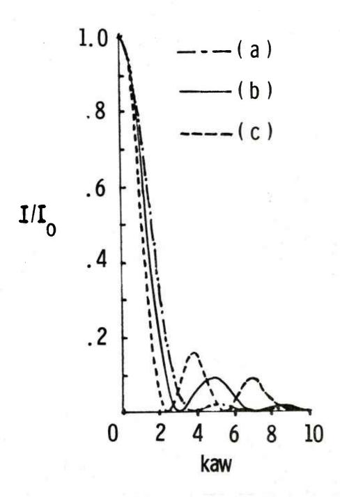
Figure 11. Normalized intensity curves for Fraunhofer patterns of (a) circular aperture, (b) annular aperture with M = 2, and (c) annular aperture with M 1. k is the laser wave vector, a is the outer radius of the aperture, and w is the angular coordinate of the far-field point (Ref. M. Born and E. Wolf, Principles of Optics, Pergamon, Oxford, 1975, p. 416).
