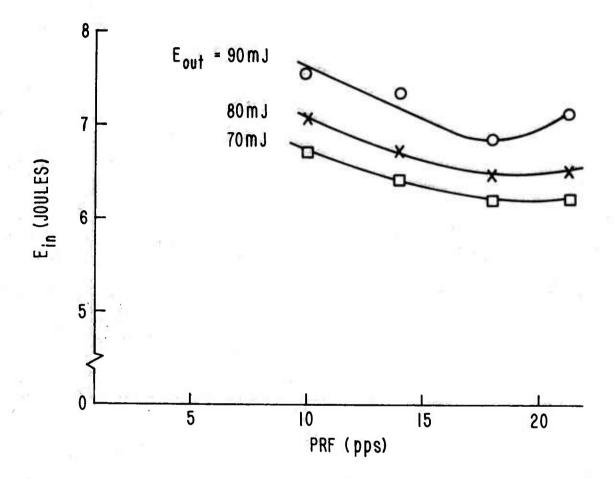
Figure 8. Ein vs. PRF. Conventional resonator with 11.4 meter negative compensating lens.
