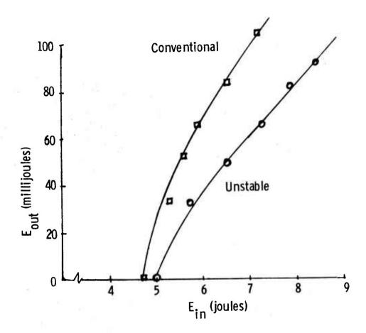
Figure 7. Input-output energy characteristics, 1 pps, of conventional and M = 2 unstable resonator.
