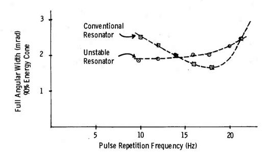
Figure 10. Divergence vs. pulse repetition frequency. Unstable resonator (M = 2), compared with conventional resonator using compensating lens to reduce thermal lensing effect.
