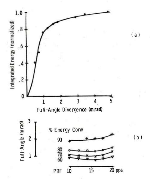
Figure 4. M = 3 unstable resonator, 90 mJ output energy per pulse. (a) Beam divergence 16 pps, (b) Divergence vs. PRF.
