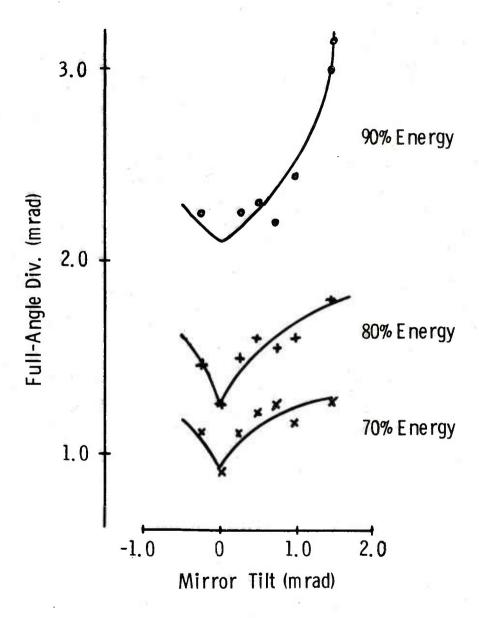
Figure 5. Divergence vs. mirror tilt for M=2 unstable resonator.
