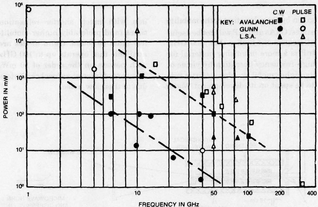
Figure 13. Output power versus frequency for some avalanche and transferred electron diodes.
