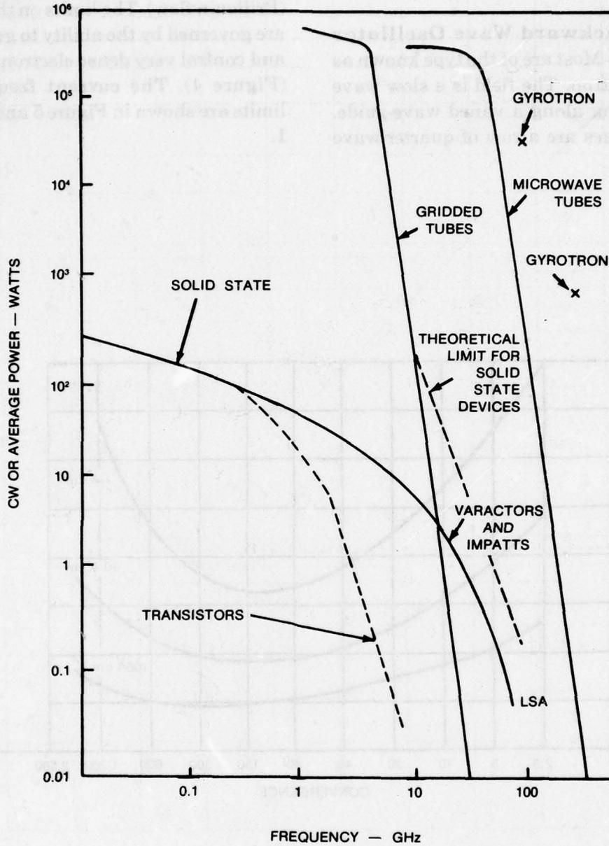
Figure 3. Power Limitations of Current Microwave Tubes and Solid State Devices
