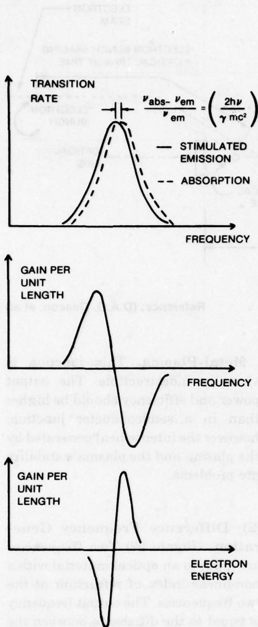
Figure 18. Relationship between line shapes for emission and absorption
