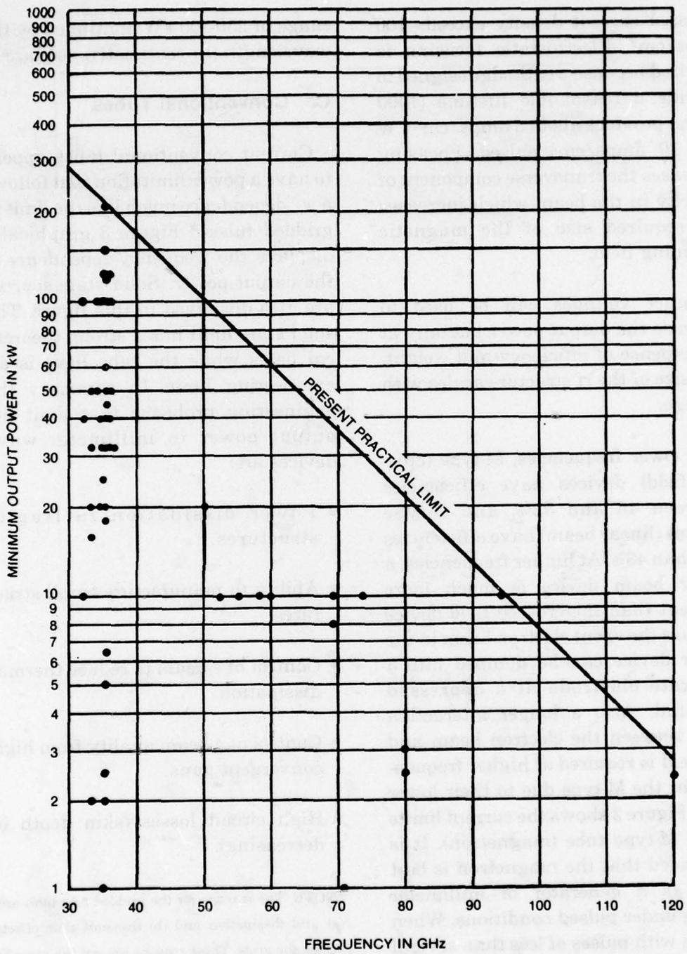
**Figure 2. Commercially Available Pulsed Millimeter Magnetrons (Reference 1)**
