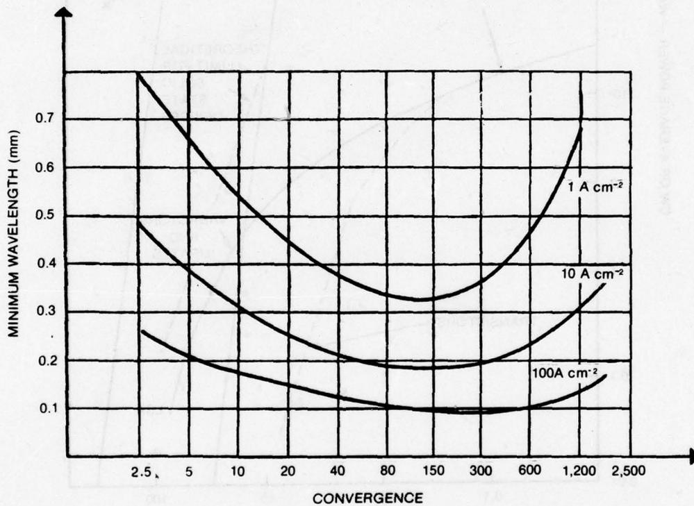
**Figure 4. The Limit in Wavelength as a Function of the Gun Convergence for Different Current Densities at the Cathode of a BWO**
