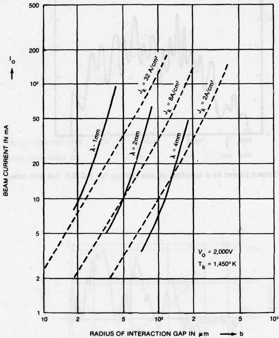
**Figure 7. Short Wavelength Limit of Reflex Klystron**
