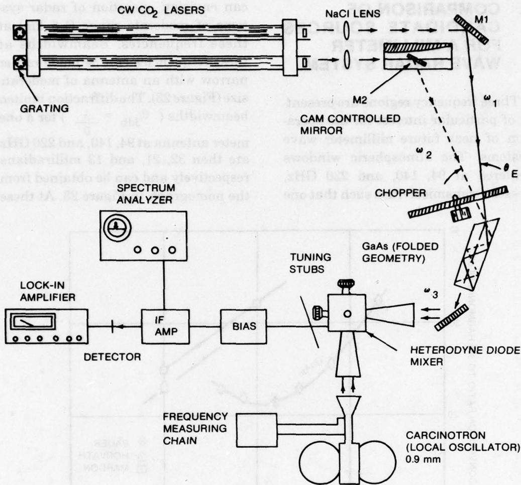
Figure 22. Noncollinear difference frequency generation (Reference 5)
