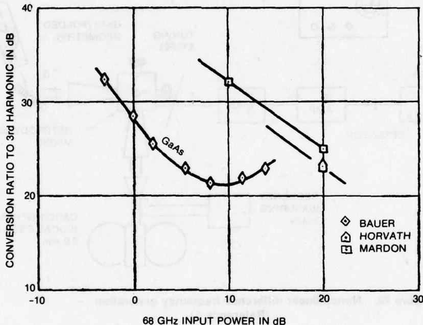
Figure 21. Third harmonic conversion efficiency of P-Si and GaAs (Reference 1)
