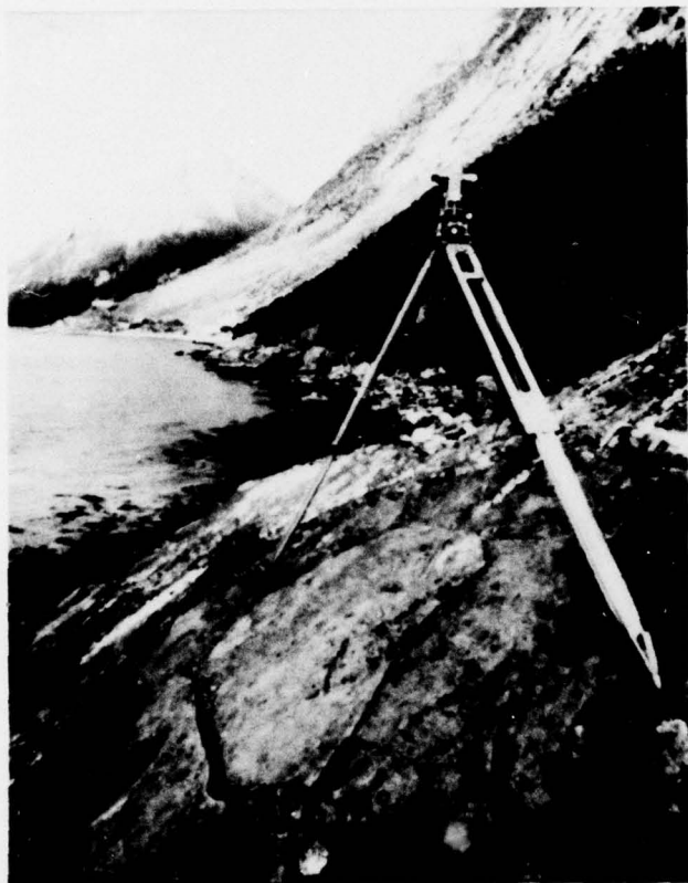
H6. Point "A" viewed from "B." It is located just above the road embankment between the house near the shore and the transmitter building. The house is the same as in picture H2. To view it through the transit requires erection of a small cairn of rocks over the "X," marked with a strip of white paper. The original point is a bench mark on top of the transmitter building; this is the circled "X" in figure H1.
