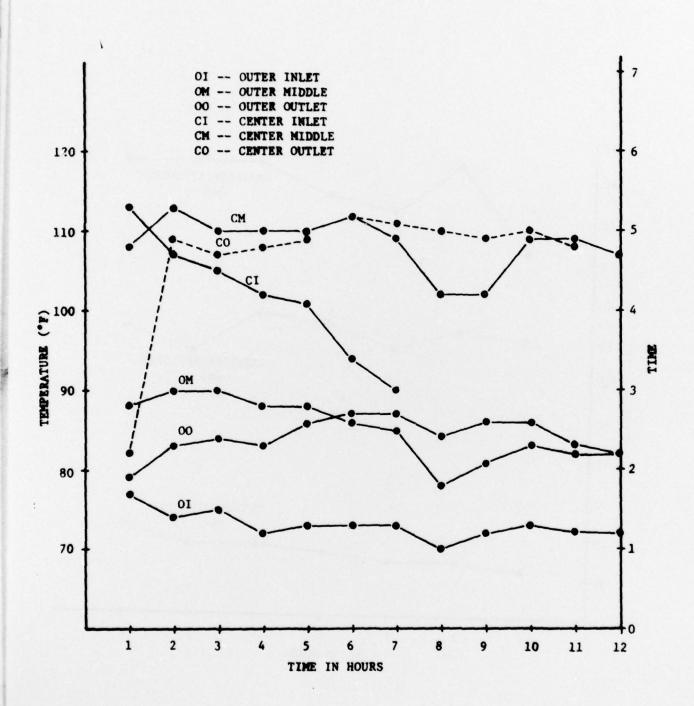
FIGURE 3. ABSORBENT BED TEMPERATURES VERSUS TIME FOR MK 11 MOD O UBA - MEAN OF ALL TESTS. WATER TEMPERATURE 29-34° F
