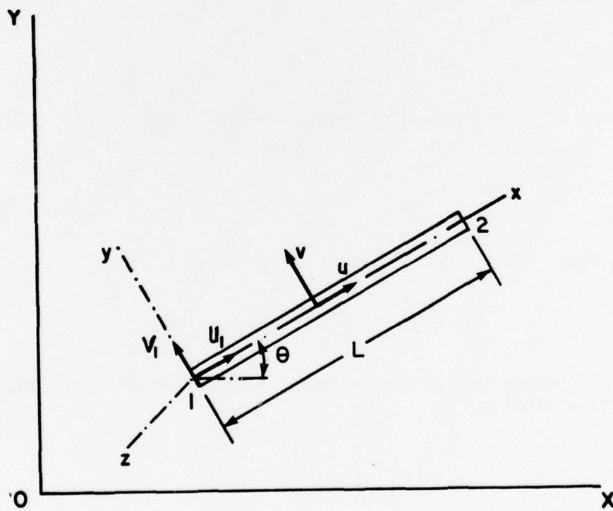
Figure 1. A beam-column finite element.
