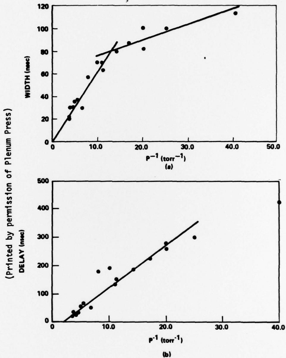
Figure 4. FIR Width and Delay vs Inverse Pressure  $P^{-1}$ .
