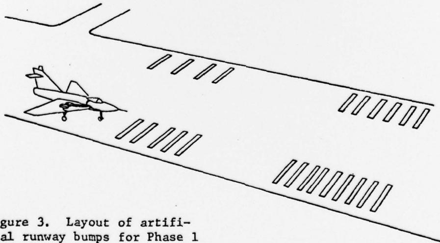
Figure 3. Layout of artificial runway bumps for Phase 1 taxi tests.
