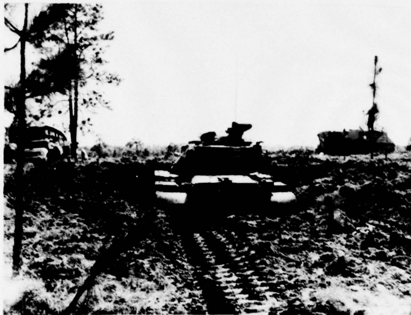
Figure 5. Rear view of an M60 tank in an explosively excavated defensive position
