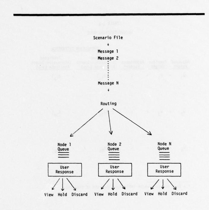
FIGURE 2-5 MESSAGE HANDLING BEHAVIORS IN INTERIM TEST FACILITY
