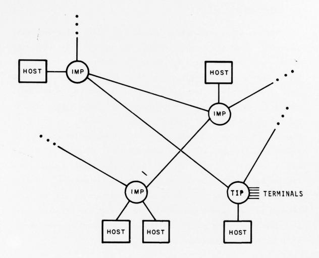
Figure 1-1 A Typical Section of the ARPANET
