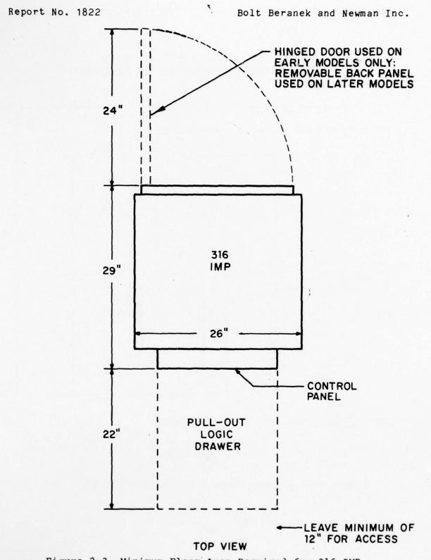
Figure 2-3 Minimum Floor Area Required for 316 IMP
