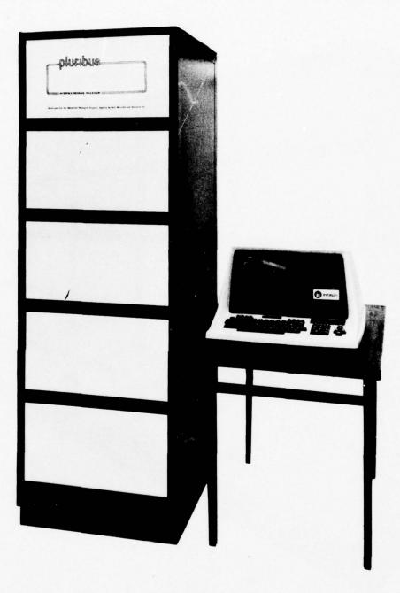
Figure 1-5 The Pluribus IMP and IMP Terminal
