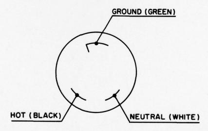
Figure G-2 Twistlock Receptacle (Viewed from Socket Side)
