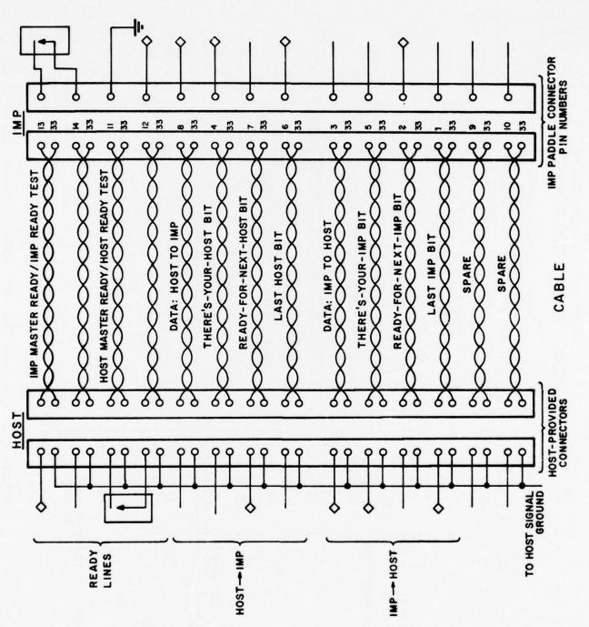
Figure 4-5 316 Host Cable Signals (Local Host)
