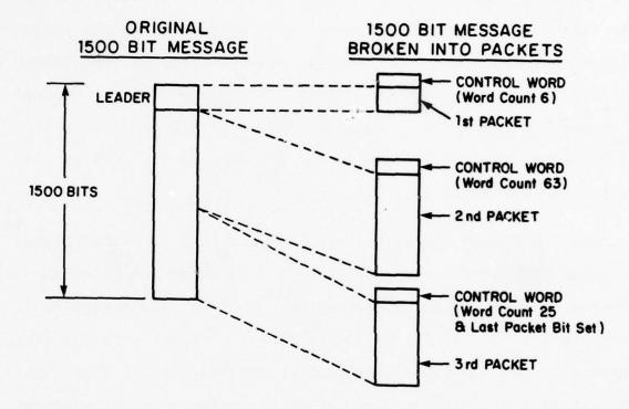
Figure F-5 Segmentation of a Message into Packets for the Very Distant Host Interface
