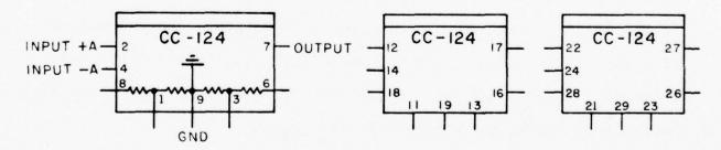
Figure D-1 Differential Receiver PAC Model CC-124, Schematic Diagram and Logic Symbol. (Shown as connected in IMP)
