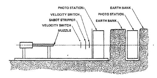
Figure 4 Experimental setup Series 1.
