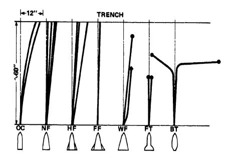
Figure 16 Trajectory stability, Series 1 and 2. (Deviations are schematic and approximate.)
