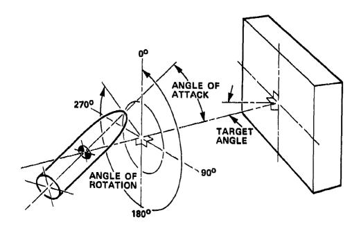
Figure 15 Projectile-target frame of reference and angle definition.
