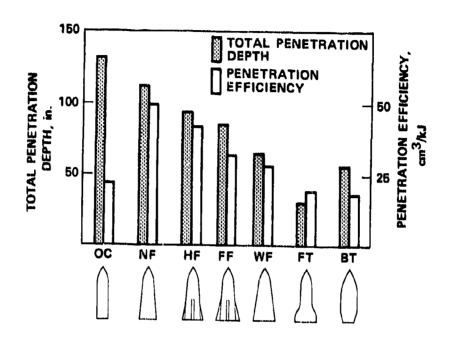
Figure 17 Total penetration depth and penetration efficiency for seven projectile shapes, Series 1 and 2.
