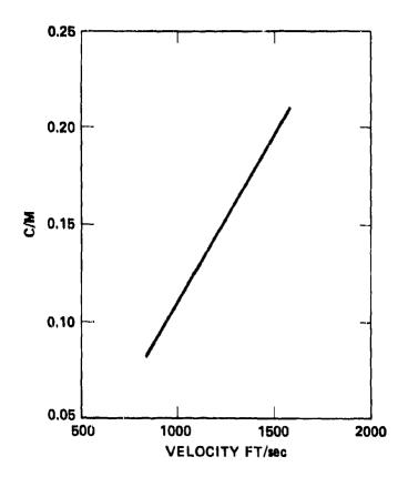
Figure 7 Projectile velocity versus c/m (charge mass/projectile mass).
