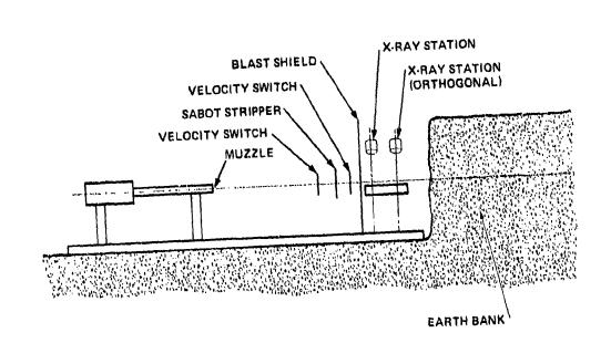
Figure 12 Experimental setup series 3.
