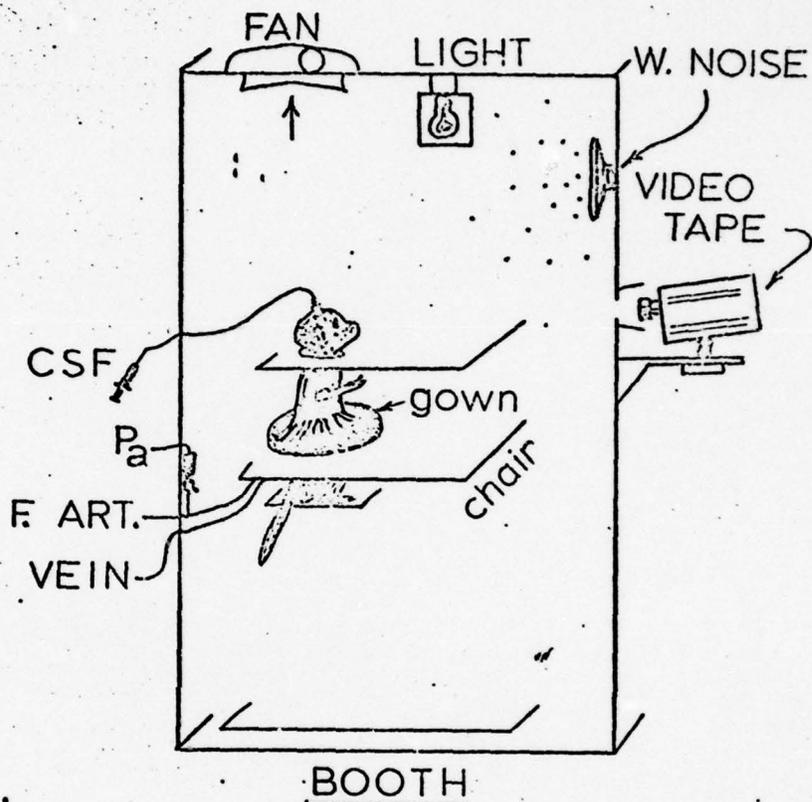
**FIGURE 1.** Experimental booth which houses the chair and primate during drug studies. The light is attached to a timer, and the monkey may remain in the booth for 24 hr at a time. A small transparent window is provided for the video tape camera. The arterial pressure gauge ( $P_a$ ) is mounted on the booth in a fixed position with respect to the monkey. The chair is set on rails which permit removal from the booth horizontally for minor adjustments, etc.
