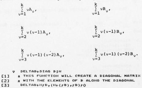
The function DIAG creates the matrix  $\Lambda(\beta)$  which is a diagonal matrix with the elements of the vector  $\underline{\beta}$  along the diagonal.
