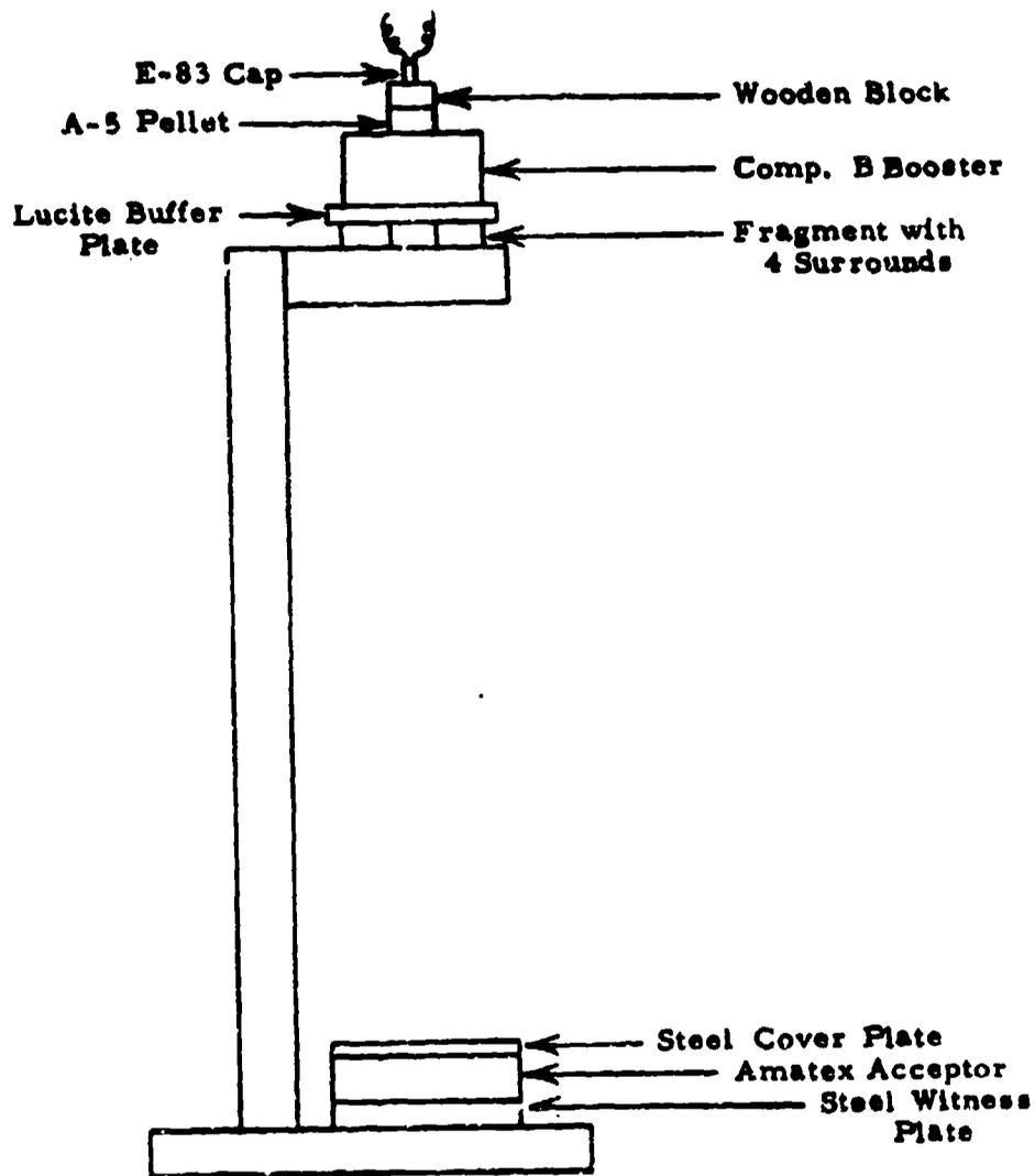
Fig 2 Schematic of experimental set-up
