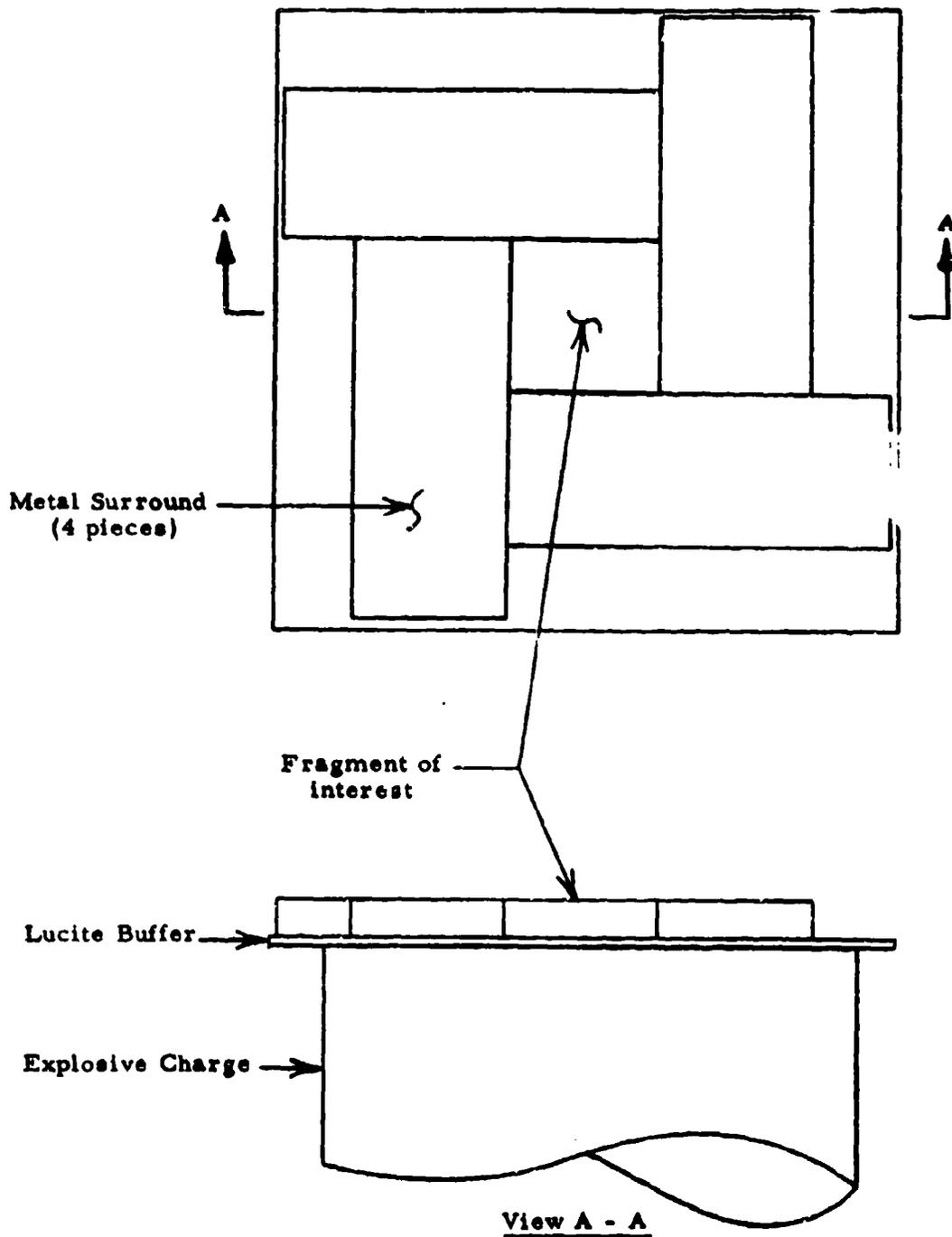
Fig 4 Schematic of fragment propulsion system
