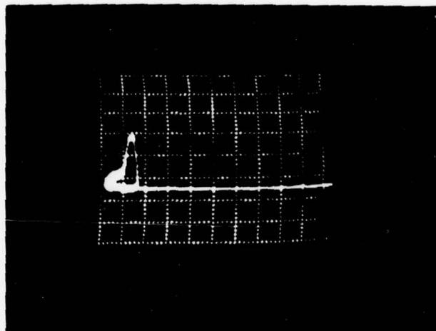
Fig. 4 Response of the 7B70 Sweep Circuit
