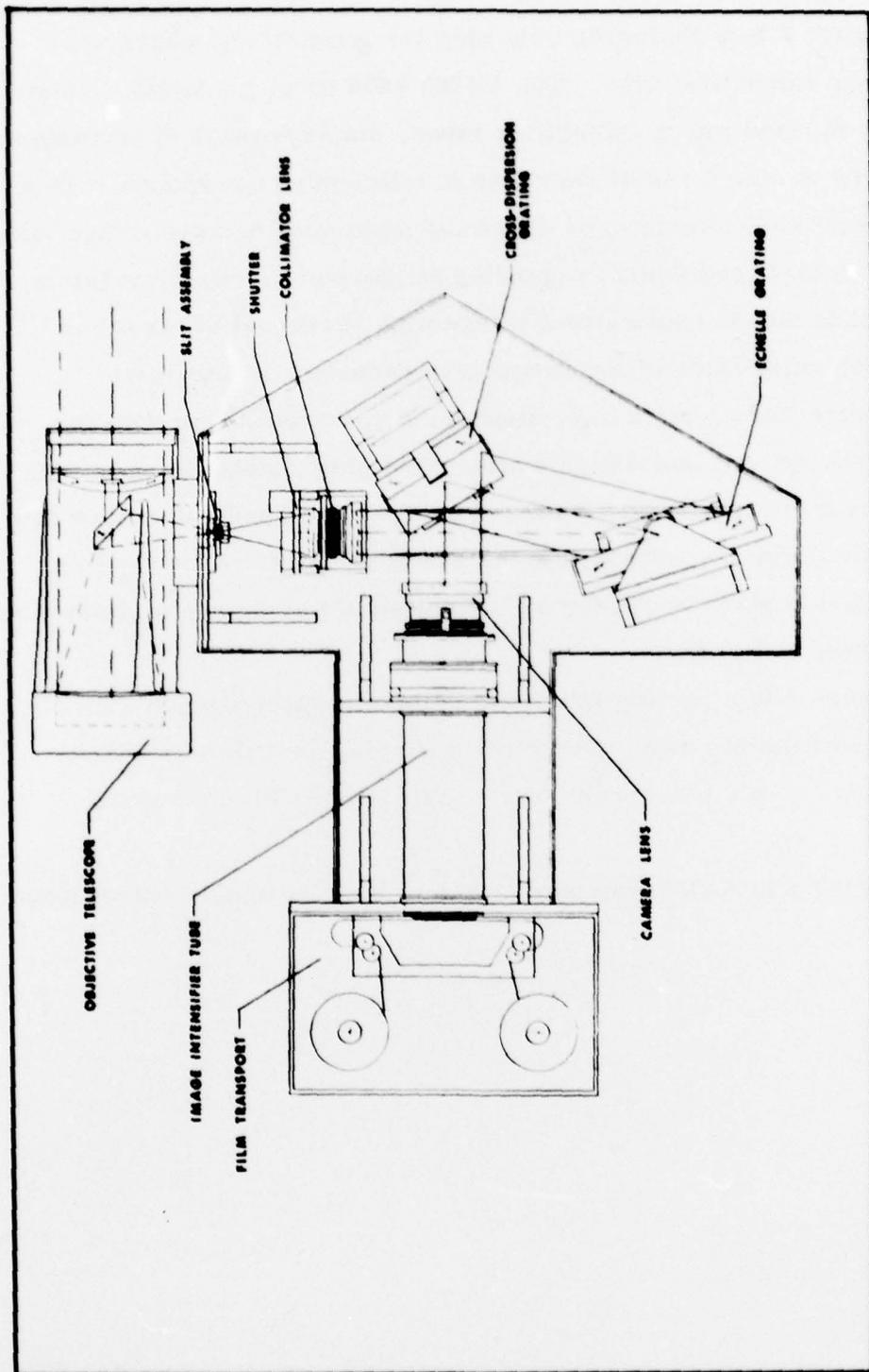
Figure 1. Optical Diagram of Spectrograph.
