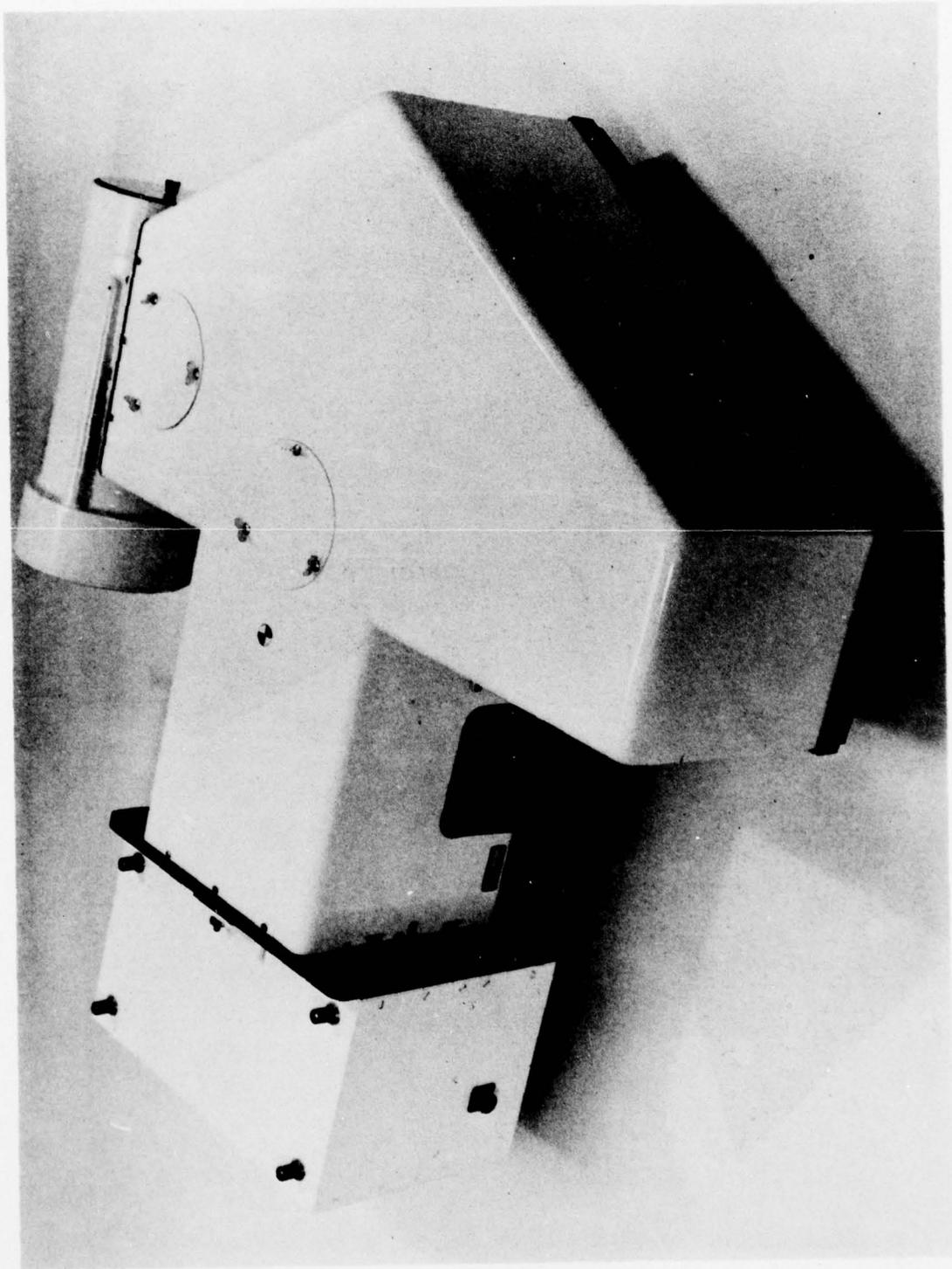
Figure 4. Completed Super Cygnus Spectrograph.
