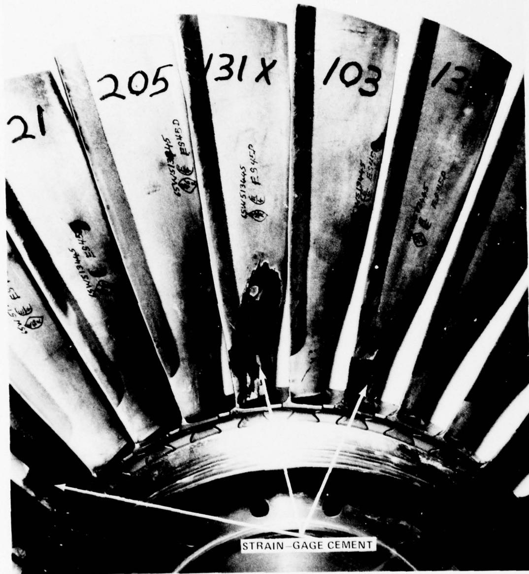
Figure 12-6 TF30P-9 BORSIC<sup>®</sup>/Aluminum Fan Blades After 184-Hr. F111-D Flight Program (Front View)
