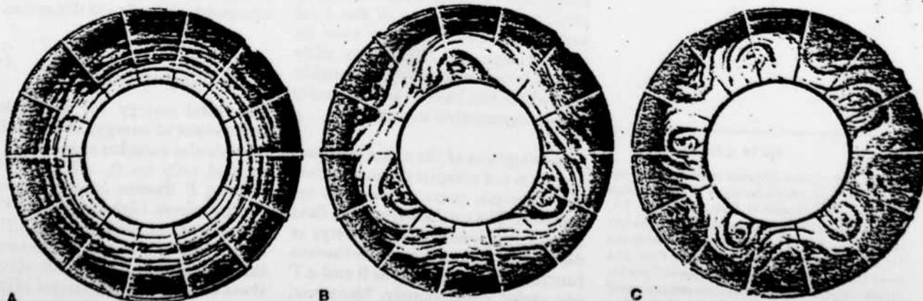
Figure 1. Streak photographs illustrate three typical flow patterns in a differentially heated rotating annulus of fluid: (A) symmetric,  $\Omega = 1.88$  radians per sec; (B) three-wave,  $\Omega = 2.19$  radians per sec; (C) five-wave,  $\Omega = 2.57$  radians per sec. All experiments were conducted with
