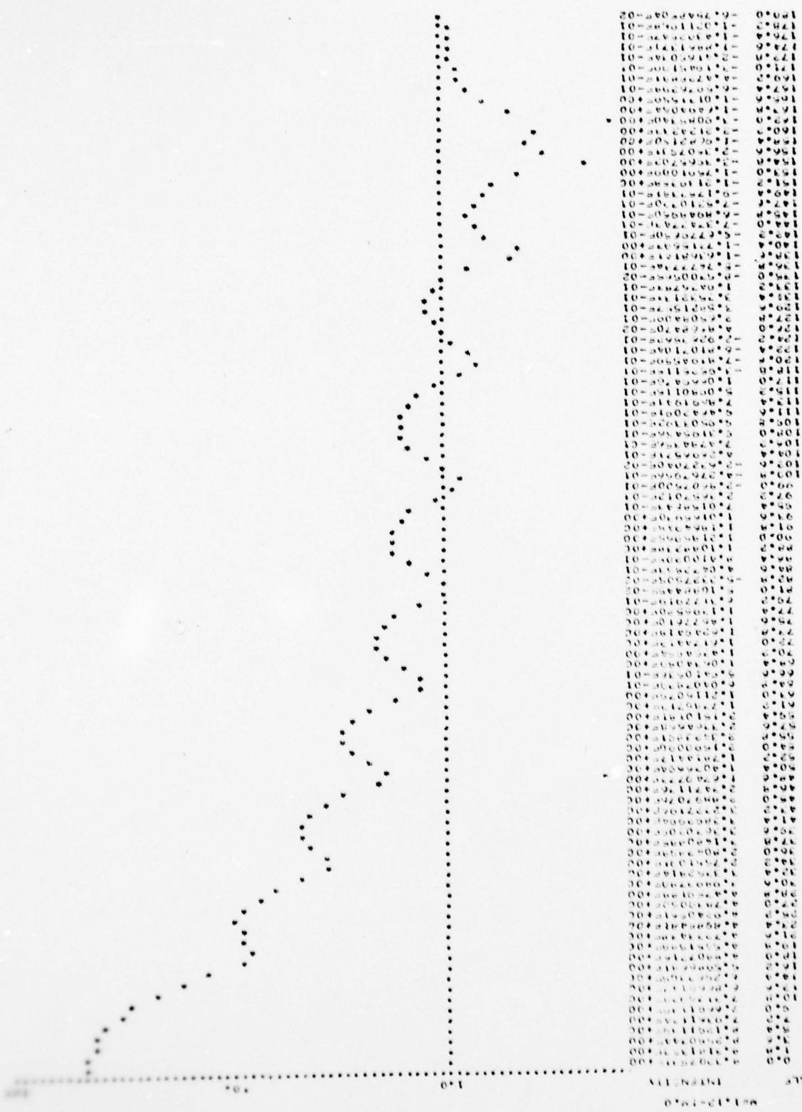
Fig. 32. Theoretical Mie results for channel 1,  $x=12.1$ ,  $R=1.12$ .
