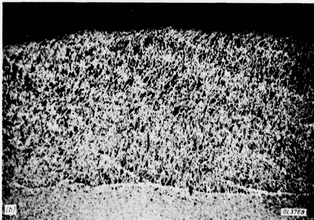
Fig. 11. Low frequency pulsing, no modulation. Pulse 0.5sec, background 0.5sec: a) Transverse x 10, b) longitudinal x 16.
