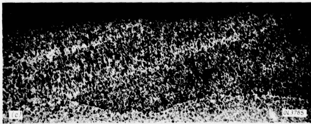
Fig.13. Effect of current modulation superimposed onto 1sec pulse, 0.5sec background: a) 50Hz; b) 20Hz; c) 10Hz. x16
