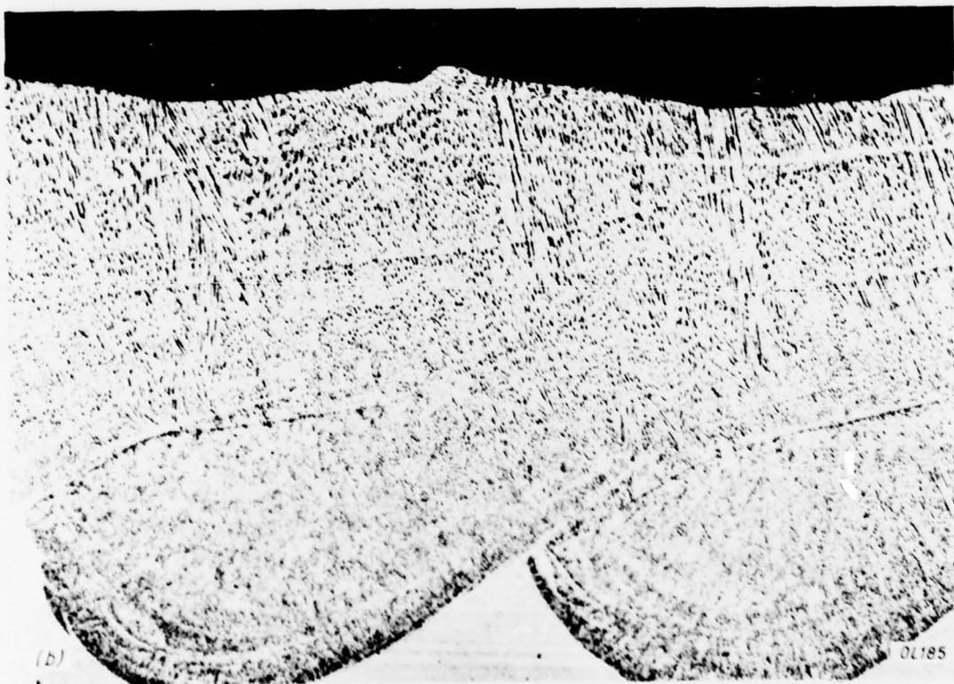
Fig. 6. As Fig. 5a etched in dendrite etch x 25. a) Transverse section. b) longitudinal section
