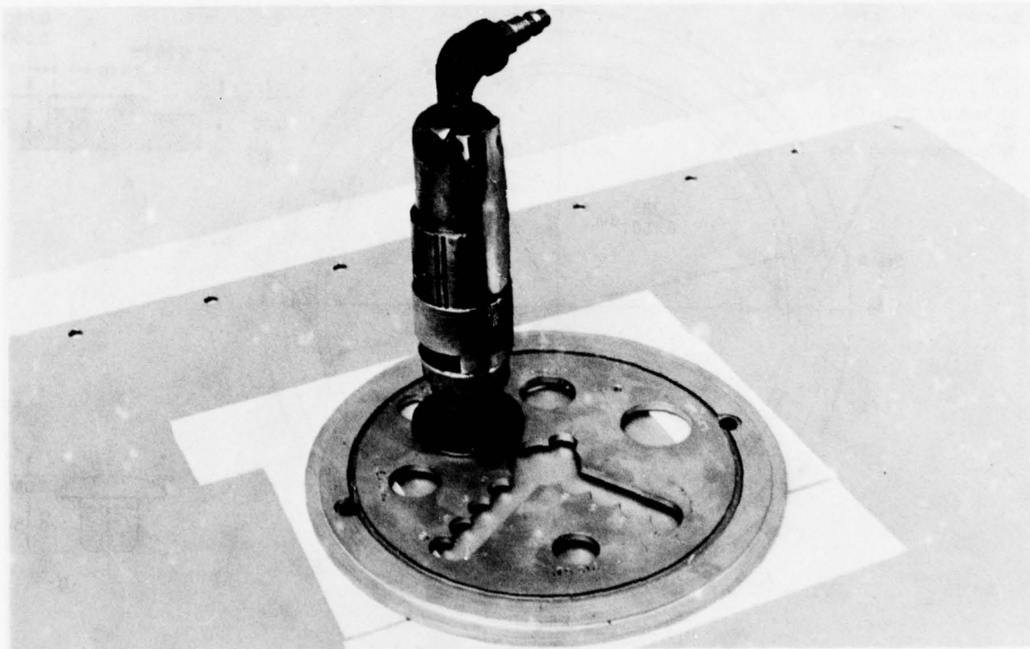
Figure 8-4.—Air-Powered Router and Variable Diameter Router Template
