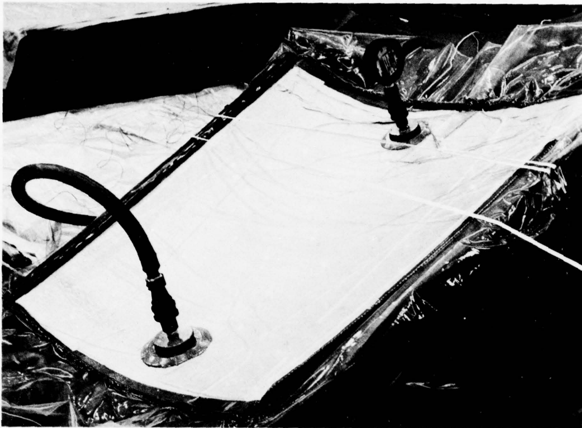
Figure 7-30.—Checking the Vacuum Assembly for Leaks
