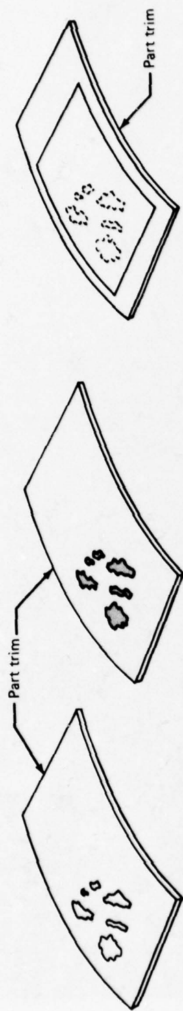
c. Model Part With 0.012 in. Aluminum Sheet Covering Filled Area
