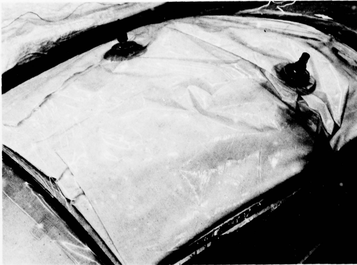
Figure 7-29.—Vacuum Probes Positioned on Bleeder Cloth at Edge of Assembly
