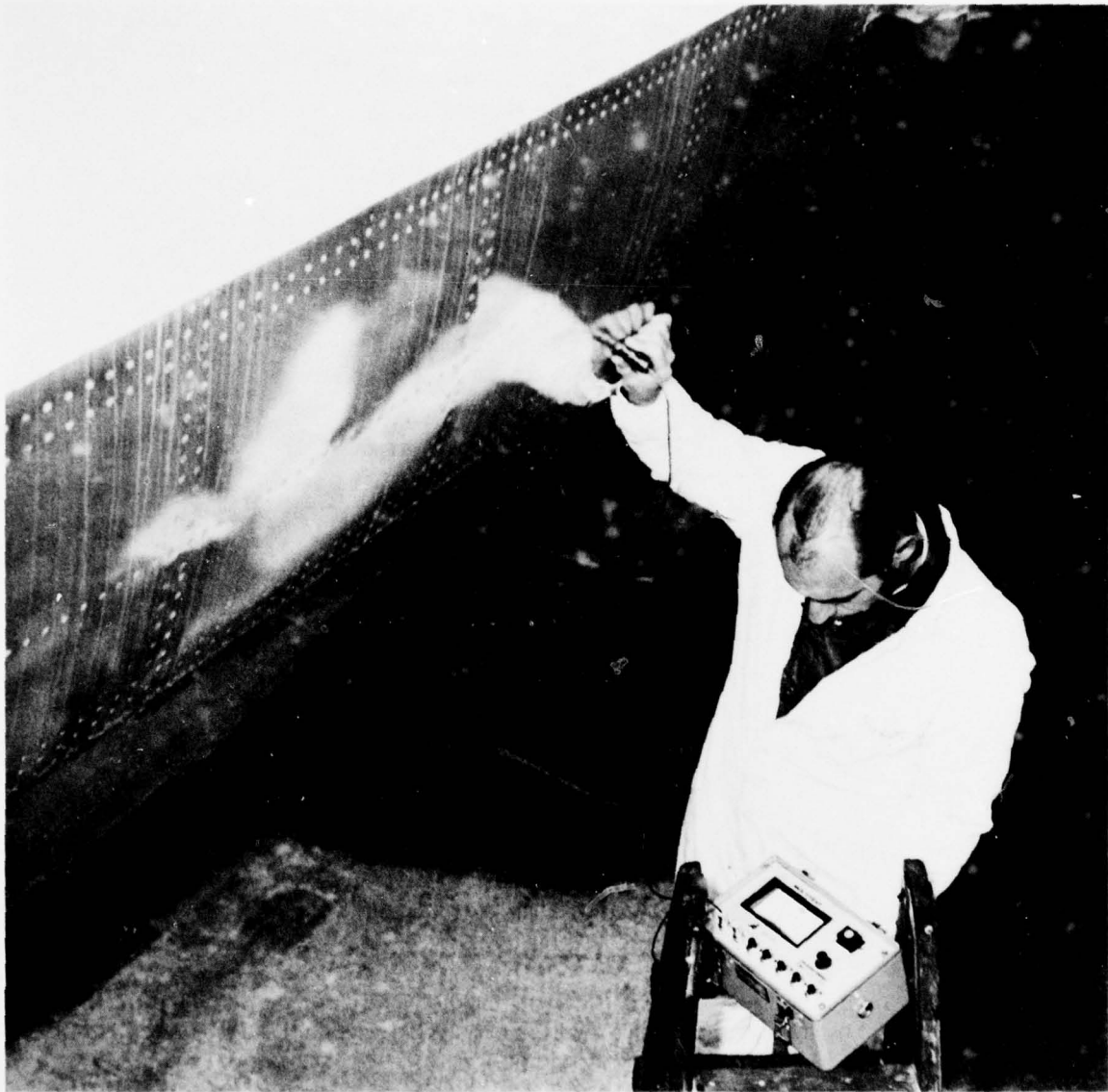
Figure 10-35. – Eddy Current Inspection of Fuselage Skins for Faying Surface Corrosion
