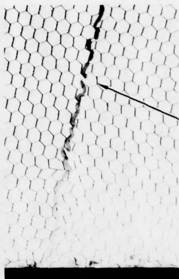
Figure 10-26.—Radiograph of Failure of Foam Adhesive to Expand into Adjacent Cells
