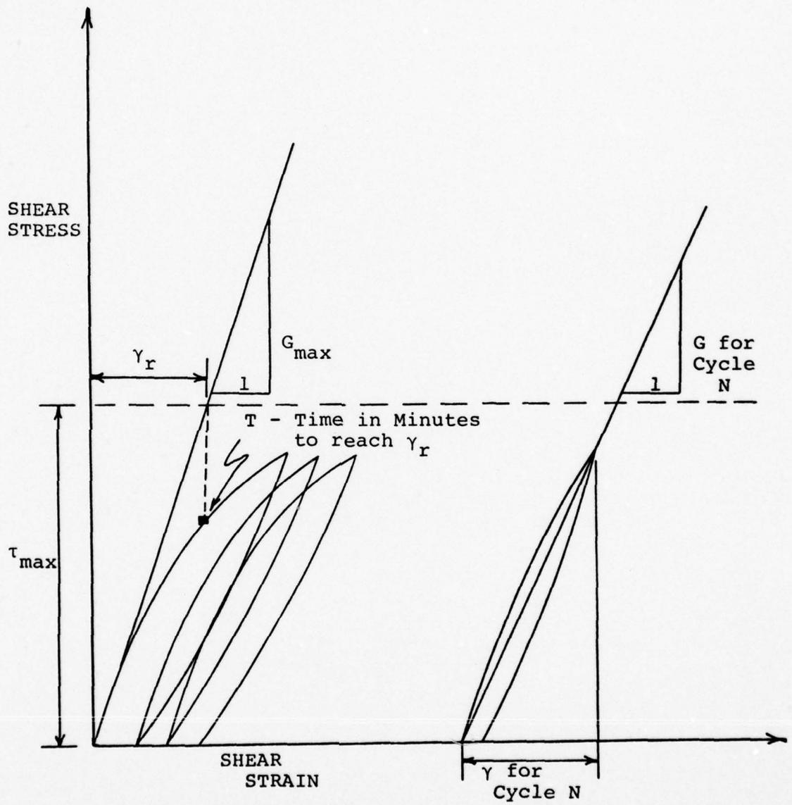
FIGURE 2 SCHEMATIC OF SHEAR STRESS-SHEAR STRAIN RELATION
