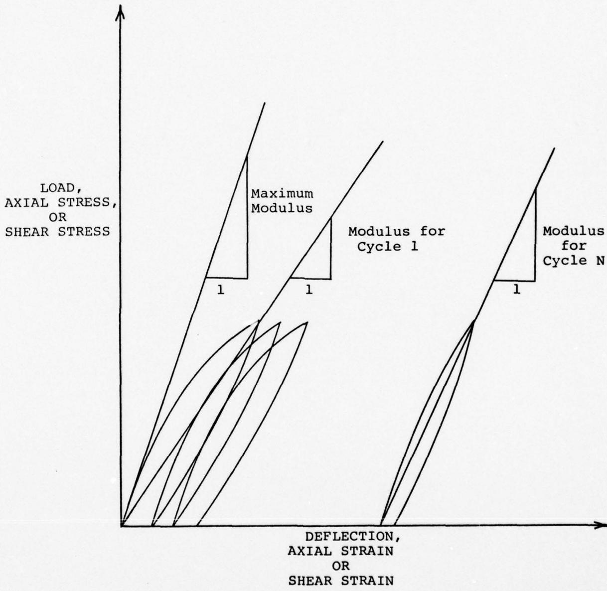
FIGURE 1 SCHEMATIC OF LOAD-DEFLECTION, AXIAL STRESS-
