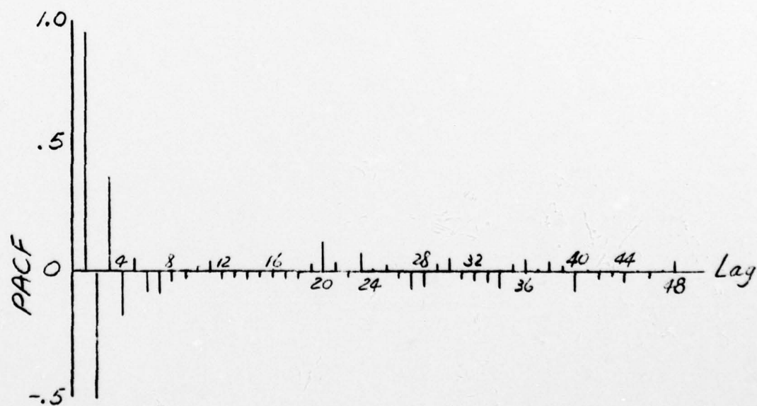
Fig. 8 Partial Autocorrelation Function of Response to White Noise
